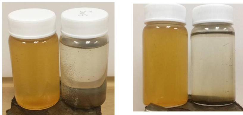
Figure 4.11 a) Water treatment using 5mg/mL maghemite concentration, 30 seconds separation time. b) Water treatment using 2.5 mg/mL, 3 hours separation time
