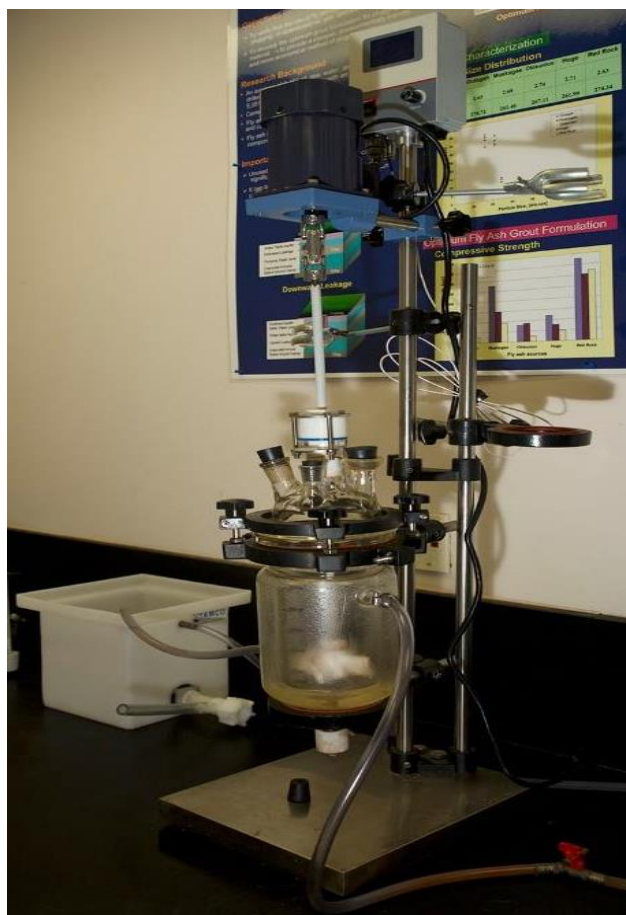
Figure 3.1 Reactor setup for MNPs synthesis
