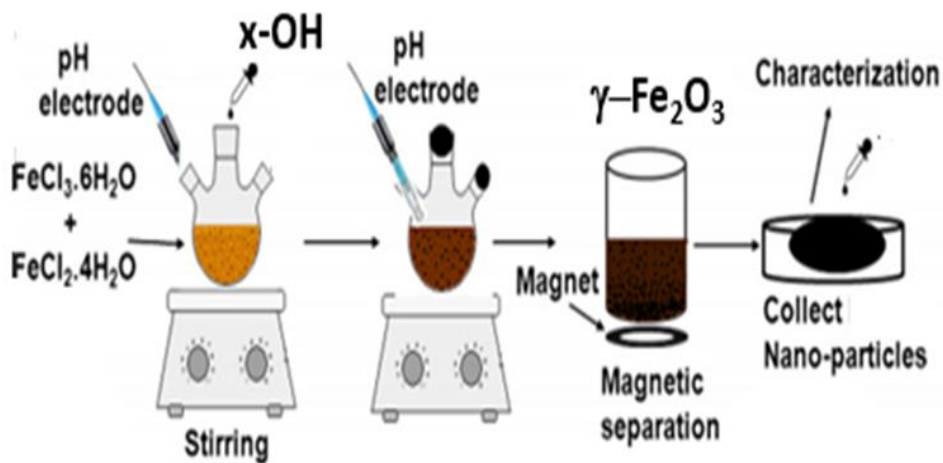
Figure 3.2 Chemical co-precipitation method schematic
