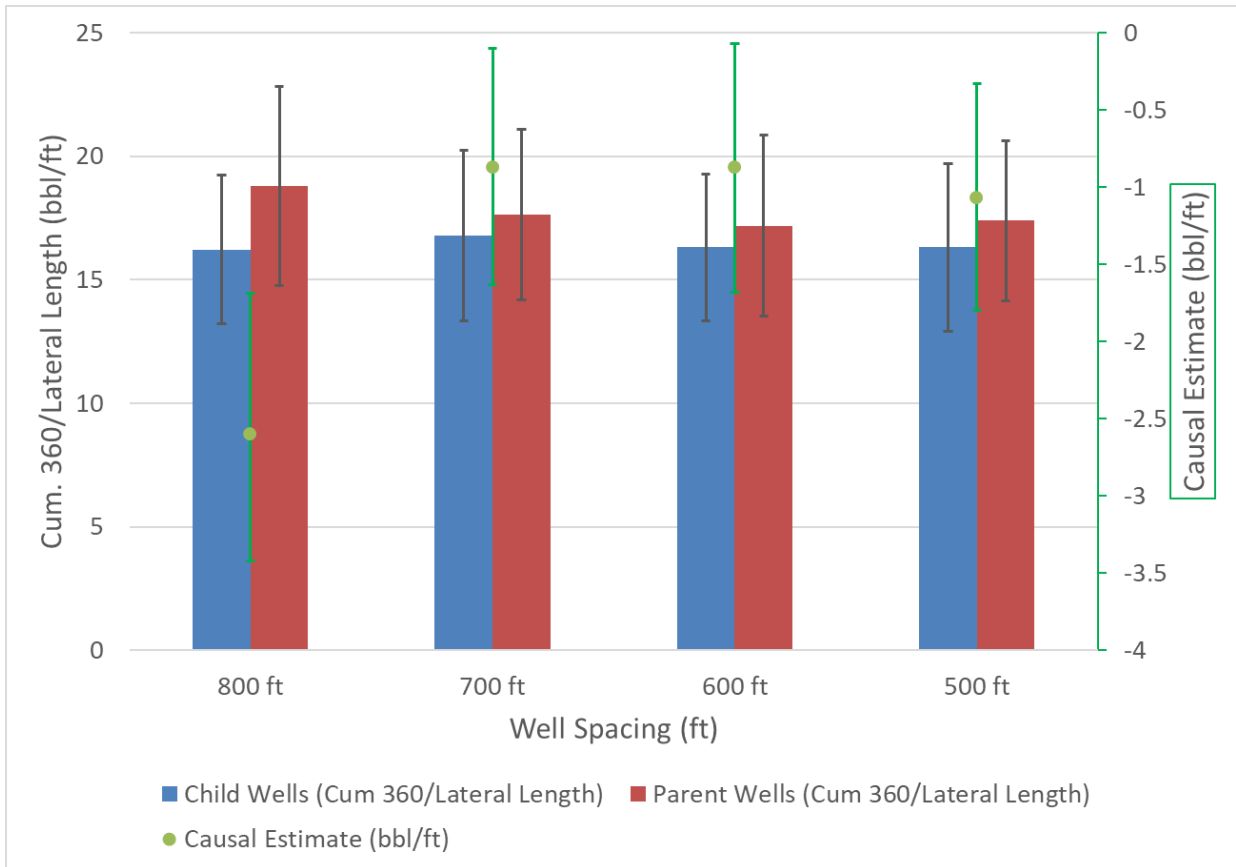
Fig. 2. 28— Bar chart comparing potential outcomes for 360-day cumulative production normalized to lateral length (bbl/ft) of parent-child well groups and causal estimates for each well spacing option using causal inference (Sakhardande and Devegowda 2021).
