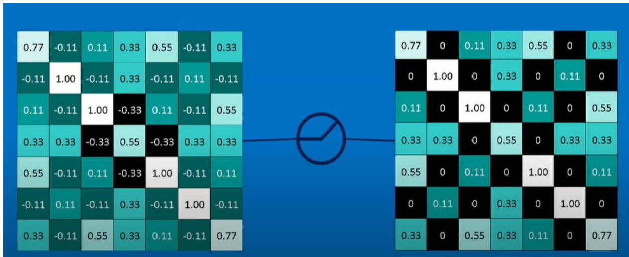
Fig.3.14—Example of ReLU function indicated by the circled operator applied on an activation map
