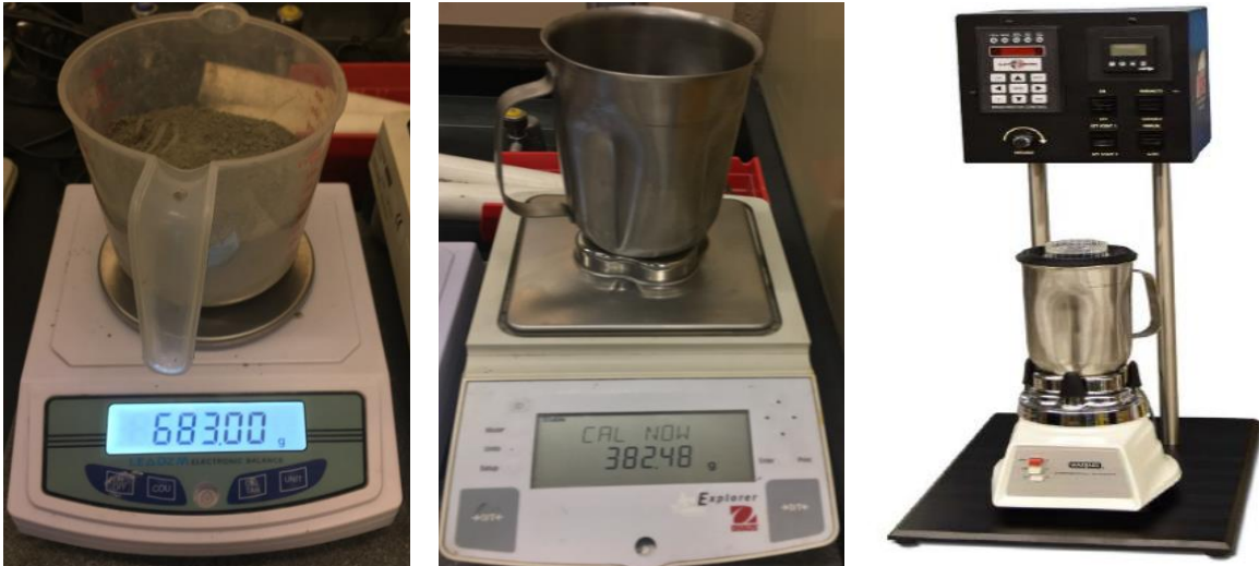
Figure 24: Digital Weighing scales and OFITE Model 20 Constant Speed Blender (OFITE Manual)
