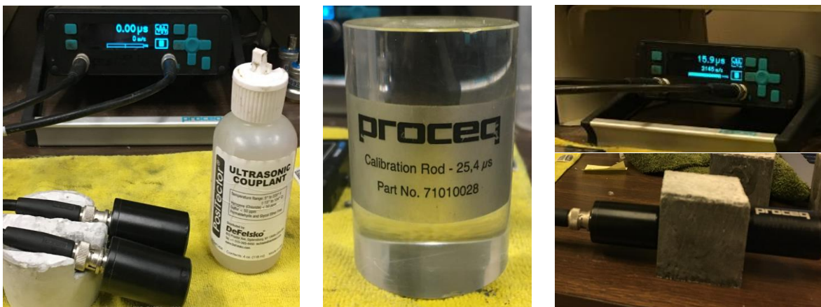
Figure 27: Proceq™ Ultrasonic device, PosiTector™ Ultrasonic couplant, Calibration Rod
