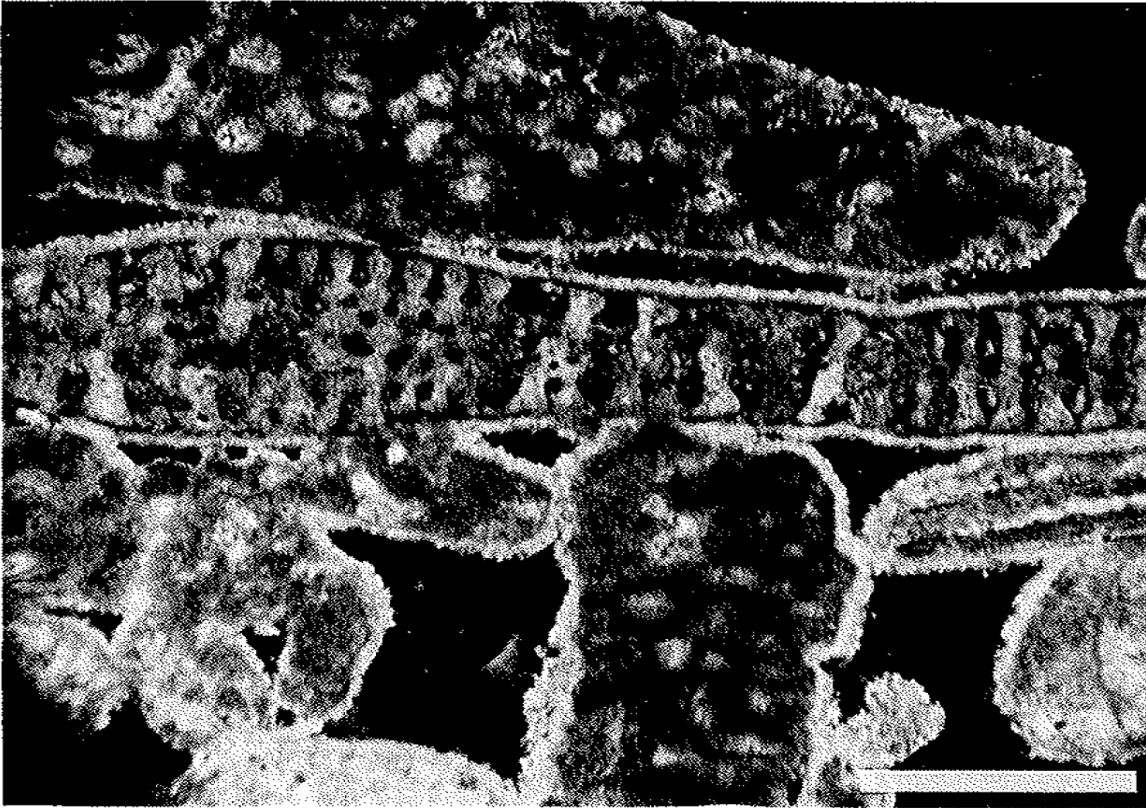
Figure 50: Cross polarized photomicrograph of Holocene high Mg Calcite isopachous allochem dasyclad cemented beachrock from Jamaica (from Pigott and Trumbly, 1985). SEM analysis reveals these allochems to be high Mg-calcite. Horizontal bar is 0.2mm. Compare this microphotograph to Figure 26.
