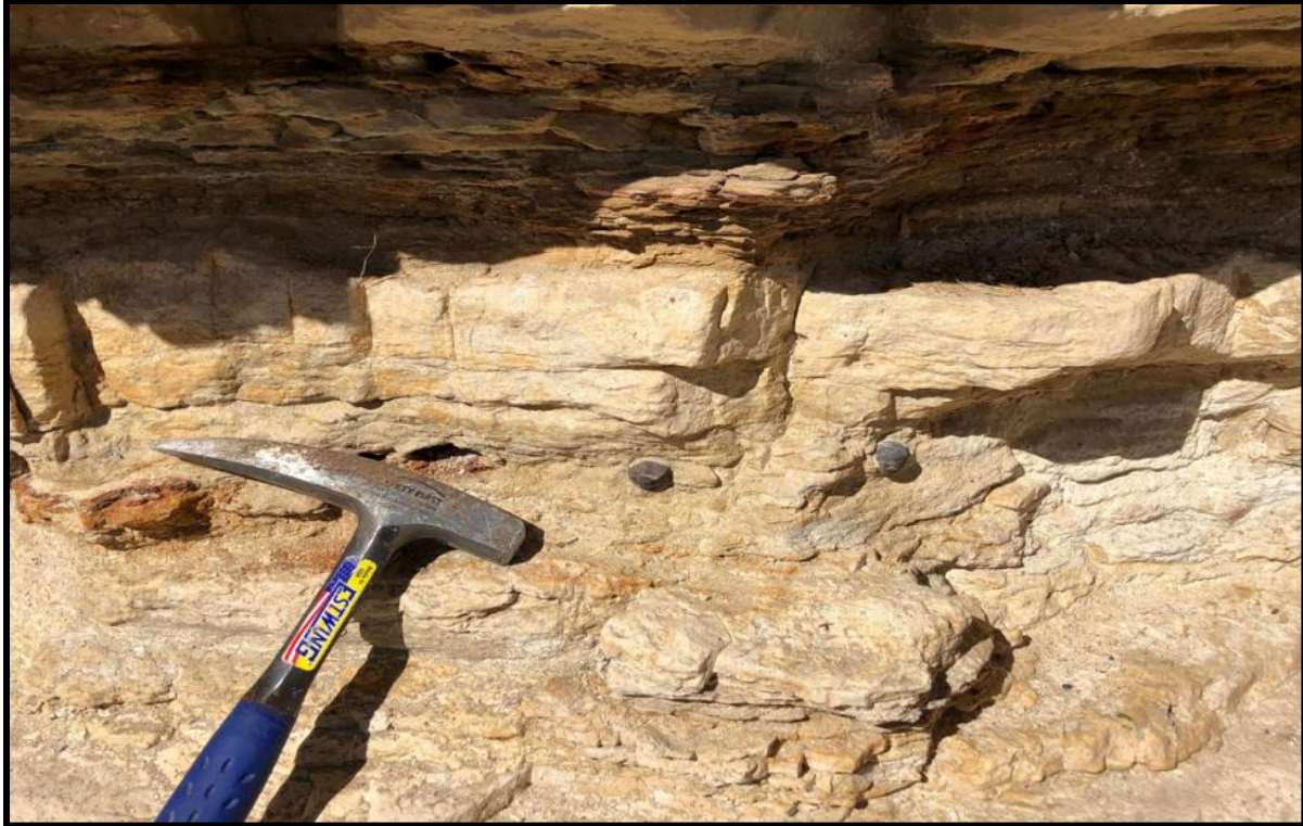
Figure 15: Siderite nodules found interbedded between the limestone and shales. Nodules are rounded, pebble like in shape and oriented parallel to bedding along section. Siderite nodules are only observed within the Unit Two. Rock hammer used for scale.
