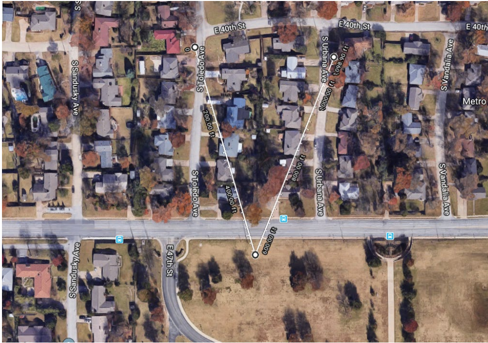
Figure 74. Antennas setup “300 feet of detection”
