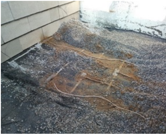
Figure 11. (Left) Exhumed instrumented reinforcement layer during deconstruction of Abutment Model #1; (Right) Survey of maximum settlements along each reinforcement layer during deconstruction
