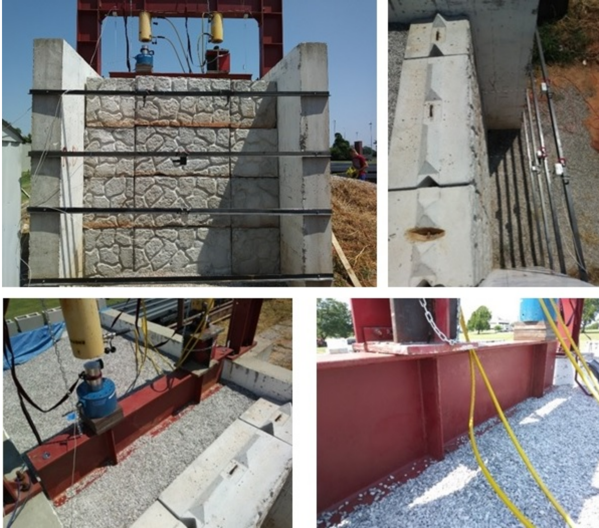
Figure 9. GRS Abutment Model #2 after surcharge loading test
