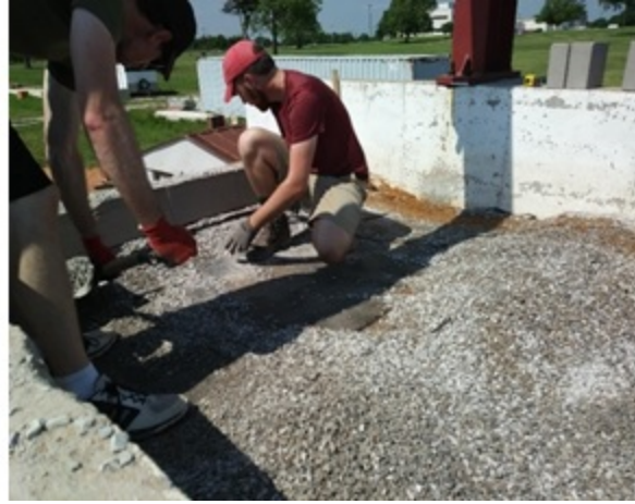
Figure 10. GRS Abutment Model #1 after load testing and removal of loading assembly: (Left) Scarp under the loading beam; (Right) Excavated fill above the top geotextile layer
