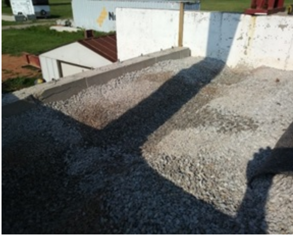
Figure 10. GRS Abutment Model #1 after load testing and removal of loading assembly: (Left) Scarp under the loading beam; (Right) Excavated fill above the top geotextile layer
