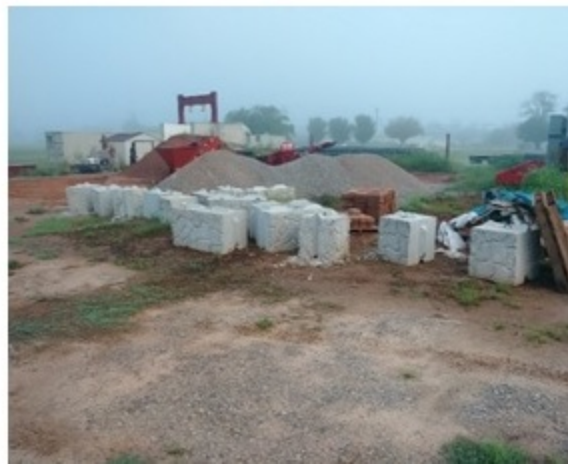
Figure 12. (Top) Removal of large concrete facing blocks at the end of test; (Bottom left and right) Test box and nearby material storage area after testing and clearing out GRS Abutment Model #2
