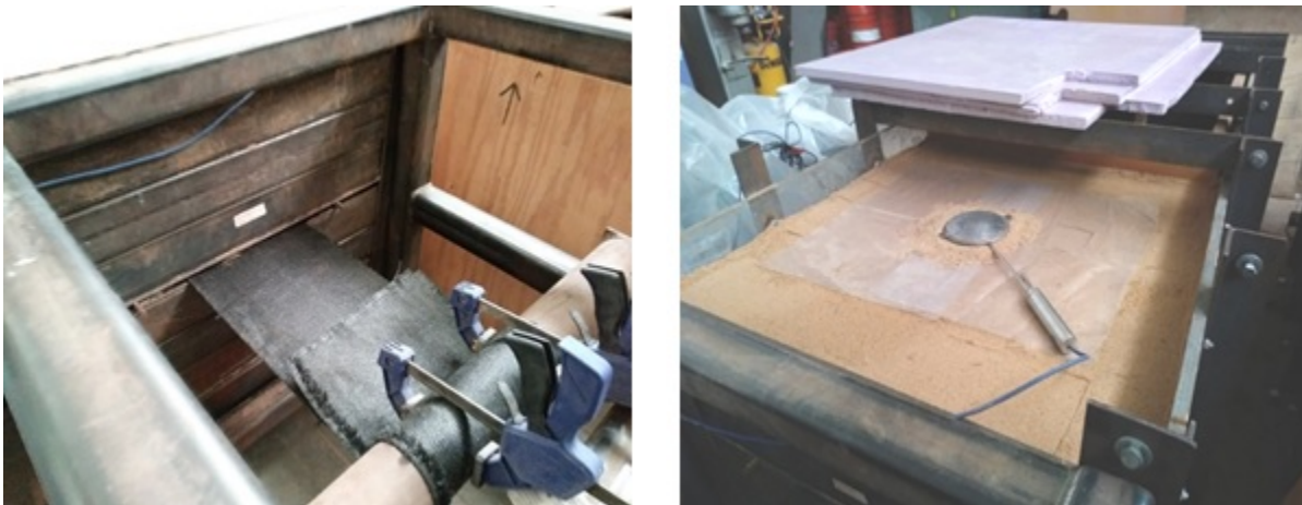
Figure 6. (Left) Geotextile specimen attached to the roller clamp of the pullout test actuator; (Right) EPC placed on the top of the sand before applying an airbag surcharge
