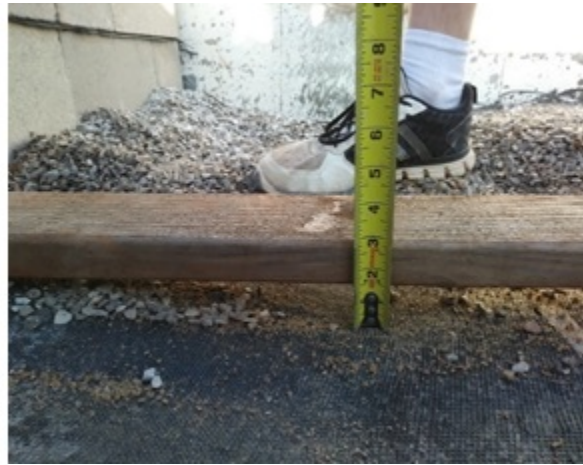
Figure 11. (Left) Exhumed instrumented reinforcement layer during deconstruction of Abutment Model #1; (Right) Survey of maximum settlements along each reinforcement layer during deconstruction
