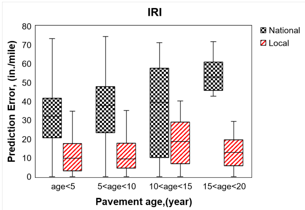
Figure 53 - Error of estimate of the IRI model vs. pavement age
