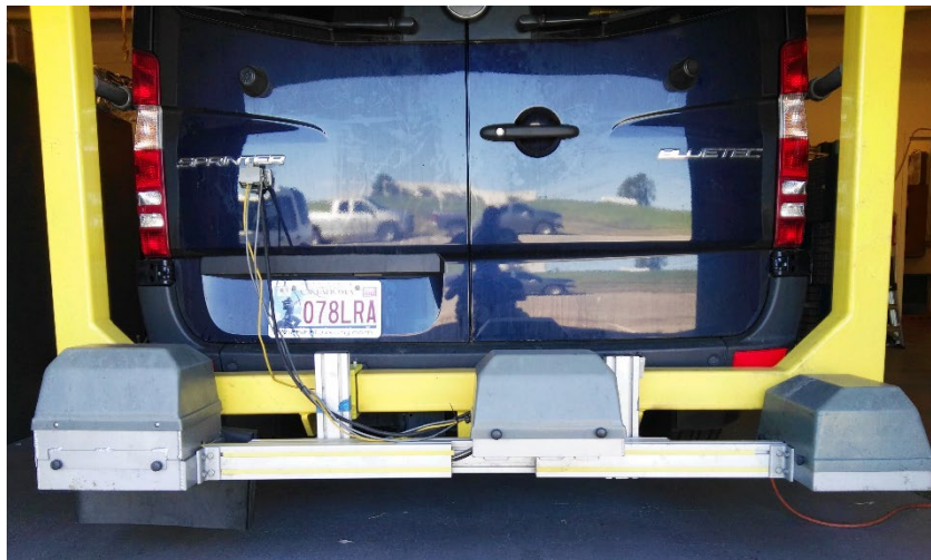
Figure 2.4 AMES 8300 Survey Pro Profiler
