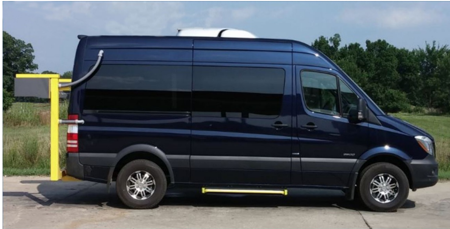
Figure 2.3 DHDV with PaveVision3D System
