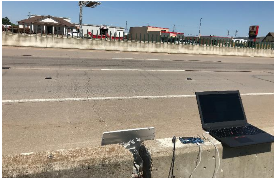
Figure 41. Laptop used to configure and communicate with two sensors in lane, through a directional antenna connected to an access point on the road side.
