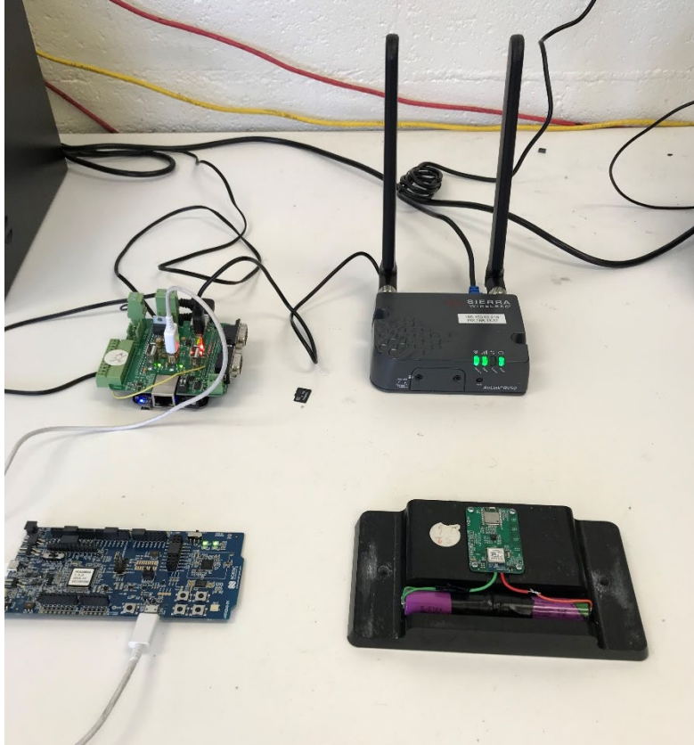
Figure 36 Remote access setup. REECE is connected to RV50 and iVCCS AP. Sensors are connected to AP over BLE.
