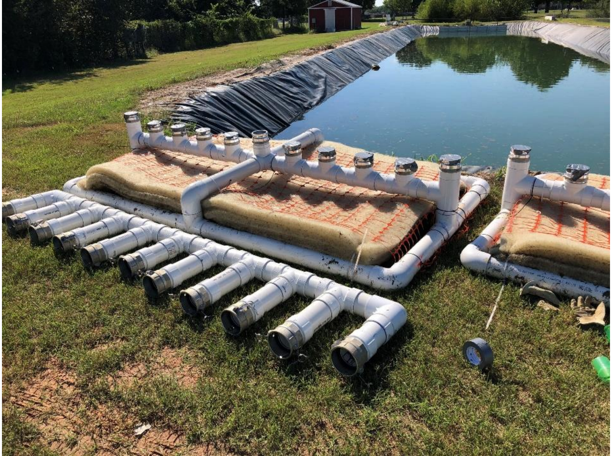
Figure 5: FWB frame used for prototype system (upside-down). Photo by Maxwell O'Brien (Oklahoma Water Survey)
