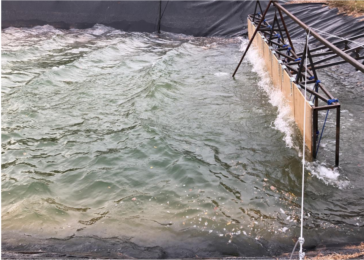
Figure 6: Wave generator used for prototype system. Photo by Maxwell O'Brien (Oklahoma Water Survey)
