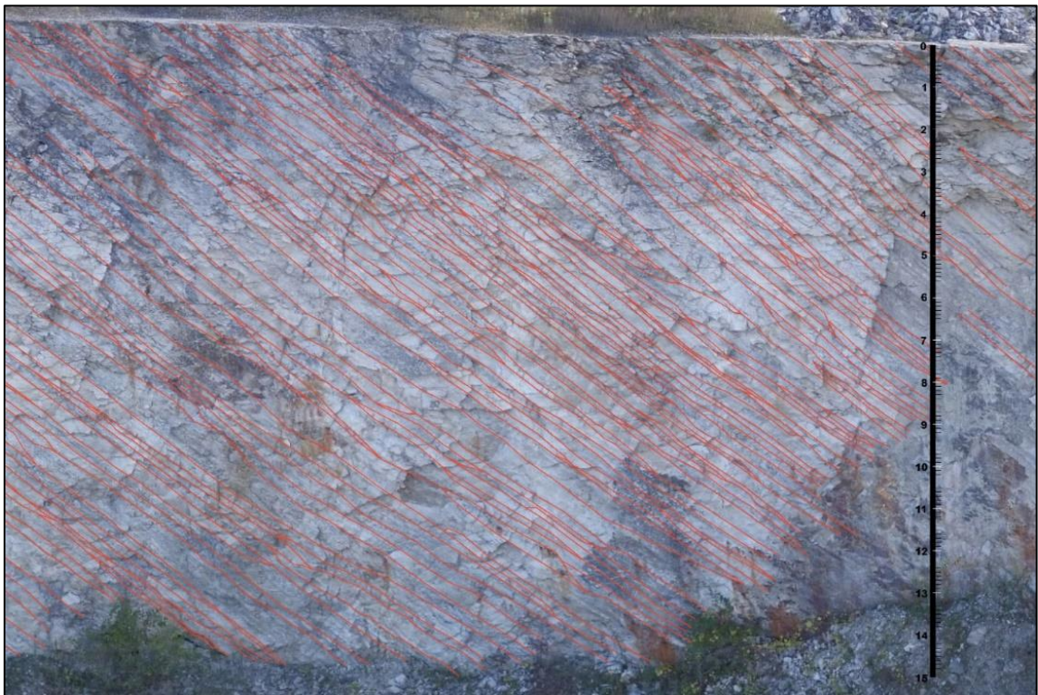
Figure 15: Bed tracings on a 21m section of the southern wall of the western section of the quarry. This was the first step in creating pseudo measured sections. In some sections of the wall, beds could not be traced or were indistinguishable. Note the ~40° apparent dip and the lenticular geometry of the beds. Scale bar is 15 m and is subdivided into meter and decimeter increments.
