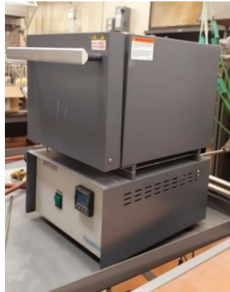
Figure 8: Oven used to dry the insulation layers
