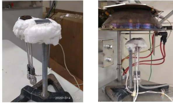
Figure 9: Experimental set up of Radiometer and PT under the cone calorimeter
