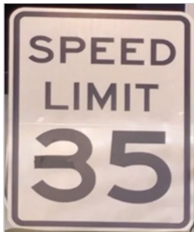
Figure 3. Attack on a speed limit sign in an experiment conducted by McAfee. Tesla car interpreted speed limit 35 as speed limit 85
