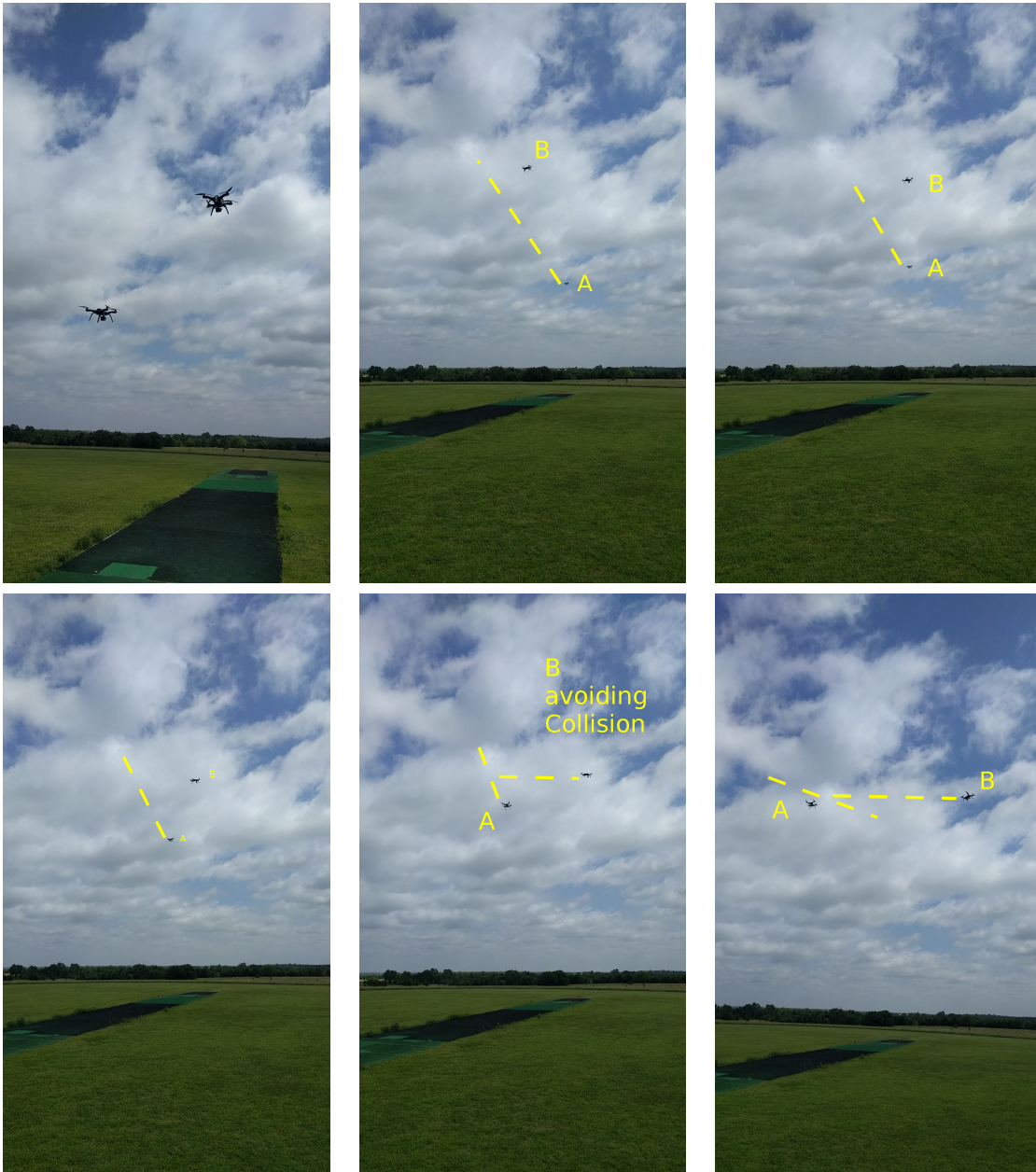
Figure 3.6: Experiment with two UAV robots A and B. (a) A started moving towards B. (b) B started moving away from A's path. (c) B is avoiding collision with A.
