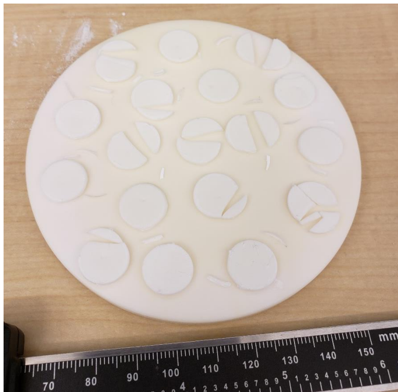
Figure 27: Alumina coated zirconia CS samples post-sintering.
