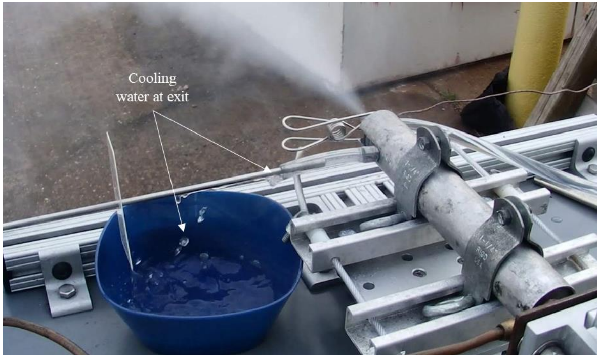
Figure 33: Single cooling passage nozzle during firing
