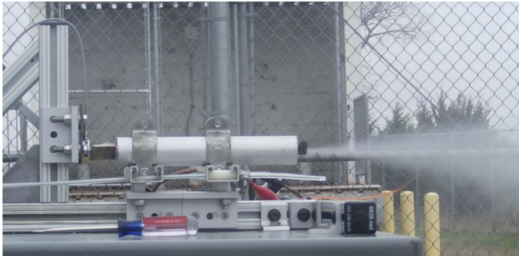
Figure 51: Gas generator performance validation test
