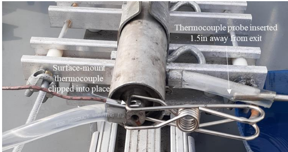
Figure 29: Thermocouples installed onto nozzle for firing
