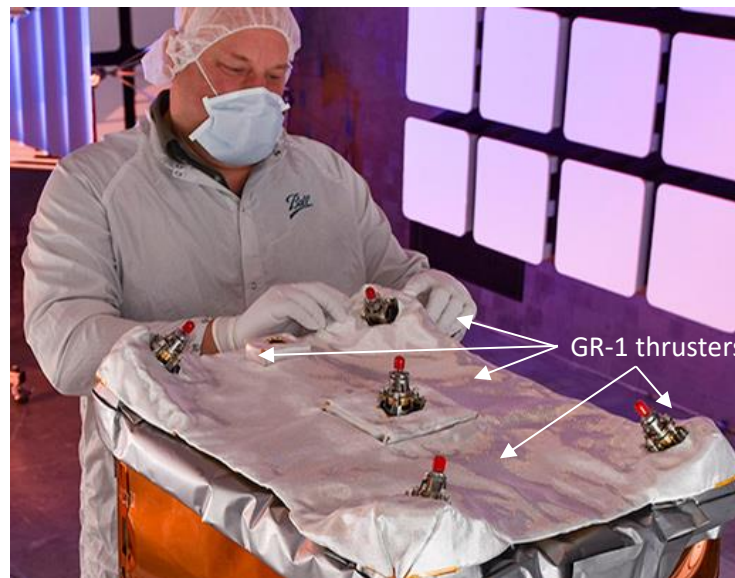
Figure 11: Integration of the (5) 1-N GR-1 thrusters to NASA's GPIM satellite [19]
