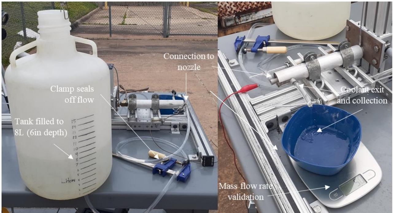
Figure 28: Water coolant flow setup prior to motor firing (left) and flow rate validation (right)
