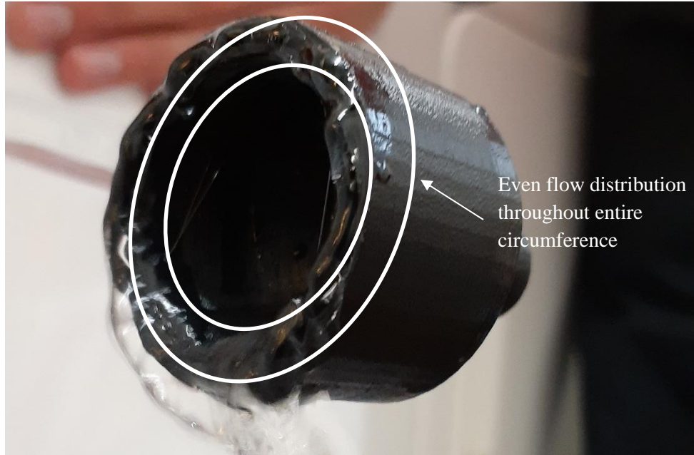
Figure 20: Test part to ensure even coolant inlet flow distribution within the nozzle
