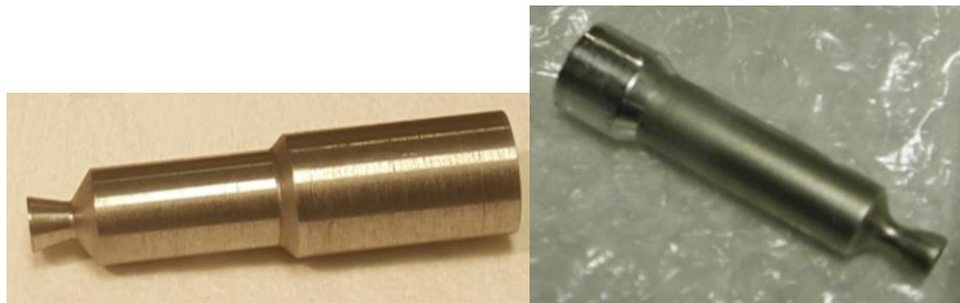
Figure 12: TZM thruster (left) vs iridium thruster (right) used by McGee with AF-M315E [21]
