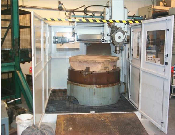
Figure 1.5: Single cutter VTL testing device with rock installed (Hellvik et al. 2012)
