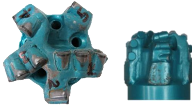
Figure 3.10: Ulterra 3.75 inch 5 blade (Raymond et al. 2015)
