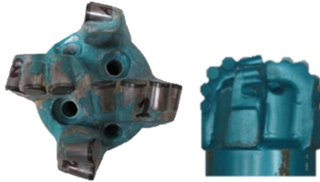
Figure 3.9: Ulterra 3.75 inch 4 blade (Raymond et al. 2015)
