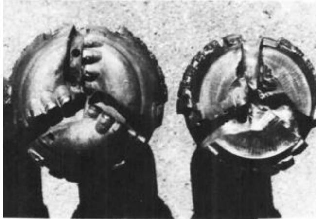
Figure 2.1: Premature wear of bits due to large fluid area (Huang and Iverson 1981)
