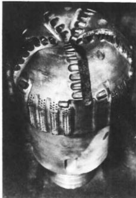
Figure 2.2: Buildup of tightly packed shale particles on the blades of a balled bit (Huang and Iverson 1981)
