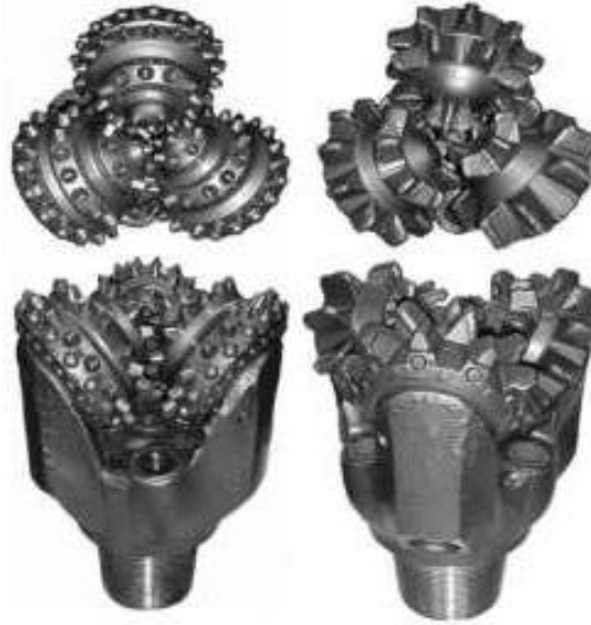
Figure 1.1: Example of roller cone button bit (left) and mill tooth bit (right) (Sheikhnejad et al. 2014)
