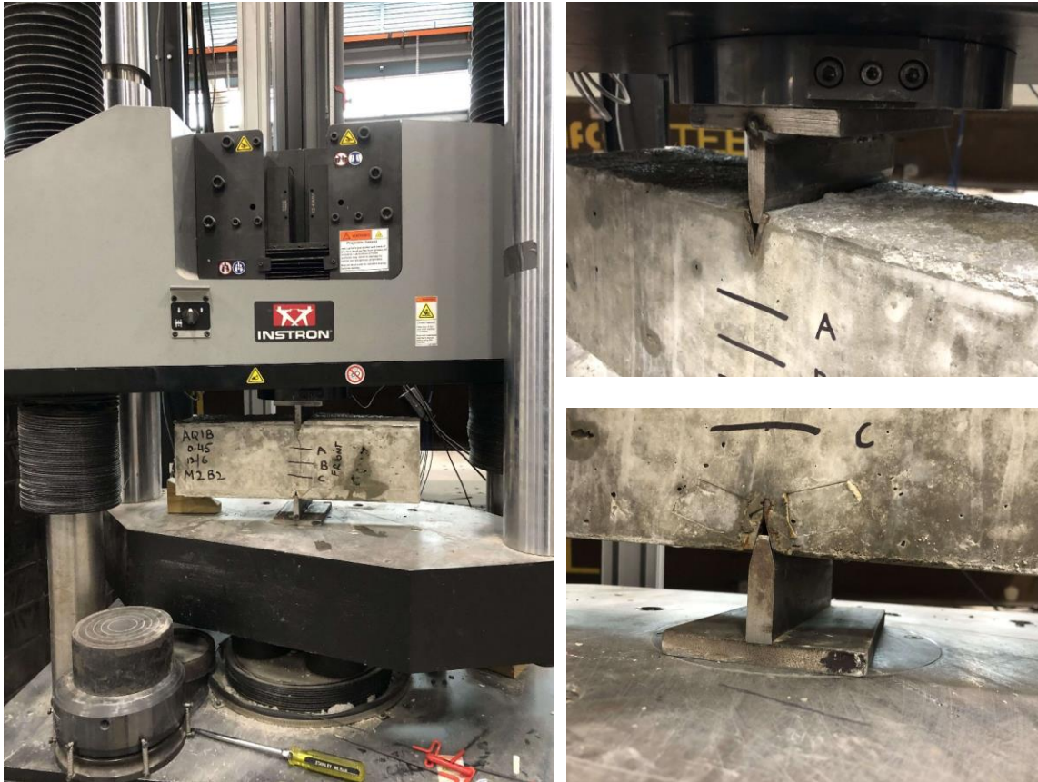
Figure I- 2: Assembly of Instron 1500 HDX with the beam mounted on loading heads
