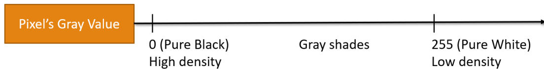
Figure II- 7: Correlation of gray scale values, brightness, and density
