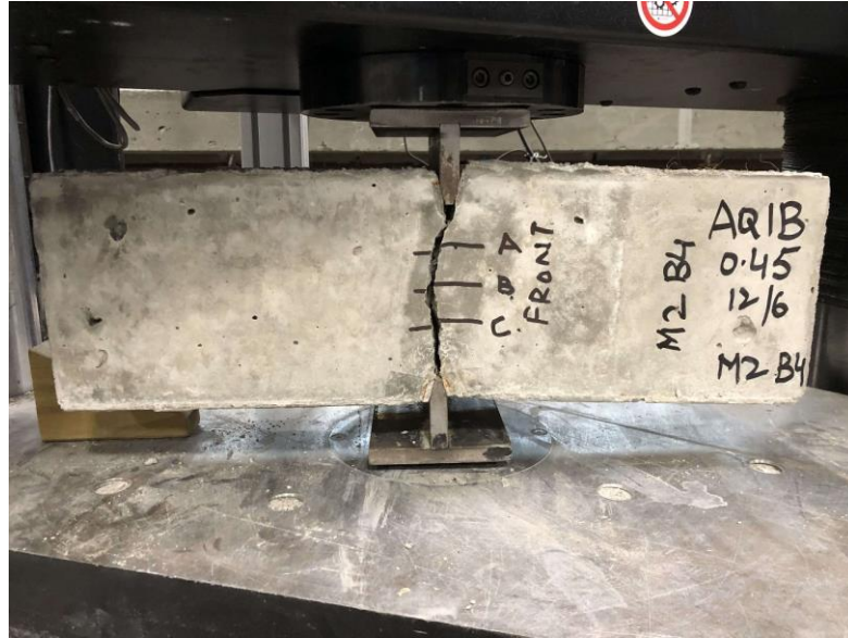
Figure I- 3:Crack propagation in beams
