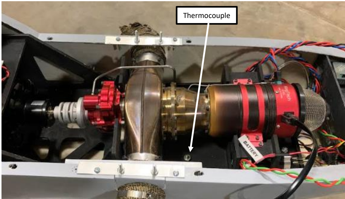
Figure 42. Photo of K-Type thermocouple location relative to turbine exhaust
