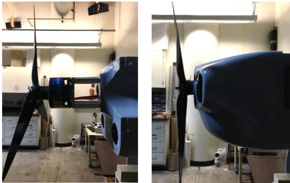
Figure 30. Photo of propeller motor with standoffs, with and without cowling
