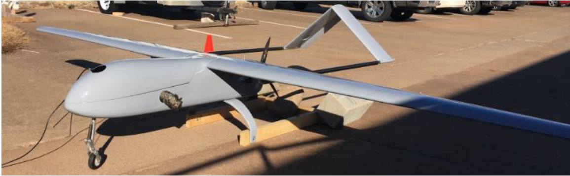
Figure 41. Photo of the Mugin 4500 test article, integrated with turboelectric propulsion and power system
