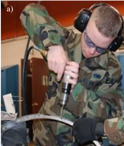
Figure 4: Mechanical drilling for fastener removal illustrating the operation, (a.) debris generated during operation, and (b.) damage to the workpiece (Photos courtesy of PPedm)
