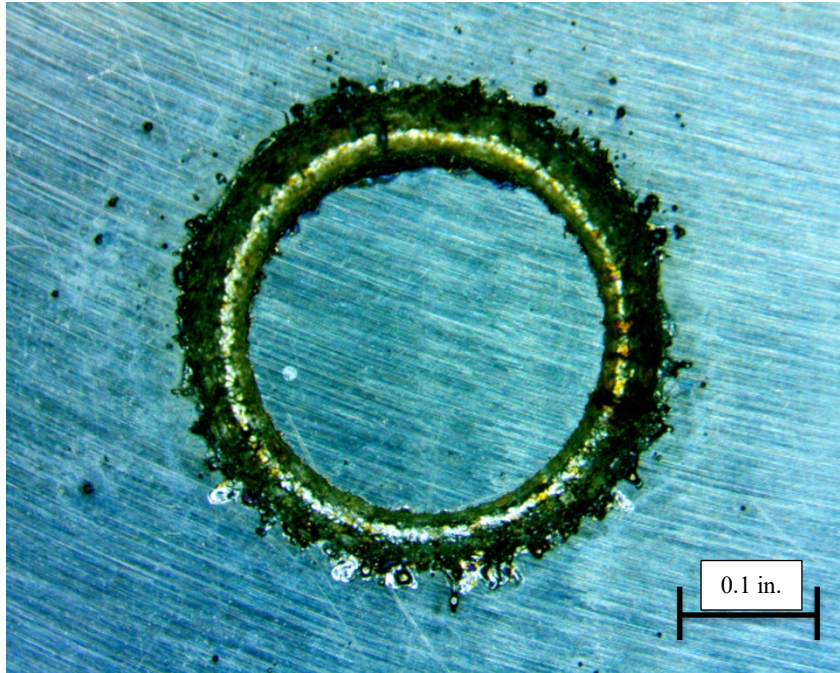
Figure 63: Task 2.1 Cut 1 with a Cut Depth of 0.05 in., an Electrode Diameter of 0.33 in., and a Fastener Material of Titanium
