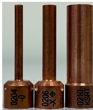
Figure 10: Electrodes Used in Study with Diameters of 0.125 in., 0.1875 in., and 0.33 in.
