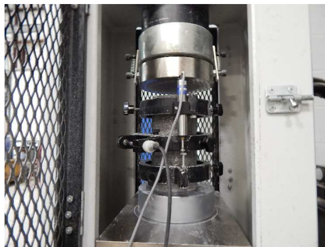
Figure 3: Example of a cylindrical sample and Modulus of Elasticity Testing
