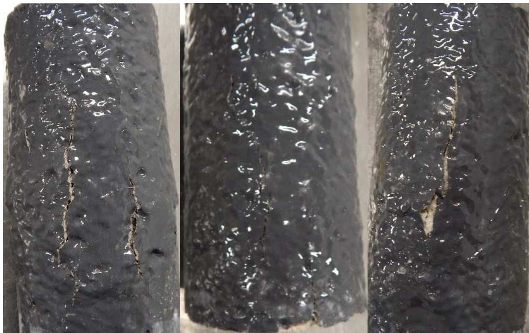
Figure 40: DYNA-PUR7416 (REG) failure type with a) one coat, b) two coats, and c) three coats
