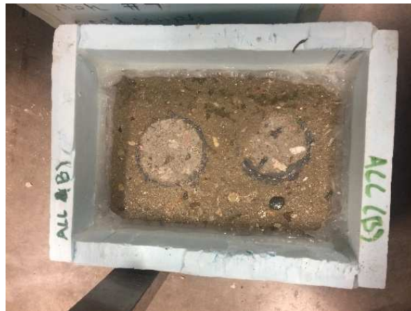
Figure 6: Pull-off testing of salt ponding samples
