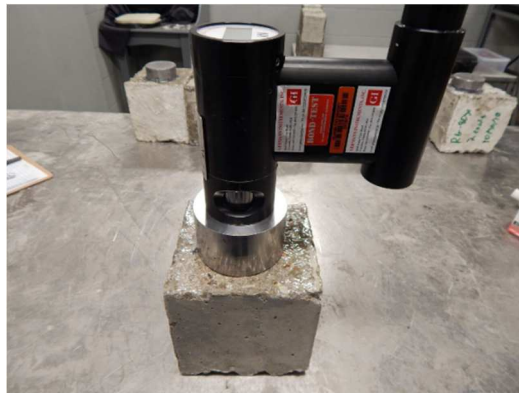
Figure 1: Example of Pull-off Testing
