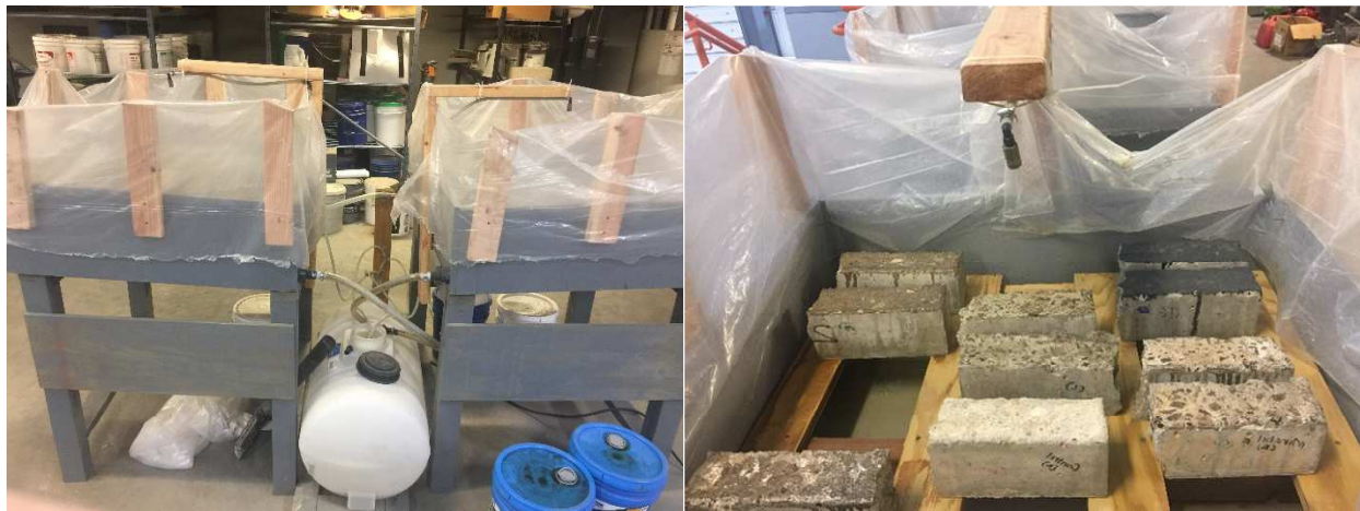
Figure 7: Cyclic wet-dry exposure setup (rain precipitation simulation)
