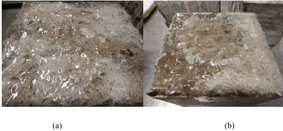
Figure 9: (a) Rustoleum RG-80X disbondment prior to testing flaking and (b) VersaFlex Clear Seal flaking from the surface
