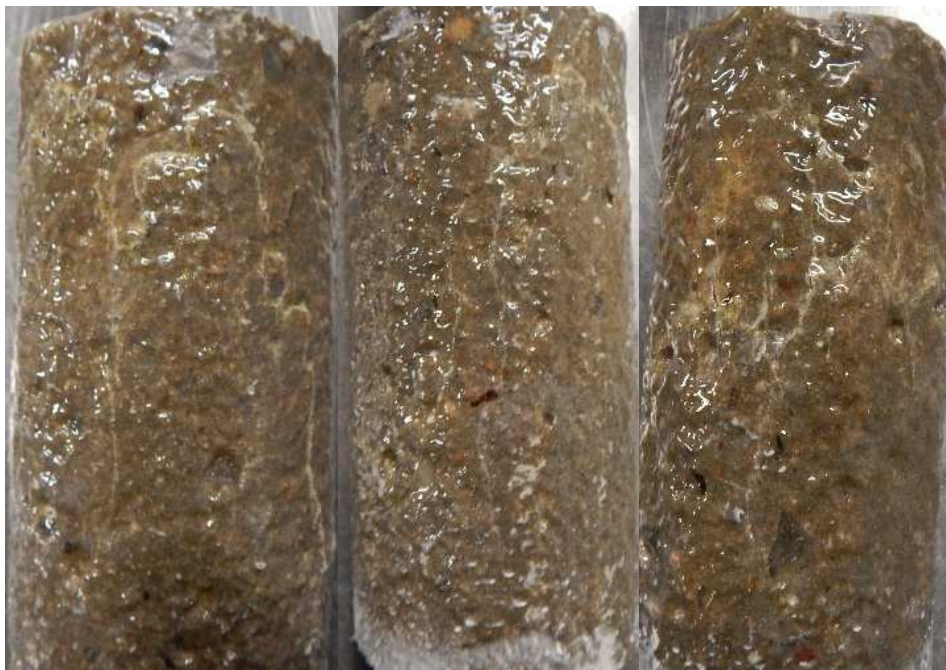
Figure 36: VersaFlex Aliphatic Clear Coat failure type with a) one coat, b) two coats, and c) three coats
