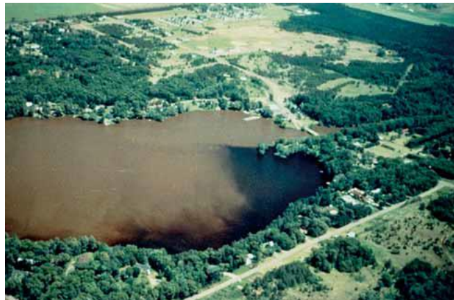
Figure 2-1 Sediment resulting from construction activity can diminish fish habitat, reduce oxygen levels, increase water temperatures, and reduce overall water quality [32].
