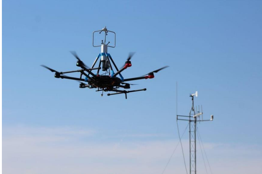
Figure 4.3. R.M. Young Model 81000 ultrasonic anemometer with Oklahoma Mesonet tower in background. (Photo: Jamey Jacob).
