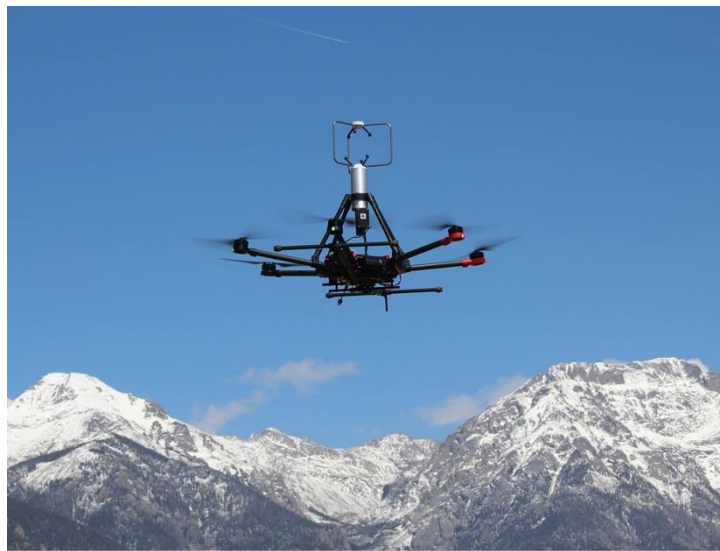
Figure 3.4. DJI Matrice 600 hexacopter outfitted with a Young Model 81000 ultrasonic anemometer on top (Photo: Jamey Jacob).
