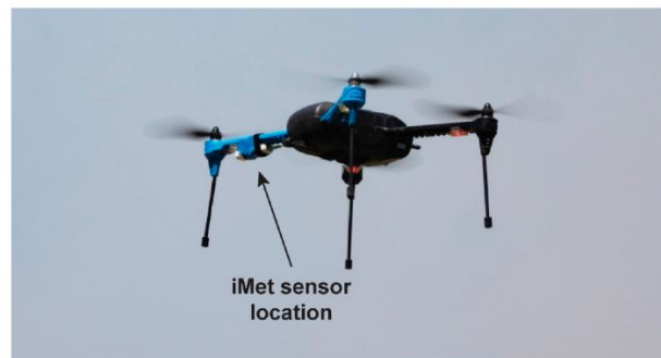
Figure 2.3. Location of iMet sensor placement on Iris+ sUAS platform.
