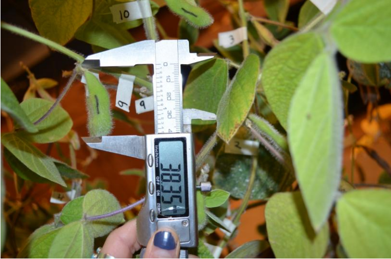
Figure 4.2. Digital calipers were utilized to measure pod growth parameters such as length (shown) and width.
