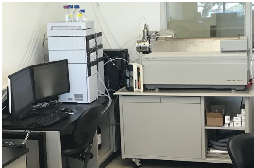
Figure 13. LC-MS/MS instrumentation setup at the OSU-FTTL. Shimadzu 20-series UFLC pumps paired with a Sciex 4000 QTRAP ® MS/MS.
