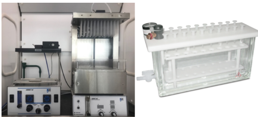
Figure 12. CEREX 48 Flow Control Unit (left), CEREX 48 Sample Concentrator (middle), and VacElut 20 manifold (right) used for SPE.
