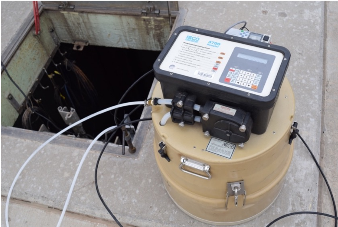
Figure 5. ISCO 3700 autosampler with silicon tubing. Water is moved by peristaltic pump from the wastewater system into polypropylene bottles housed within the body of the autosampler.
