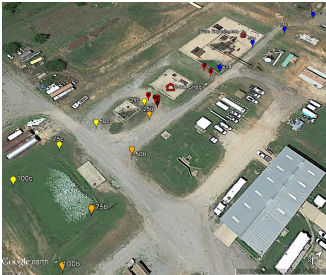
Figure 31. GMAP vehicle and SPod sampling locations at the Oklahoma State University Fire Research and Training Center. Red pins represent the GMAP vehicle locations while the blue, orange, and yellow pins represent the SPod locations (See Table 14). The red house icon denotes the One Pot production site.
