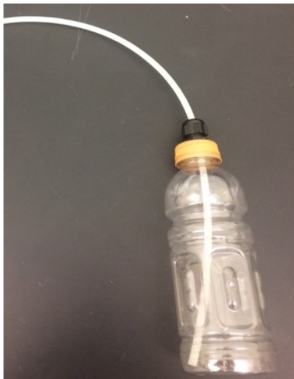
Figure 21. A typical hydrogen chloride gas generator, comprised of a plastic bottle with a hole in the cap and a hose protruding from the hole.
