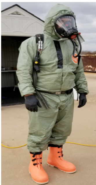
Figure 18. Level B protective suit, including chemically and thermally protective suits and a self-contained breathing apparatus
