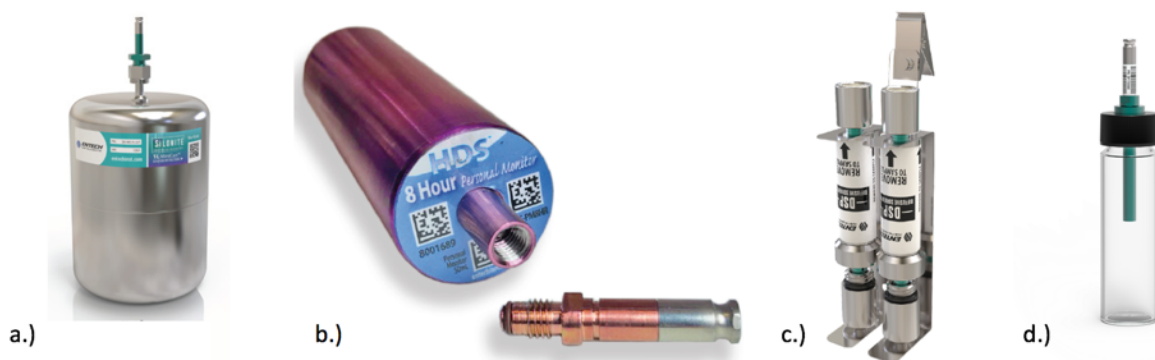
Figure 27. Passive air monitors provided by Entech Instruments for capturing air contaminants during One Pot cooks. a.) 1L Minican™ vacuum canister, b.) Helium diffusion sampler (HDS), c.) A set of diffusive sorbent pens (DSPs), one packed with Carbo Pack X and one packed with Tenax TA sorbent, and d.) a 40 mL screw-top grab sampler.
