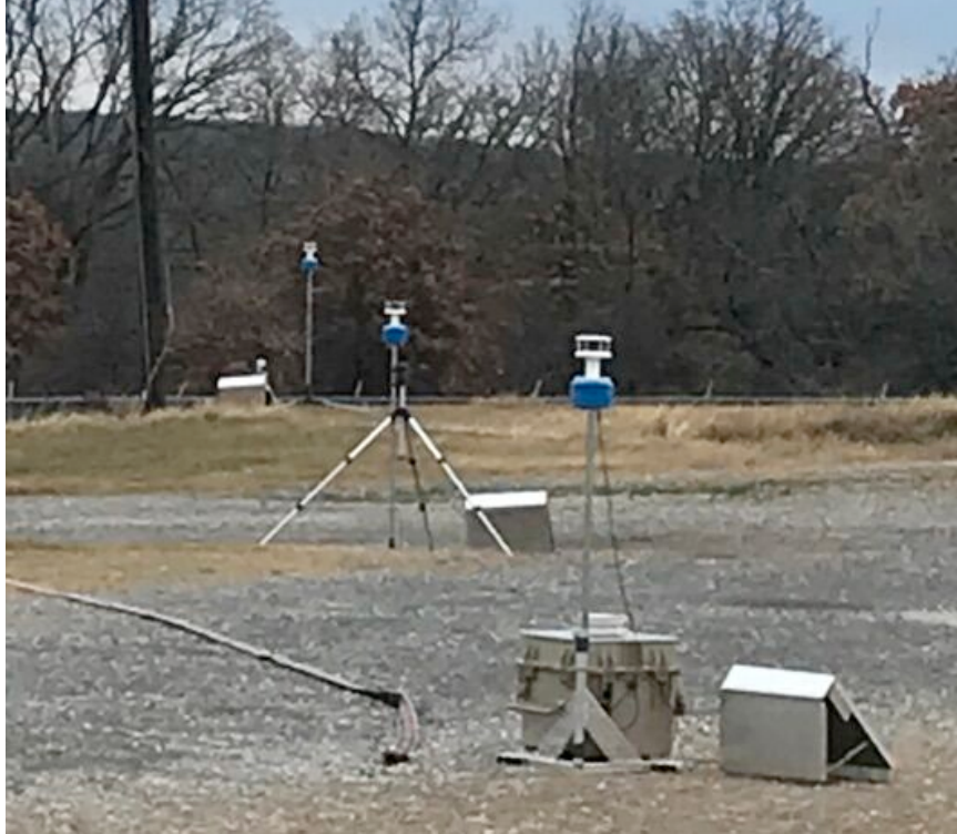
Figure 34. Three SPods deployed at 50, 75, and 100 m from the One Pot methamphetamine cook shed.
