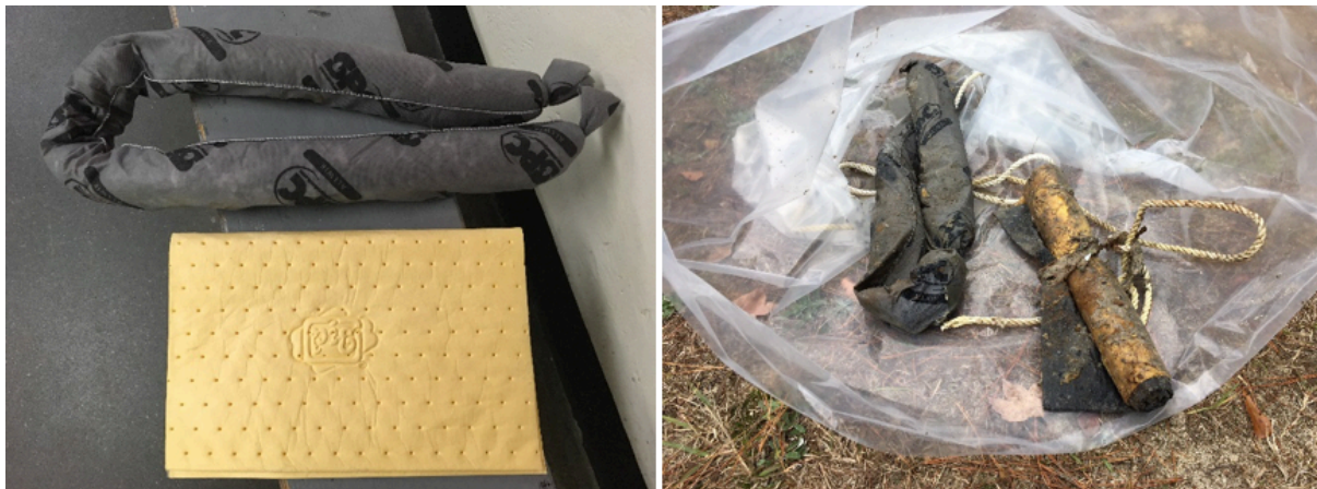
Figure 11. Polypropylene industrial sorbent sock (black) and industrial sorbent pads (yellow) used to collect SC 70 and 71. The left image shows the sorbents prior to being submerged in wastewater and the right image shows the sorbents following retrieval.
