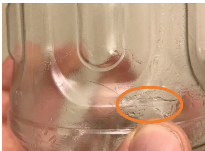
Figure 37. A hole formed in the One Pot reaction vessel of the final camp fuel cook due to repeated expansion and relaxation of the plastic.
