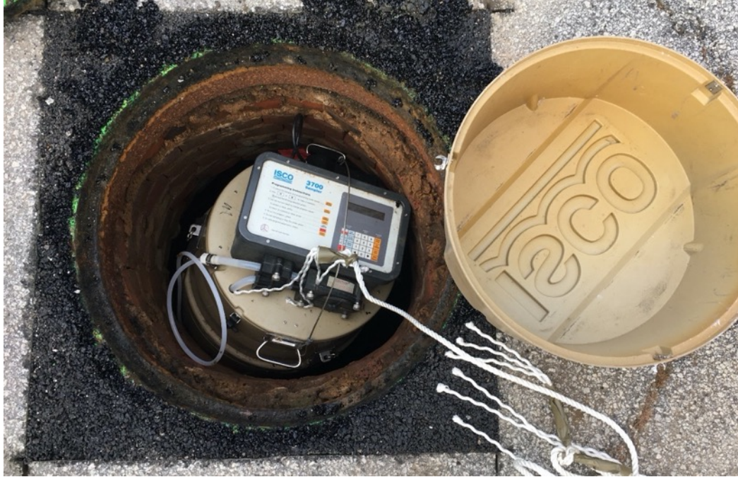
Figure 9. ISCO 3700 autosampler positioned inside the manhole at the headwater gravity line where composite samples SC 57-69 were collected. Headwater gravity line was located at the end of a residential block and served approximately 30 residences with no other known feeders.
