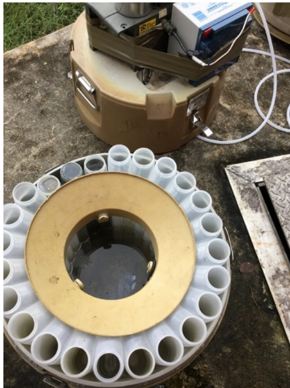
Figure 7. Spillage from SC 36-38 was contained within the autosampler housing, collected, and reported as SC 39.
