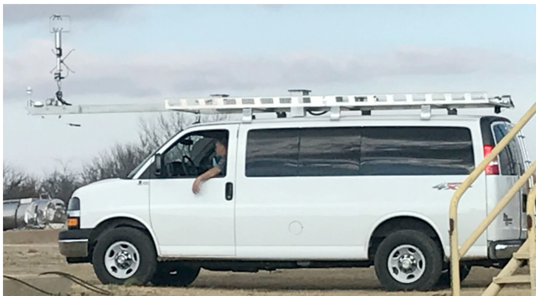
Figure 30. The GMAP vehicle operated by EPA-NEIC. On-board instrumentation includes an ICOS, PID, DUVAS, GPS, a meteorological station, and an air canister collection mechanism.
