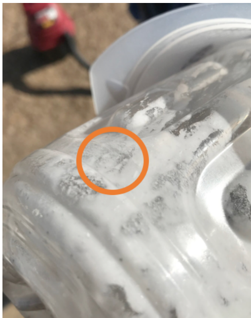
Figure 36. A hole formed in the One Pot reaction vessel of the second camp fuel cook due to repeated expansion and relaxation of the plastic.
