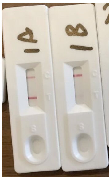
Figure 77. Competitive lateral flow immunoassay cassette developed by CDC-NIOSH for detection of methamphetamine at a concentration of 50 ng/100 cm 2 . Sample 1A was taken pre-cook and sample 1B was taken from the same location post-cook. Two red lines indicate the absence of methamphetamine in the sample. One red line indicates the presence of methamphetamine in the sample.
