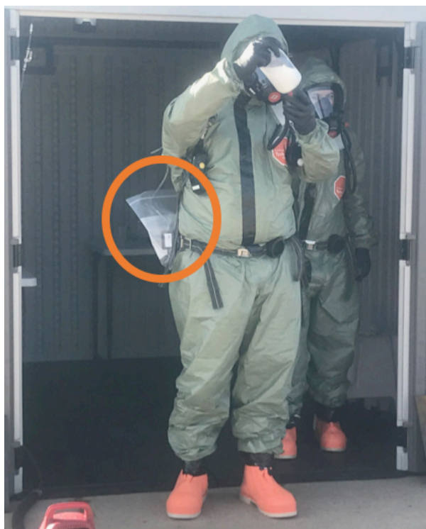
Figure 24. An SKC Airchek 2000 active air sampler fitted to a researcher as they performed a One Pot methamphetamine cook.
