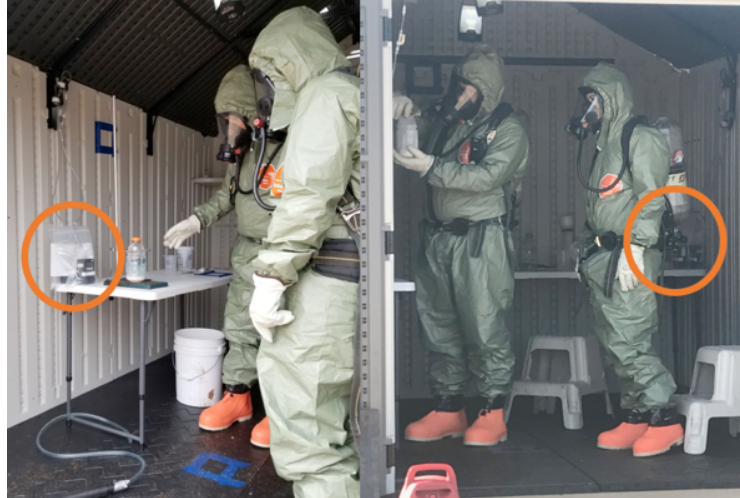
Figure 25. Locations of 4 out of 5 active air samplers. Two samplers were placed in each location designated by the orange circles. Two samplers were located left of the active One Pot methamphetamine lab and two samplers were located behind and to the right of the researchers performing the One Pot methamphetamine cooks.
