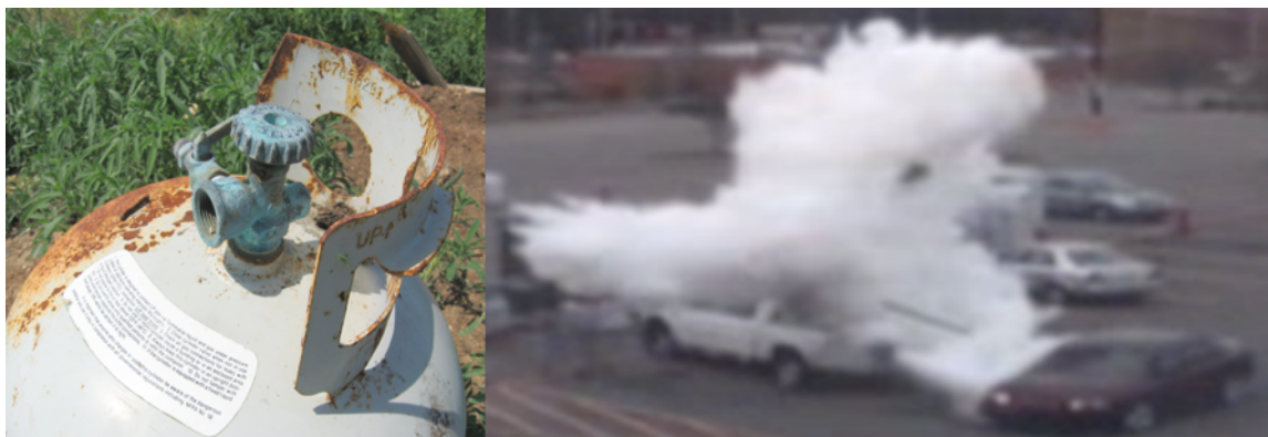
Figure 16. Left.) A propane tank used to illicitly transport anhydrous ammonia. The blue discoloration of the bronze fitting is indicative of the presence of ammonia. Right.) A vehicle illicitly transporting anhydrous ammonia in a propane tank when the tank's structural integrity became compromised, resulting in a plume of ammonia being released into the environment. Images adapted from the Clandestine Laboratory Safety Certificate Program Student Manual. 73
