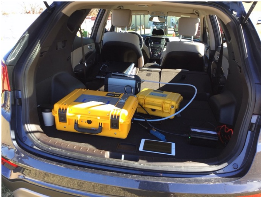
Figure 33. Configuration of battery-powered ICOS (larger yellow in foreground), vacuum pump (gray), battery pack (smaller yellow to right) as positioned in moving vehicle during data-logging. Trace background ammonia detected from vehicle exhaust was dampened or eliminated by opening all vehicle windows when vehicle was in motion or by shutting off the engine when parked.
