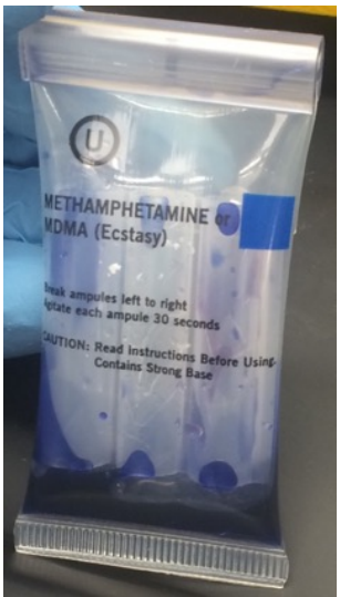
Figure 22. An example of a positive NIK Public Safety Narcotics Identification System presumptive colorimetric test. Test U: Methamphetamine and MDMA was used to identify the presence of methamphetamine in the salts produced by each One Pot.
