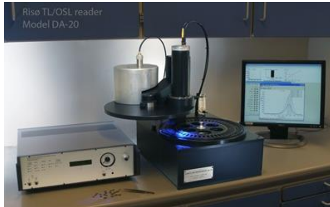
Figure 3-2. Risø TL/OSL reader, DTU Nutech 2014.
