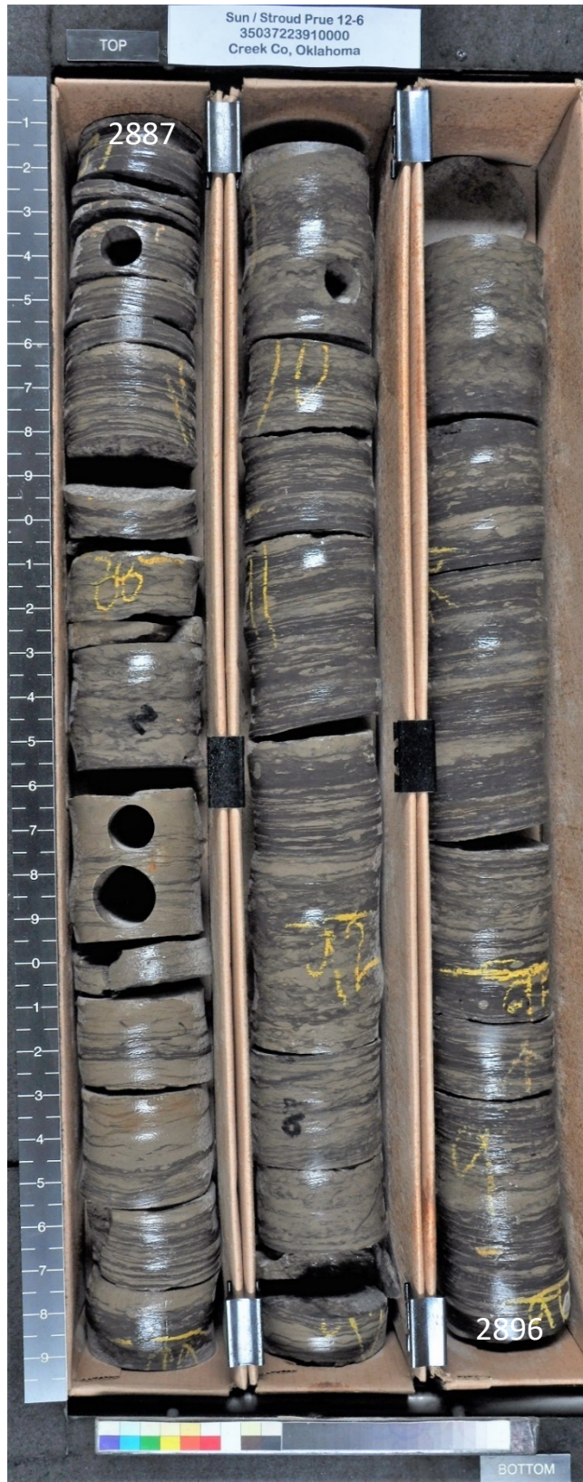
Core from the Stroud Prue Unit Tr. #12-6 covering the interval from 2887 to 2896.
