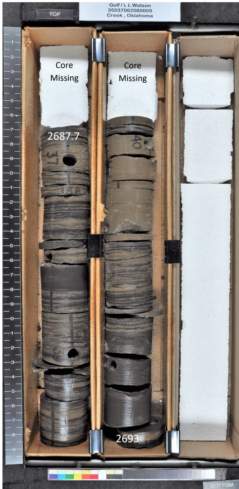
Figure 32. Core of Watson #1 from depth 2687.7 to 2693 feet. The core has abundant interbedded shale at the bottom of the core. The sandstone has rhythmic wavy and lenticular bedding with small-scale burrowing in the bottom of the core. Shale is the predominant lithology at 2692.1 feet. Scale bar indicates tenths of feet.
