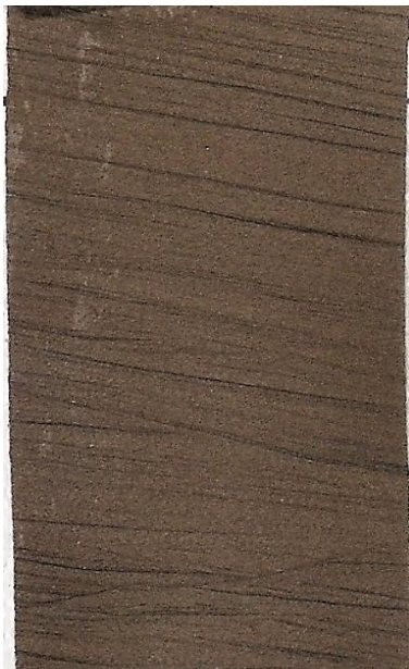
Figure 22. Close up of Yarhola Royalty #25 core showing the abundant cross bedding in the bottom half of the core at depth 2314 feet.
