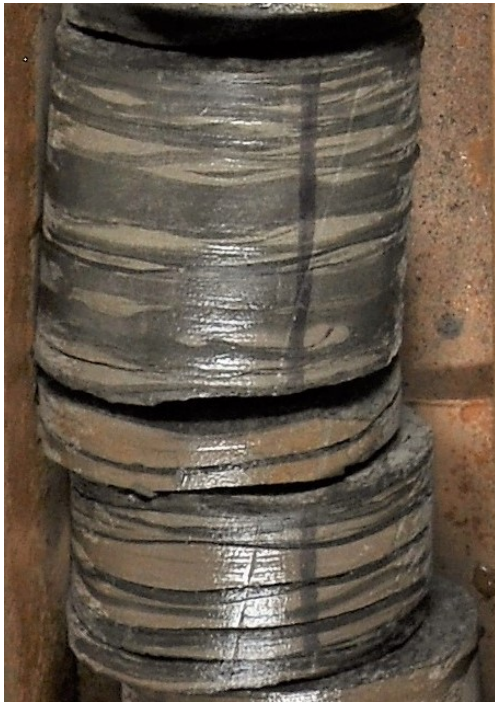
Figure 27. Close up of Watson #1 core showing the lenticular bedding at the top of the core at depth 2668.2 feet.
