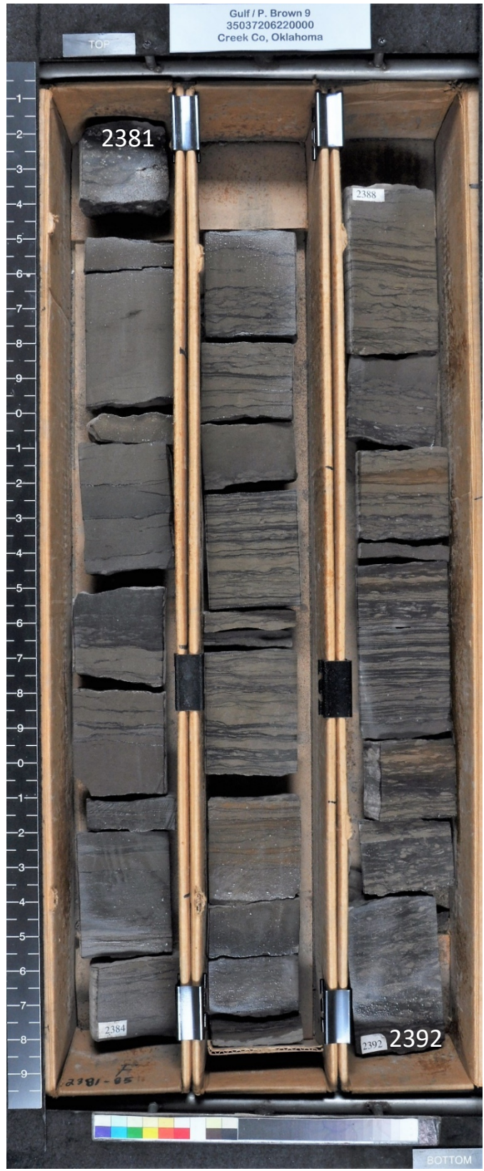
Entire slabbed core from Peter Brown #9 covering the interval from 2381 to 2392 feet.
