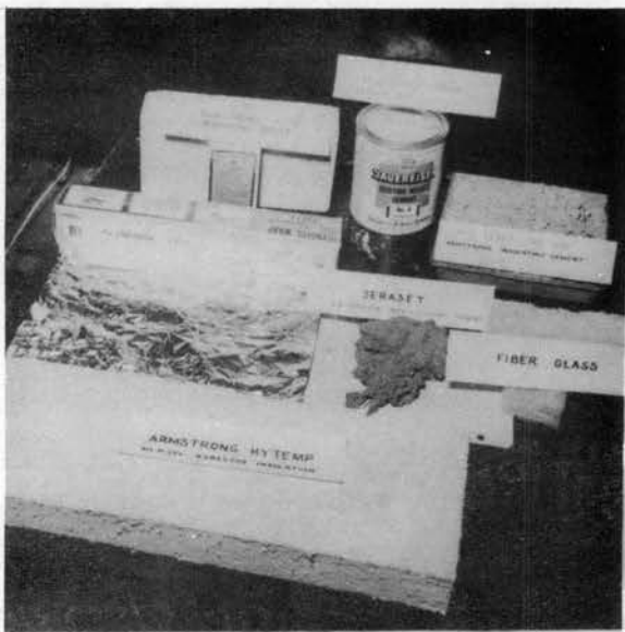
Figure 5. Insulating materials used in construction of furnace
