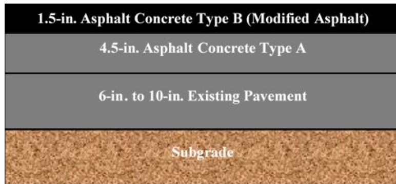
Figure 3.1 Typical pavement structures of US 287
