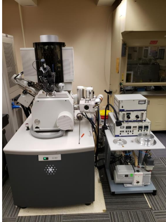
Figure 3.2 – FEI Helios Nanolab™ 650 DualBeam™ Scanning Electron Microscope
