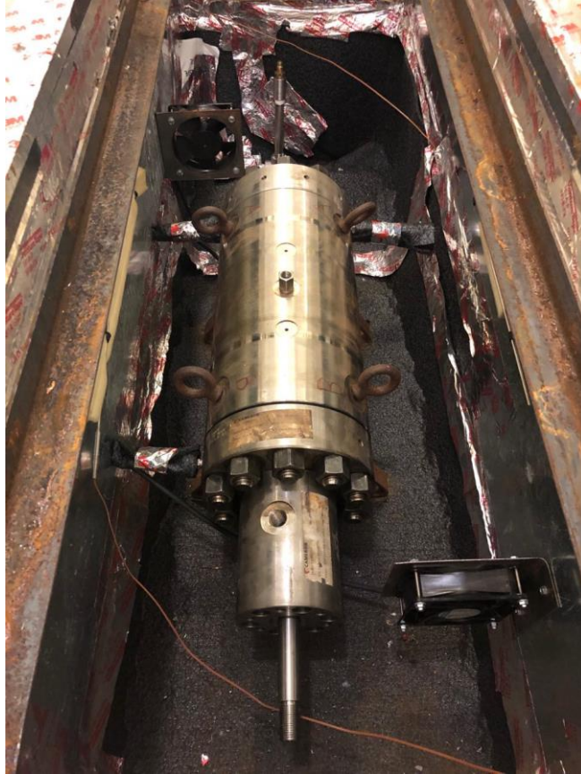
Figure 9 - Tubing of the inside of the box has been covered by insulation
