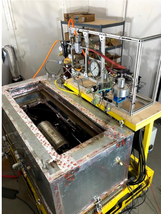
Figure 6 - High-Pressure Gas Supply, Test and Collection System (front)
