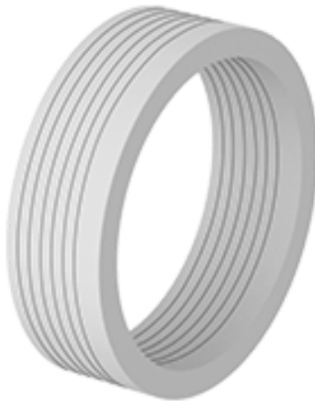
Figure 62 - Schematic of a generic plastic V-stack
