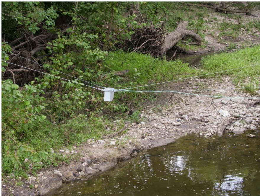
Figure 5: Cable mounted stream radar at Mill creek
