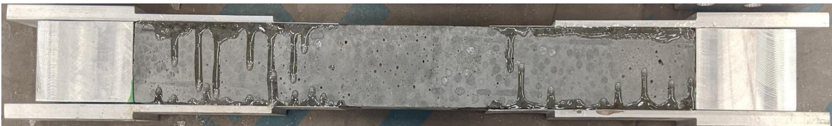
Figure 5.9 Ends Epoxied on FHWA Specimen
