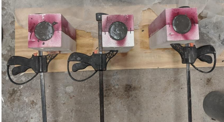
Figure A. 1 Setup for cylindrical dogbone casting
