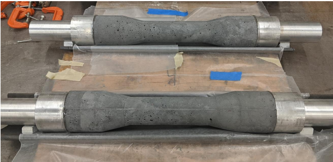
Figure 4.2 Cylindrical Dogbone Specimen Gluing Setup
