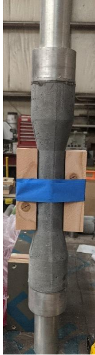
Figure 4.4 Spacer for LVDT Brackets
