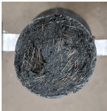
Figure 7.8 Example of Excessive Fiber Concentration
