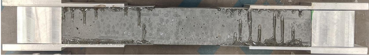
Figure 3.6 FHWA Specimen with end anchorages
