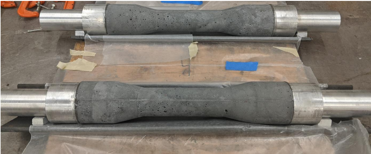
Figure A. 3 Cylindrical Dogbone Specimen Gluing Setup
