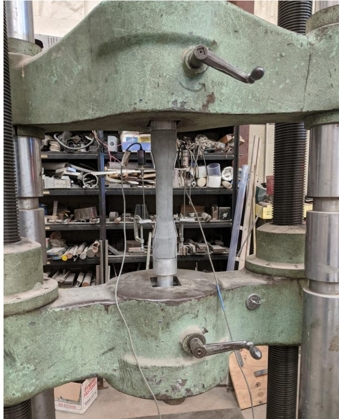
Figure 4.6 Cylindrical Dogbone in Baldwin with LVDTs
