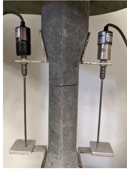
Figure 4.8 Multiple Crack Formation
