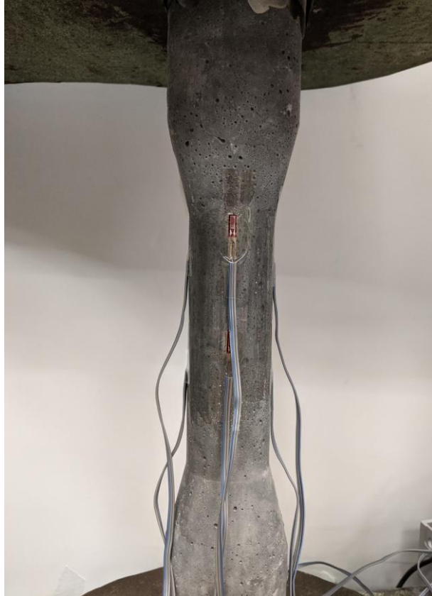
Figure 5.1 Strain Gauge Location on Cylindrical Dogbone Specimen
