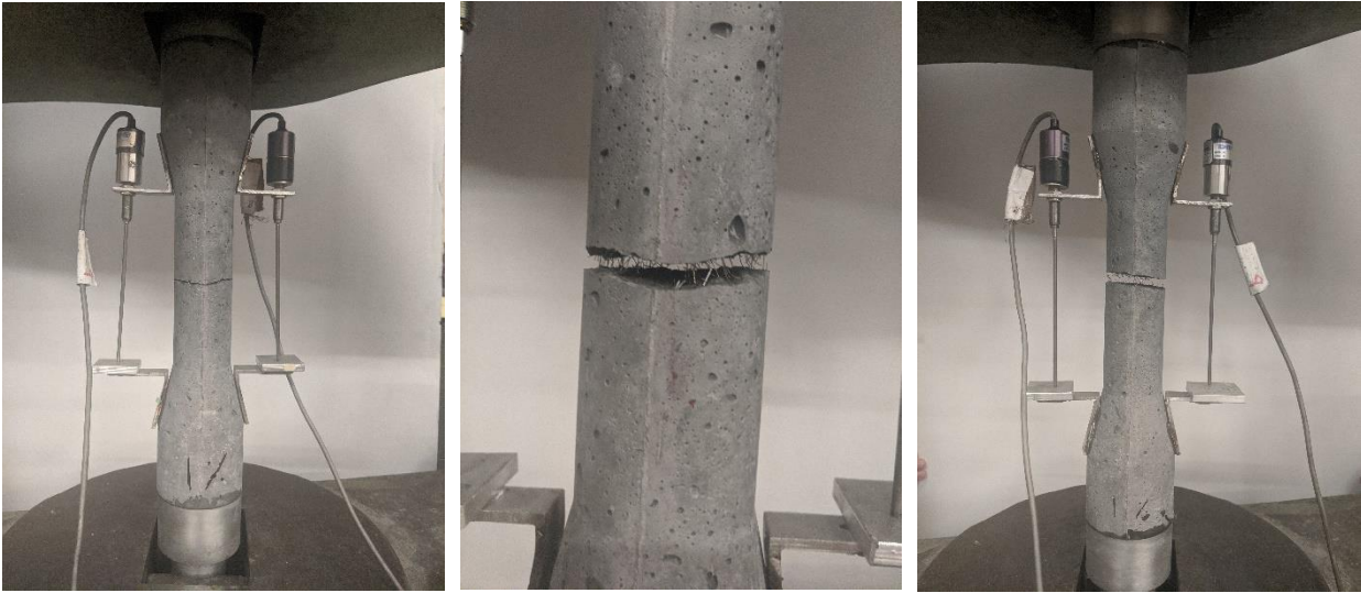
(a) (b) (c) Figure 4.9 (a) Initial Crack Location, (b) Fibers Bridging Crack, (c) Post Crack
