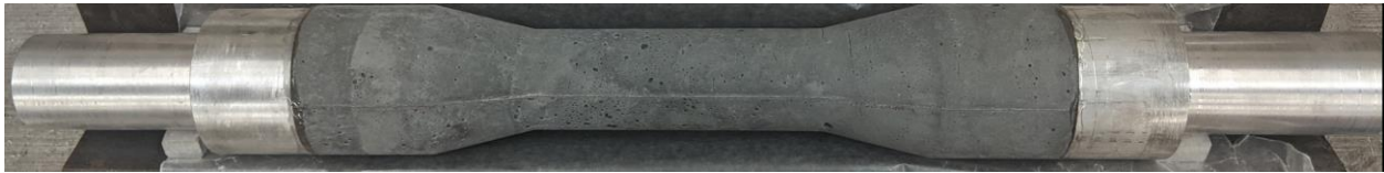
Figure 3.2 Cylindrical Dogbone Specimen with Aluminum Ends
