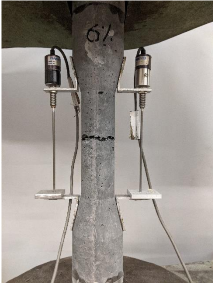
Figure 4.7 Crack Formation on Cylindrical Dogbone Specimen
