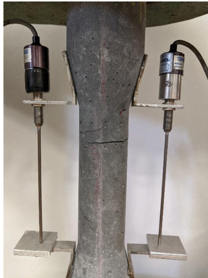
Figure A. 5 Multiple Crack Formation
