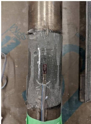
Figure 5.6 Strain Gauge Location for Cylindrical Specimen
