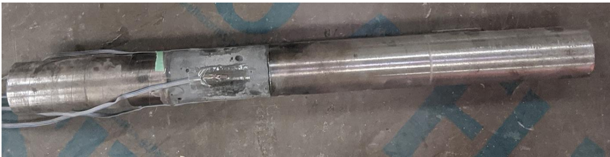
Figure 3.4 Cylinder Specimen with End Anchorages
