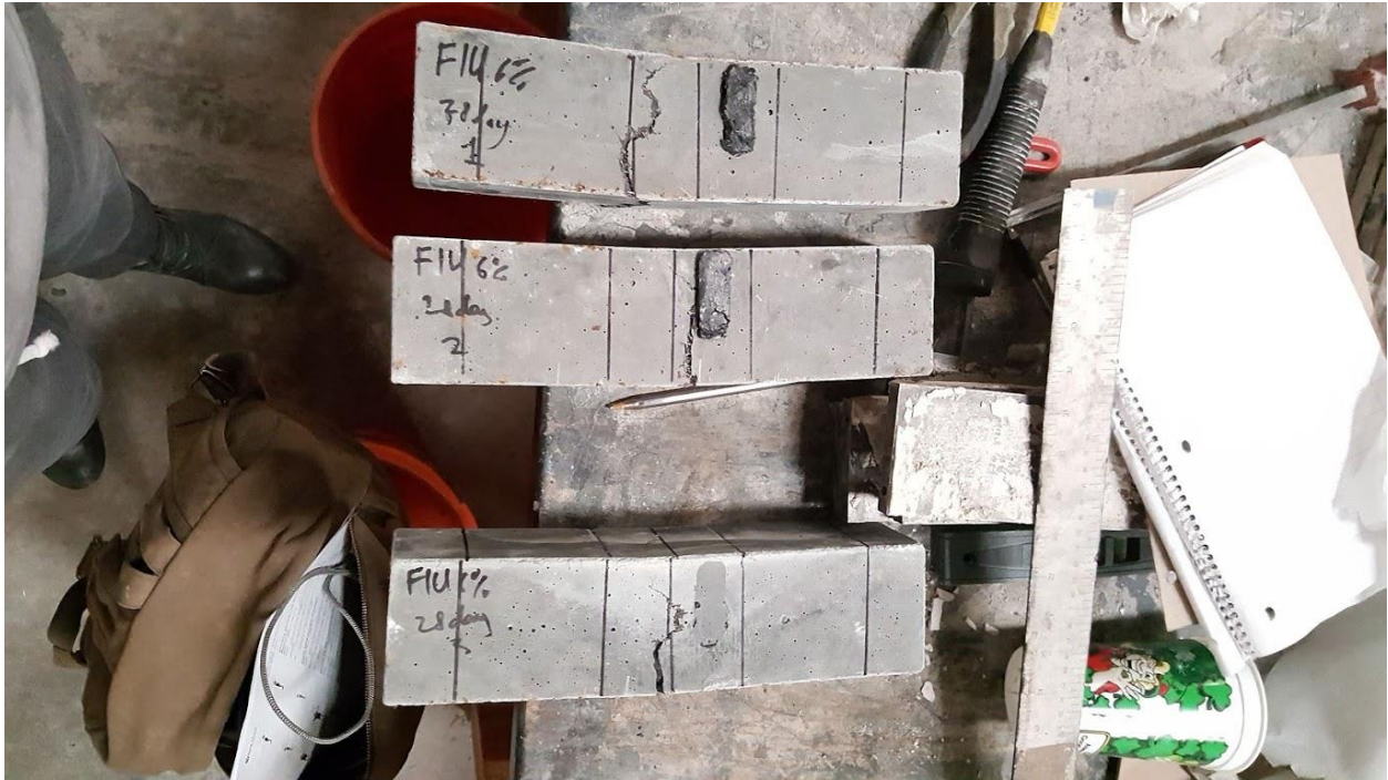
Figure 104: FIU J3 6% 28 day MOR test specimens after failure
