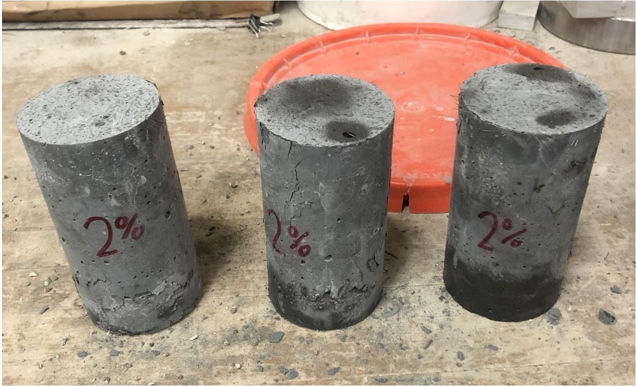
Figure 122: OU J3 2% cylinder 3 day compressive strength test specimens after failure
