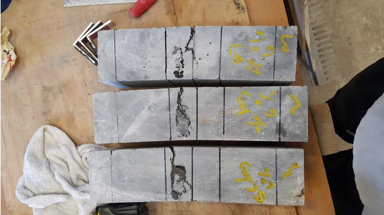
Figure 61: OU J3 6% 56 day MOR test specimens after failure
