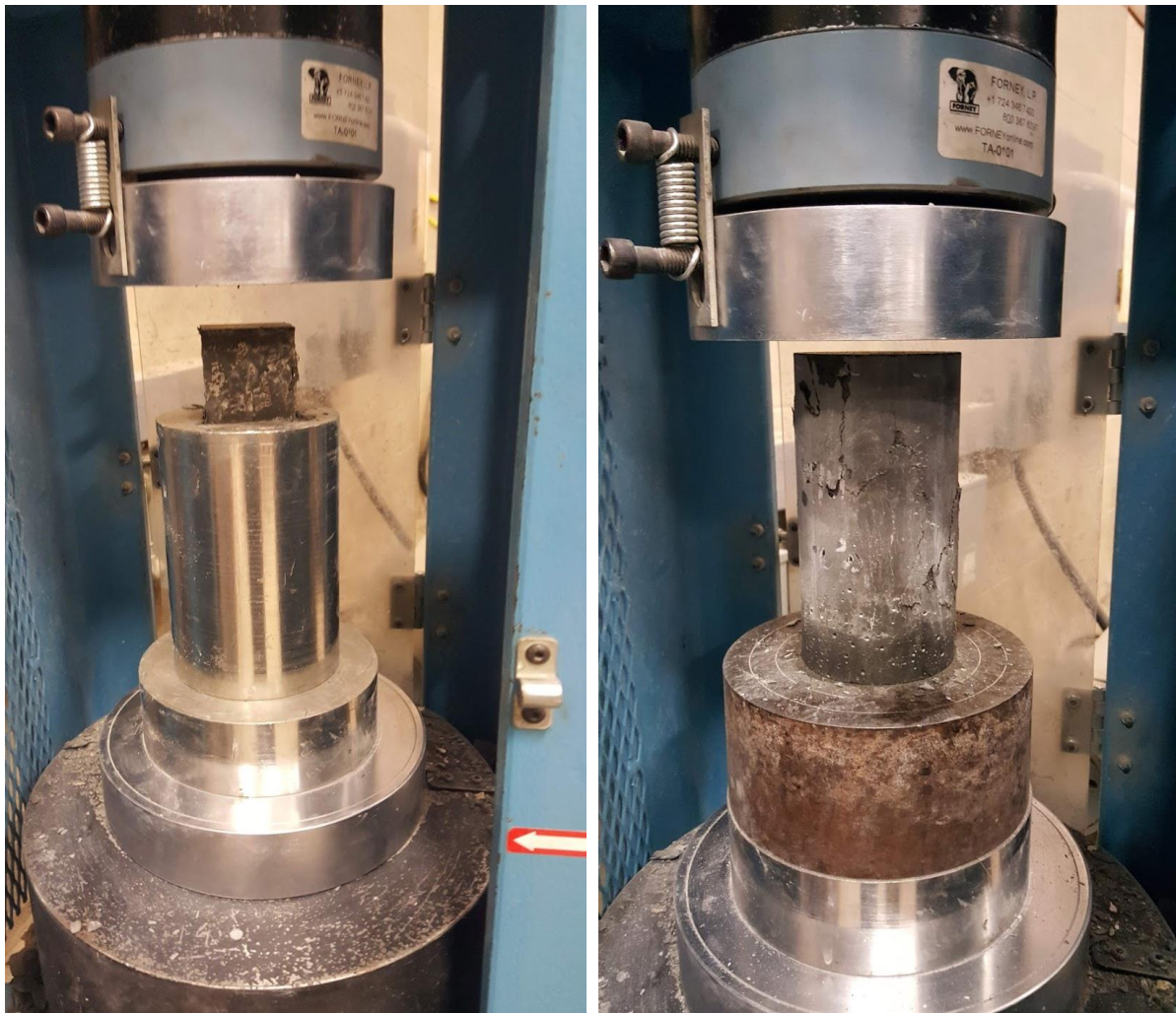
Figure 6: Standard compressive strength test set up for cube (left) and cylinder (right) specimens
