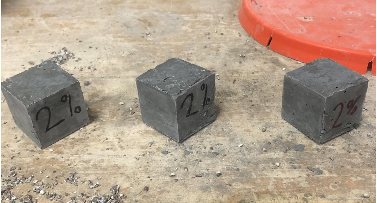
Figure 124: OU J3 2% cube 3 day compressive strength test specimens after failure
