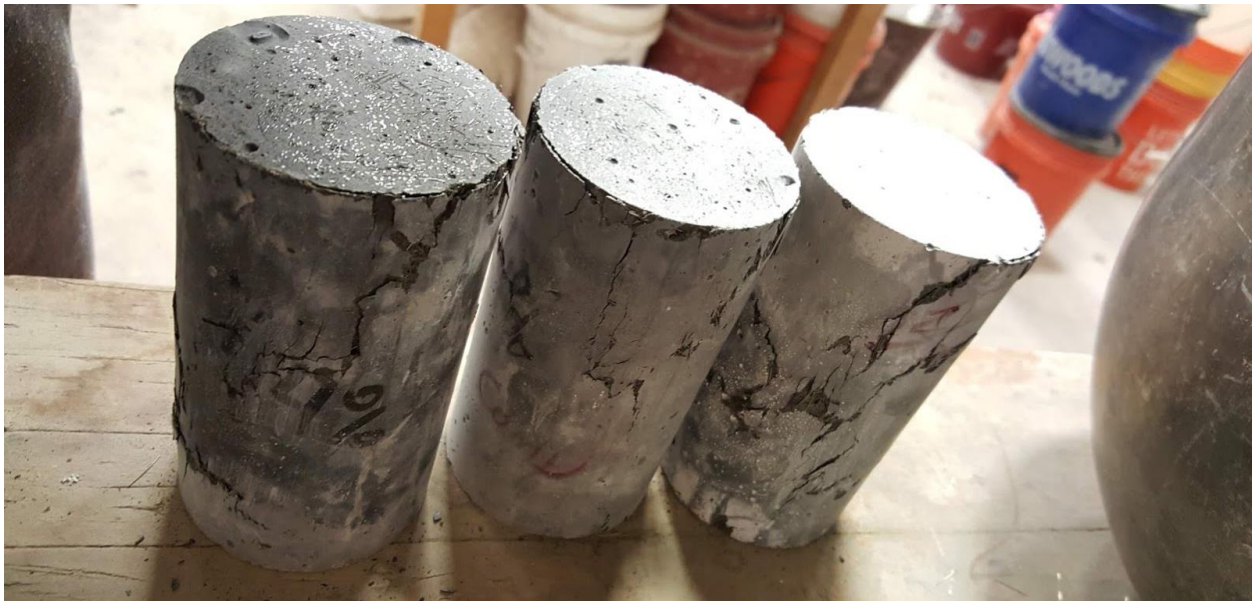
Figure 33: OU J3 4% cylinder 28 day compressive strength test specimens after failure
