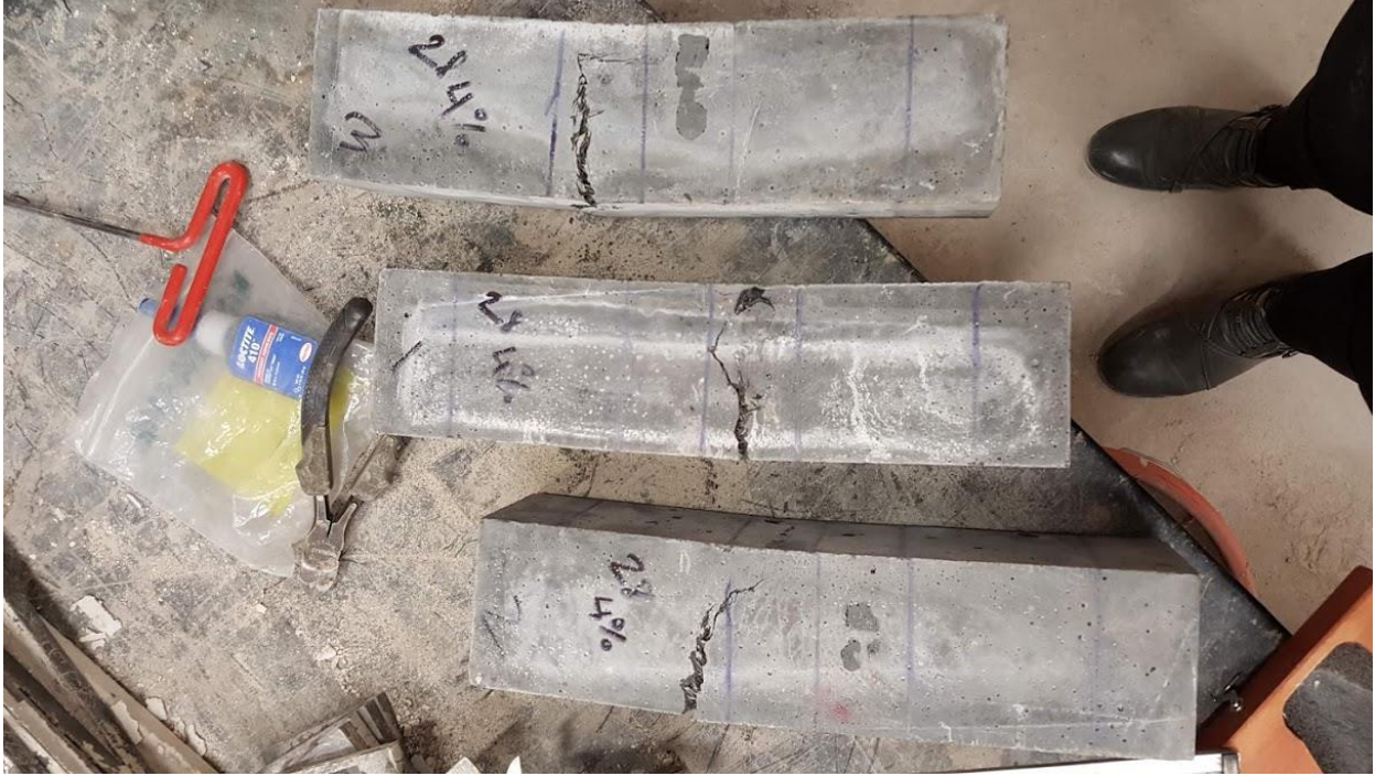
Figure 103: FIU J3 4% 28 day MOR test specimens after failure
