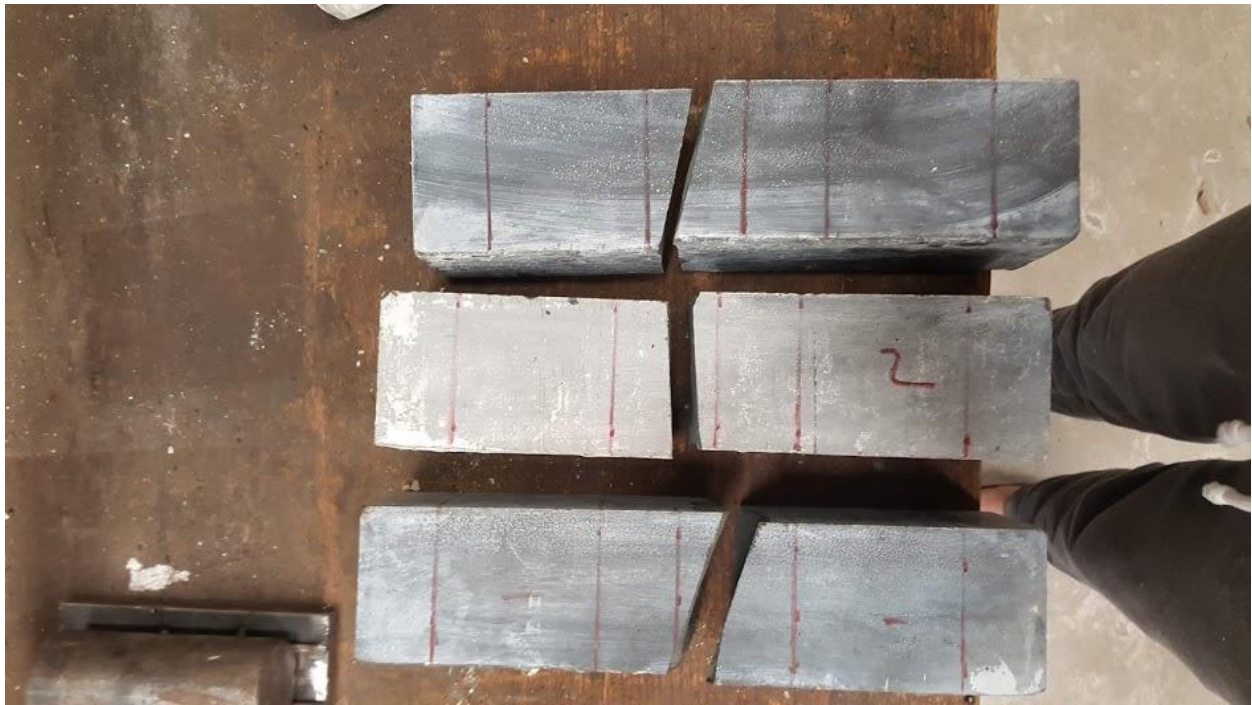
Figure 57: OU J3 0% 56 day MOR test specimens after failure
