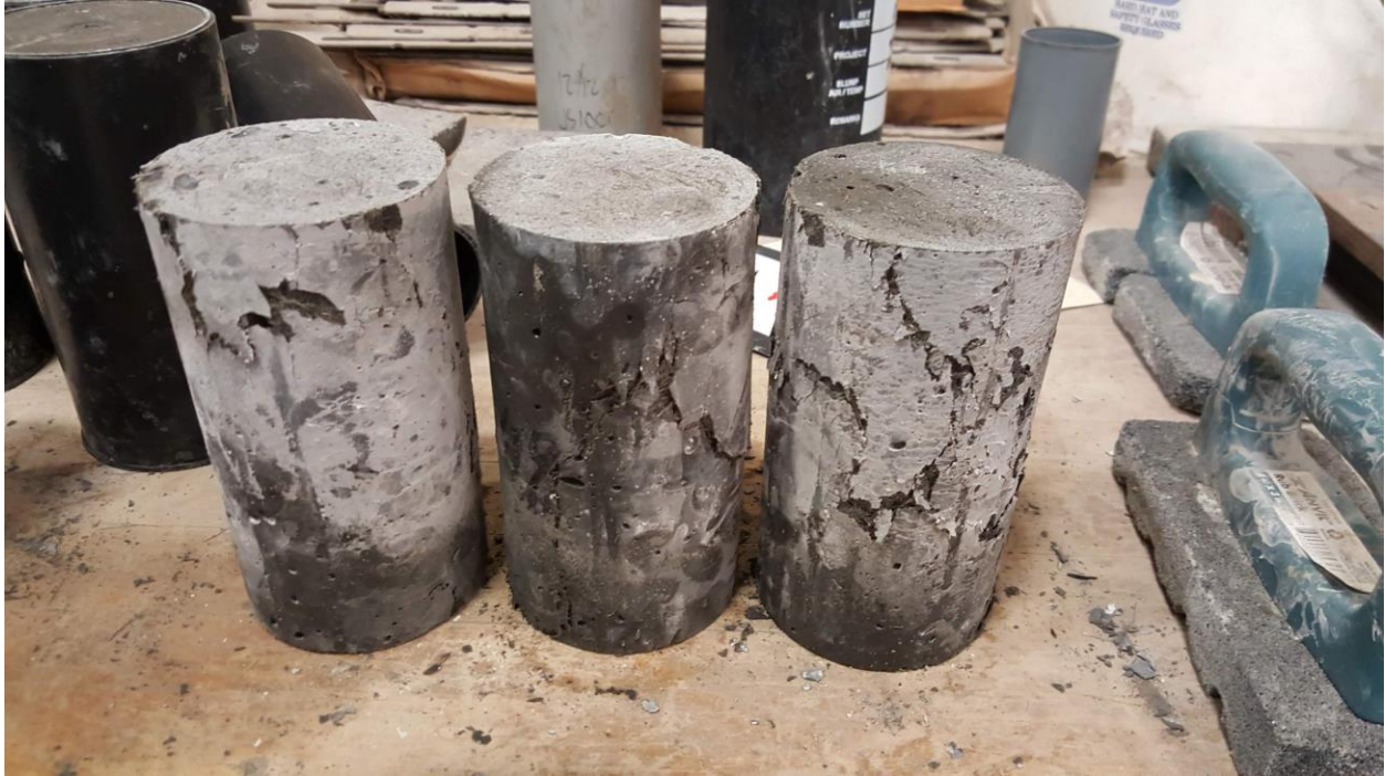
Figure 34: OU J3 4% cylinder 56 day compressive strength test specimens after failure
