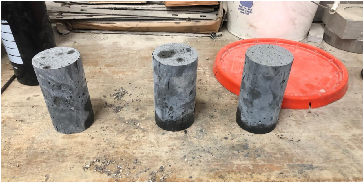
Figure 119: OU J3 1% cylinder 7 day compressive strength test specimens after failure
