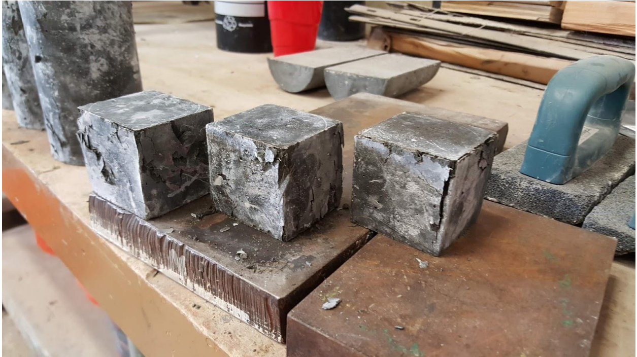
Figure 32: OU J3 2% cube 56 day compressive strength test specimens after failure
