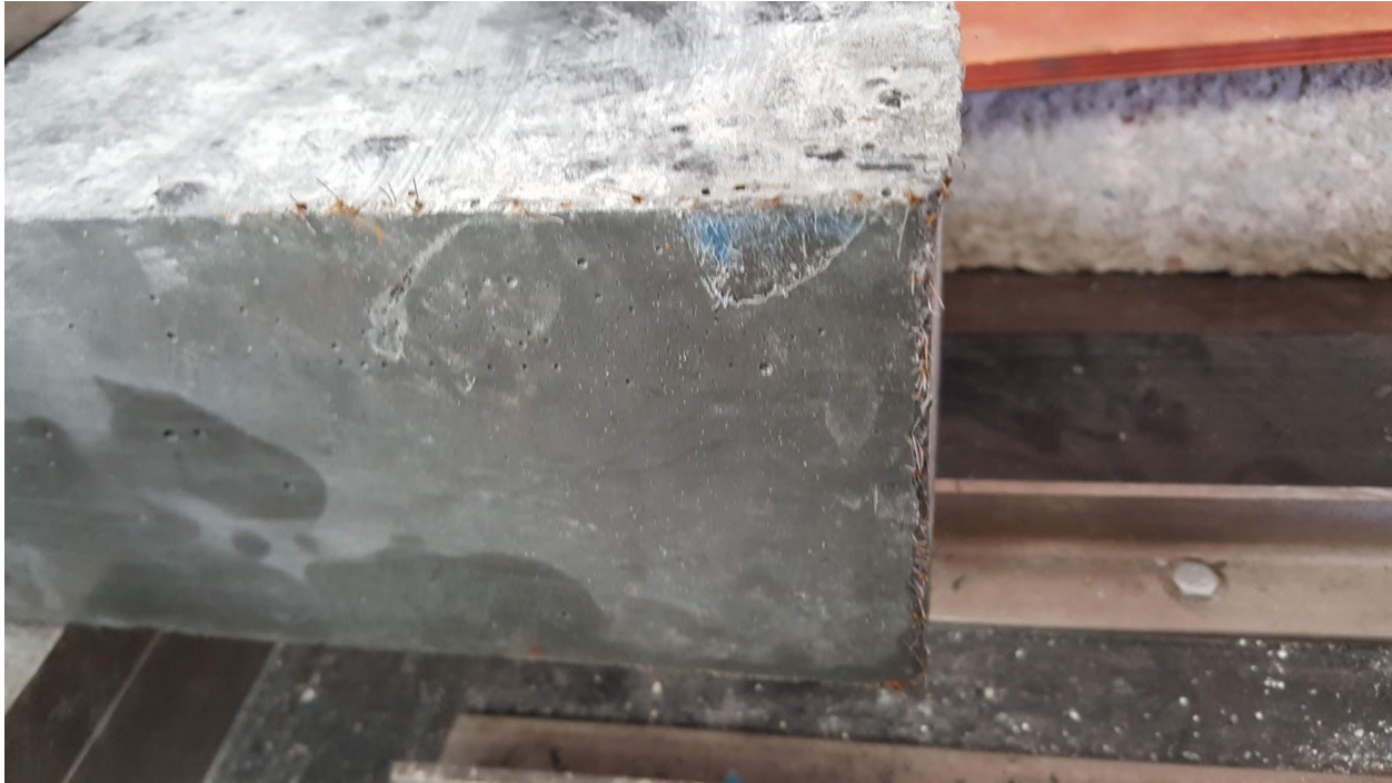
Figure 75: Freeze-thaw first sign of rust on 2% specimen after 9 cycles (07/08)
