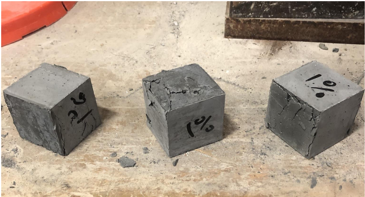
Figure 121: OU J3 1% cube 3 day compressive strength test specimens after failure
