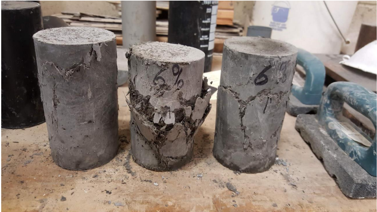
Figure 37: OU J3 6% cylinder 3 day compressive strength test specimens after failure
