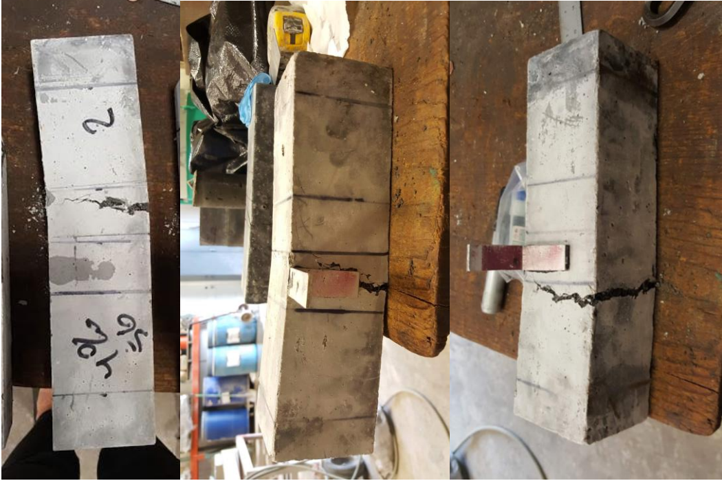
Figure 60: OU J3 4% 56 day MOR test specimens after failure
