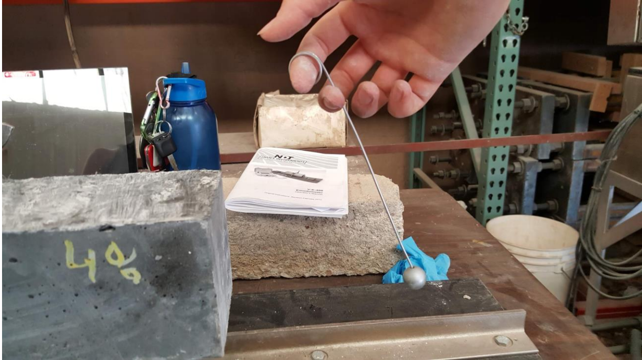
Figure 12: Metal ball and distance of hit used to determine resonant frequency for the freeze-thaw tests
