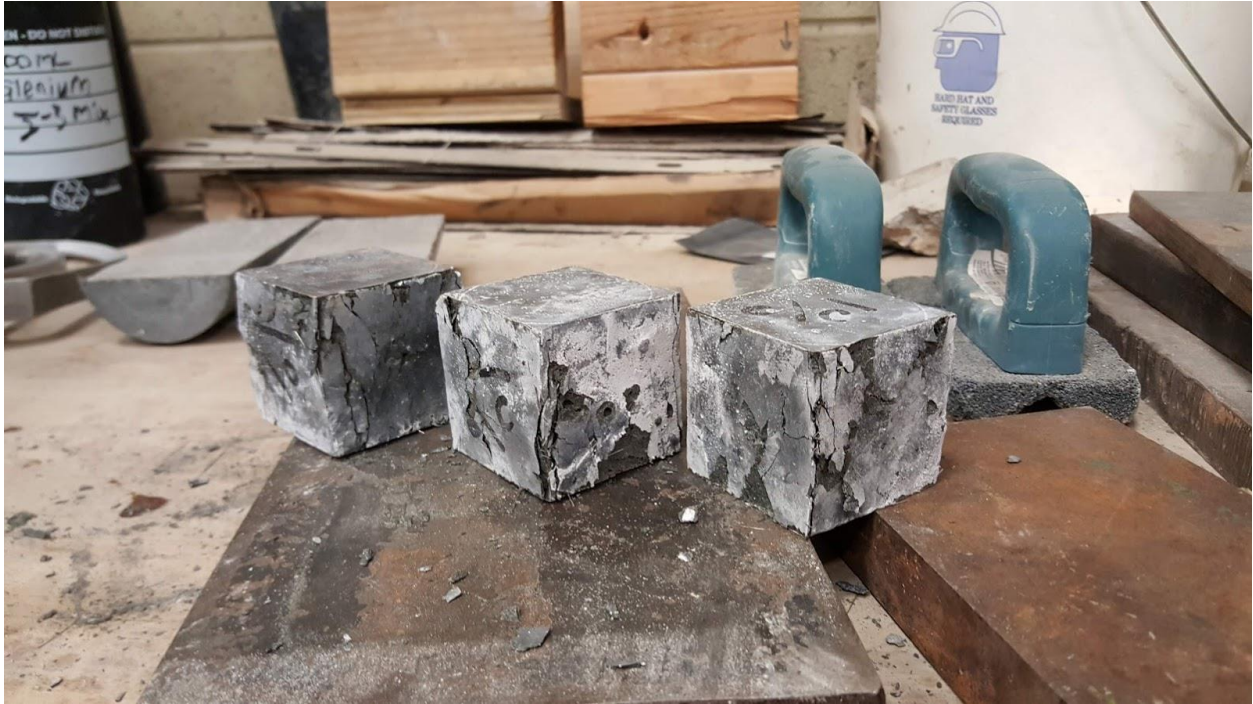
Figure 28: OU J3 1% cube 56 day compressive strength test specimens after failure
