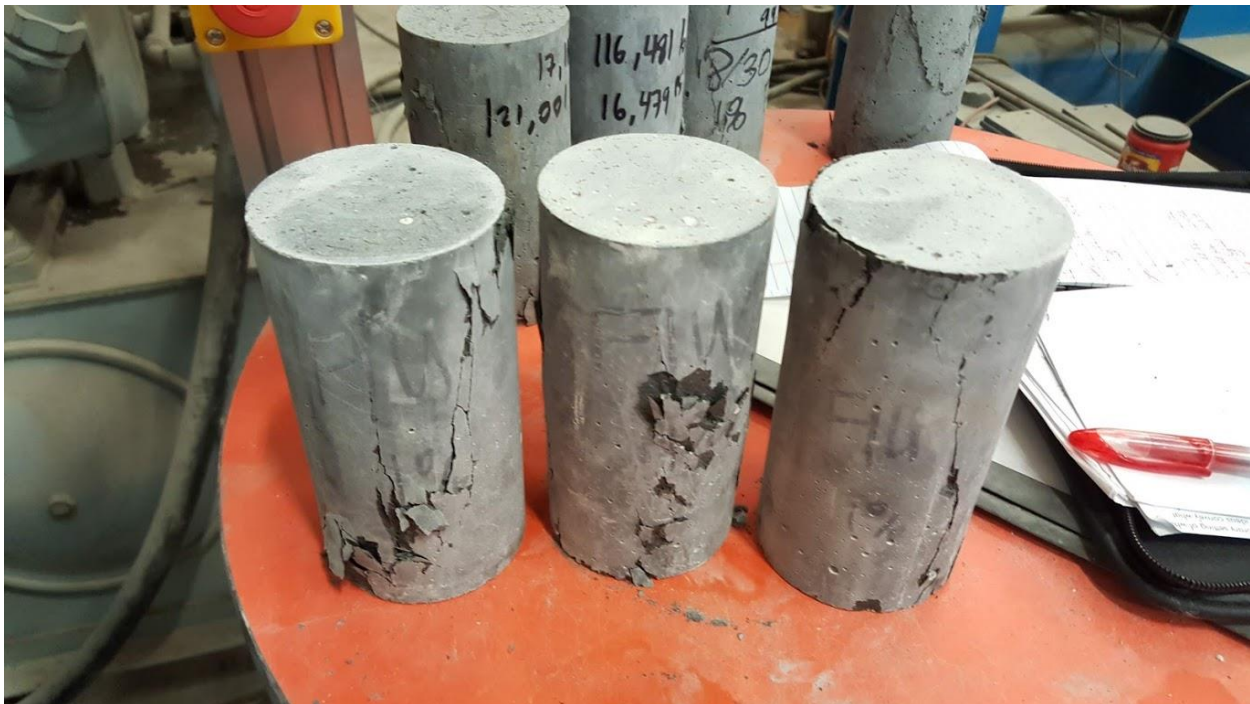
Figure 89: FIU J3 1% cylinder 28 day compressive strength test specimens after failure
