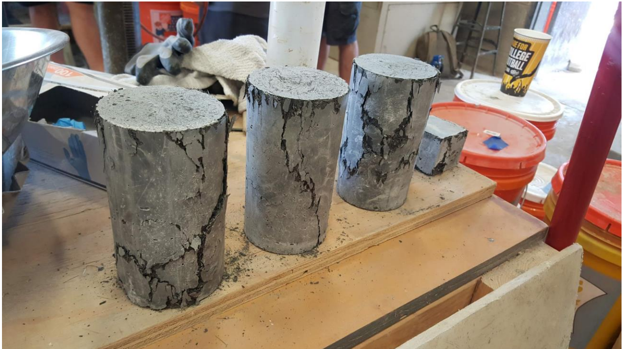
Figure 39: OU J3 6% cylinder 56 day compressive strength test specimens after failure
