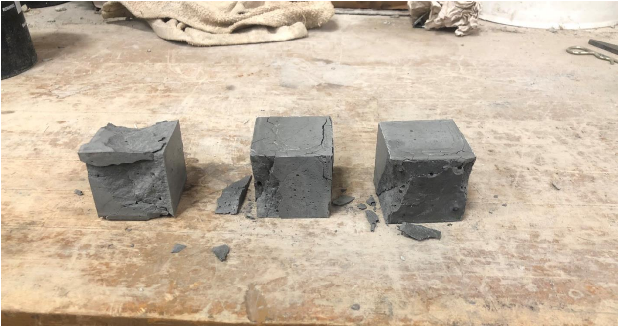
Figure 116: OU J3 0% cube 3 day compressive strength test specimens after failure
