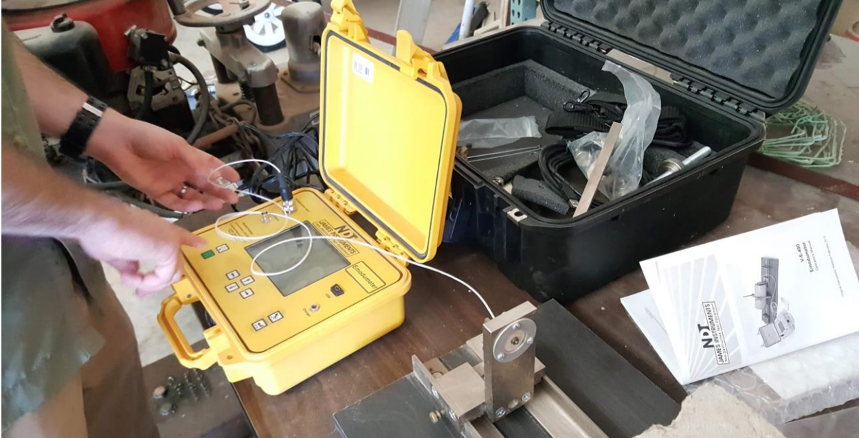
Figure 10: James Instruments E-Meter device used to record resonant frequency data during the freeze-thaw test
