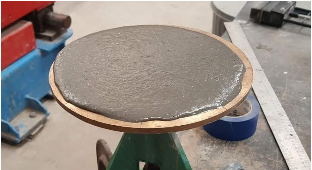
Figure 15: OU J3 1% fiber mix flow test
