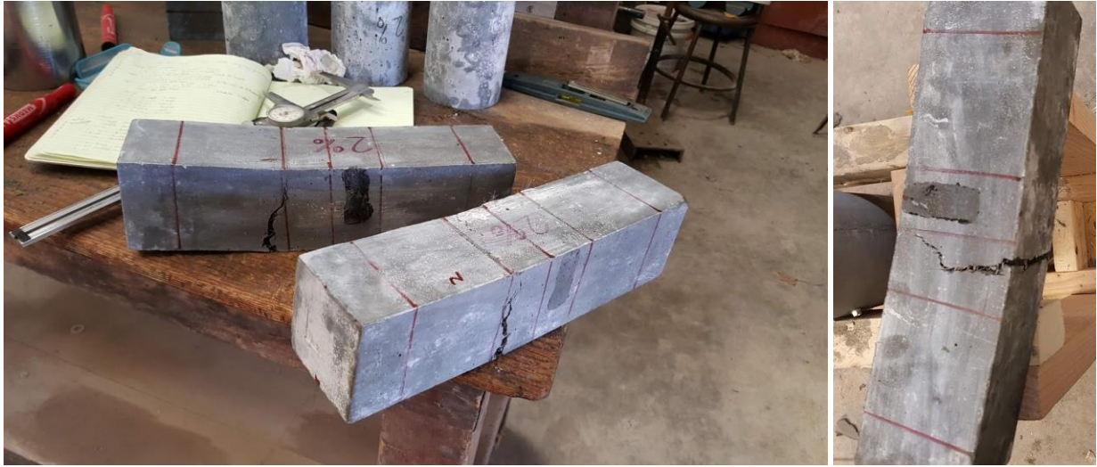
Figure 54: OU J3 2% 28 day MOR test specimens after failure
