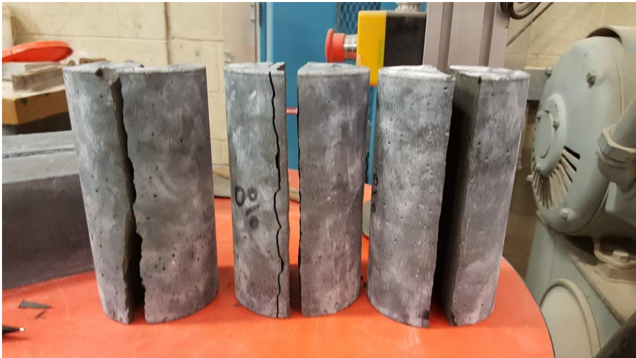
Figure 45: OU J3 0% 28 day splitting tensile test specimens after failure
