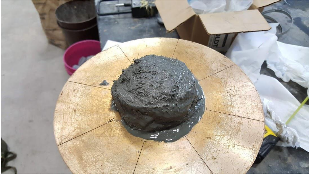
Figure 18: OU J3 6% fiber mix flow test
