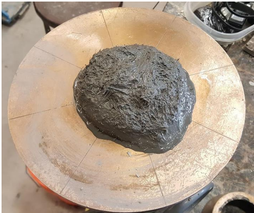
Figure 81: FIU J3 6% fiber mix flow test
