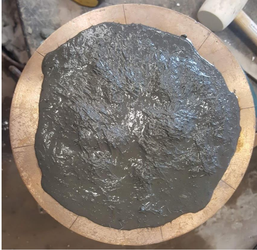
Figure 80: FIU J3 4% fiber mix flow test
