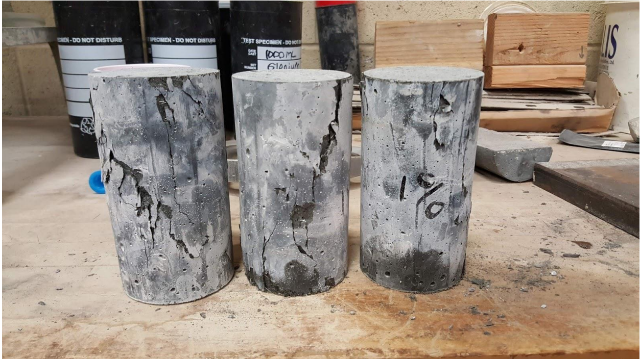
Figure 120: OU J3 1% cylinder 56 day compressive strength test specimens after failure
