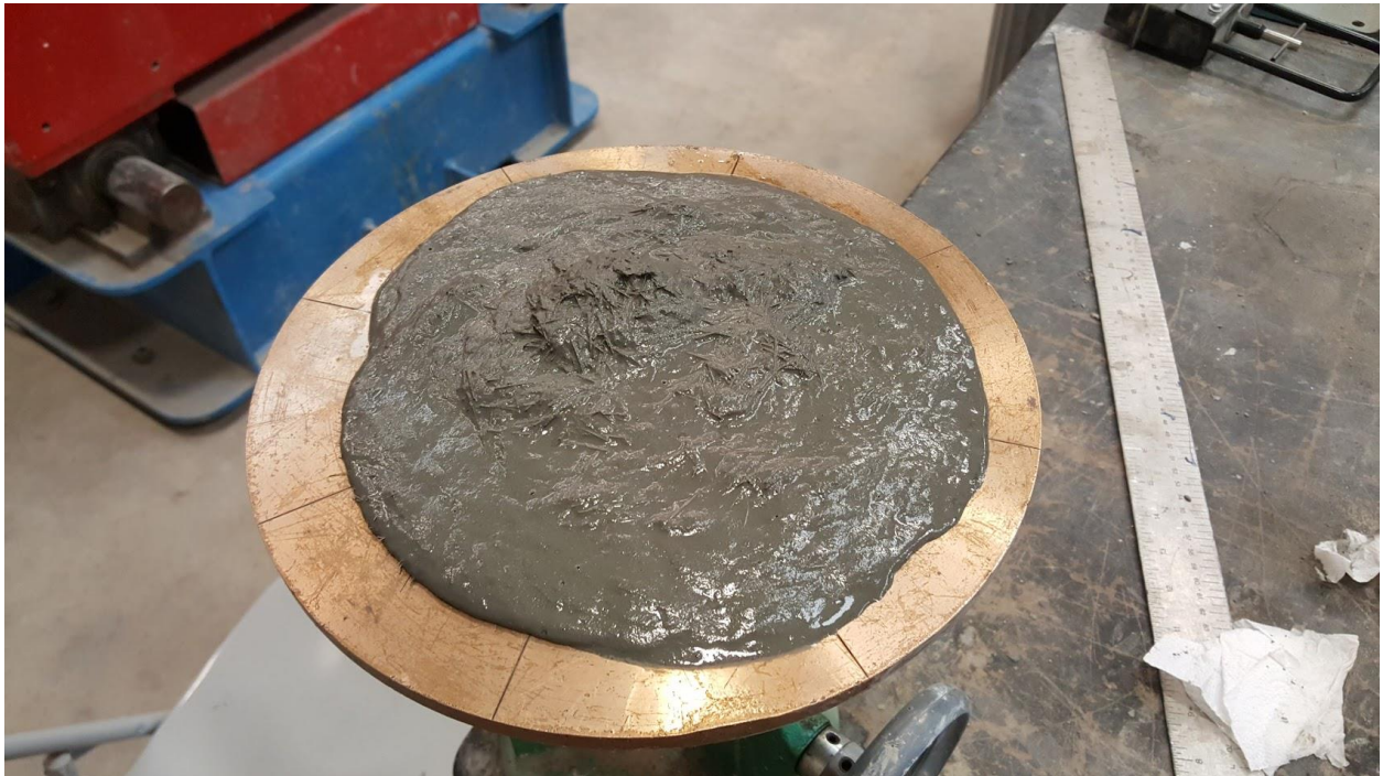
Figure 17: OU J3 4% fiber mix flow test
