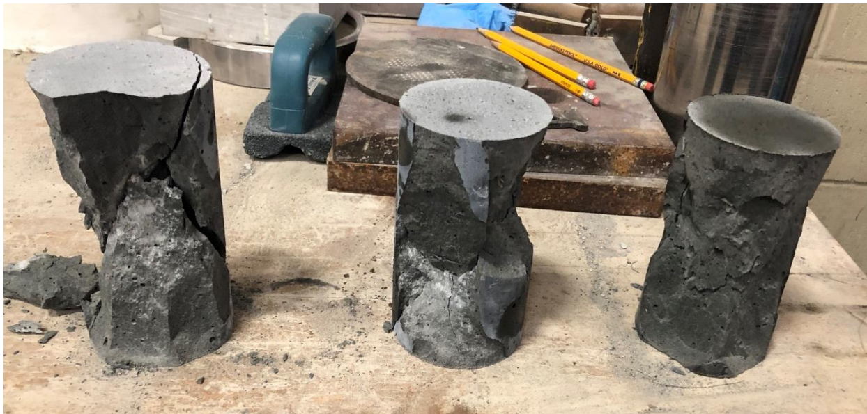
Figure 23: OU J3 0% cylinder 7 day compressive strength test specimens after failure
