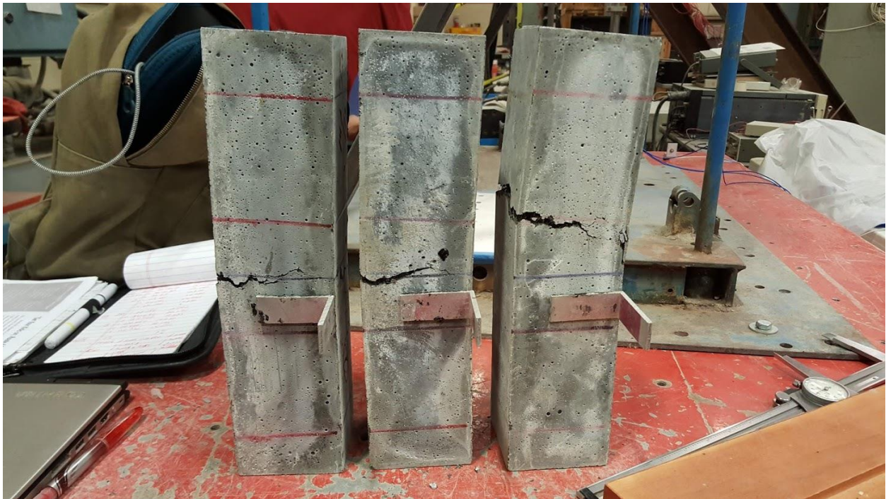
Figure 108: FIU J3 4% 56 day MOR test specimens after failure
