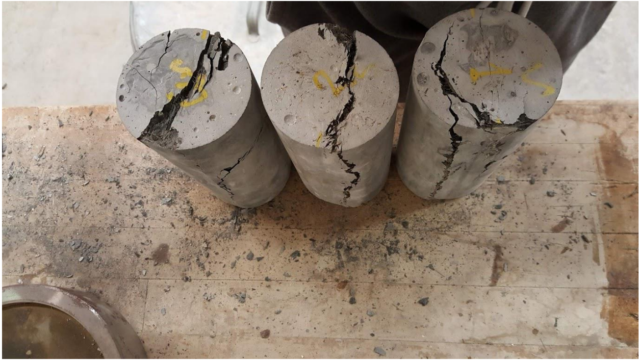
Figure 49: OU J3 6% 28 day splitting tensile test specimens after failure
