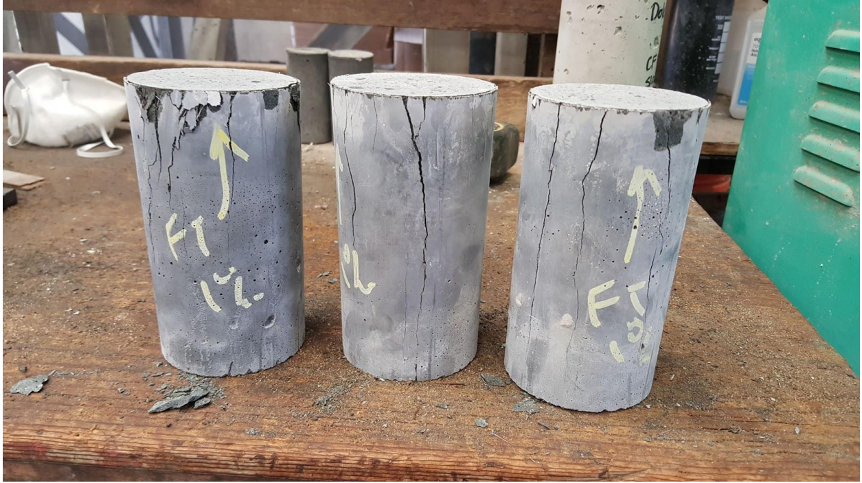
Figure 65: Freeze-thaw 1% 28 day cylinder compressive strength test specimens after failure
