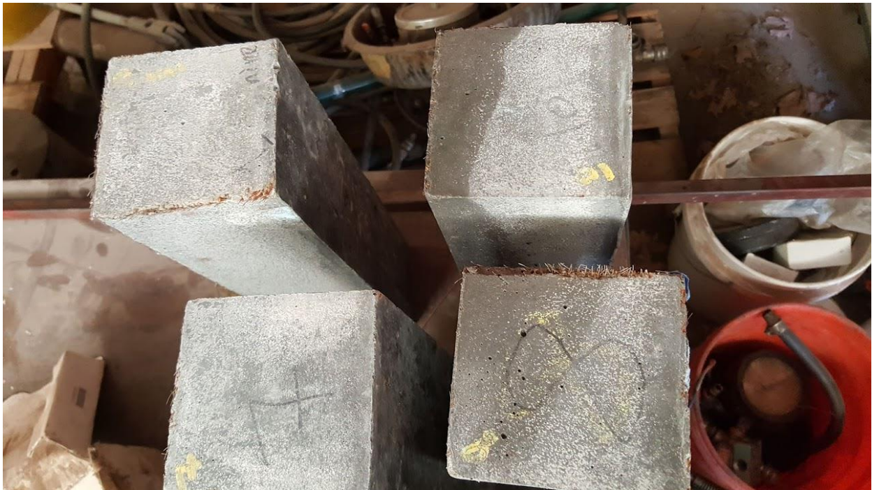
Figure 74: Freeze-thaw specimens after 351 cycles (11/03 final day) showing rusted exposed fibers
