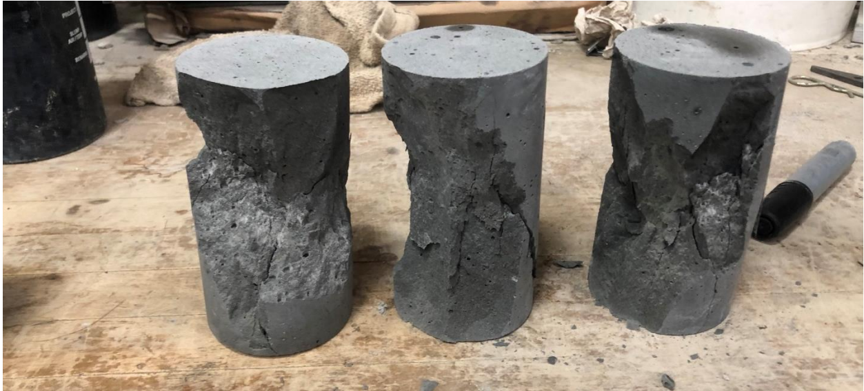
Figure 22: OU J3 0% cylinder 3 day compressive strength test specimens after failure
