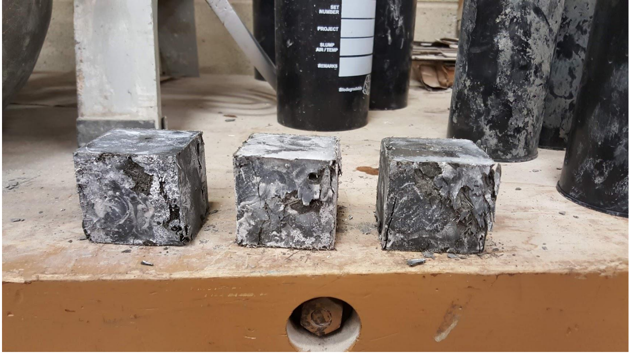
Figure 36: OU J3 4% cube 56 day compressive strength test specimens after failure
