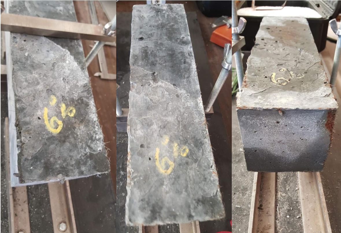
Figure 76: Freeze-thaw 6% specimens after 0 (7/01) (left), 42 (7/15) (middle), and 351 cycles (11/03) (right)
