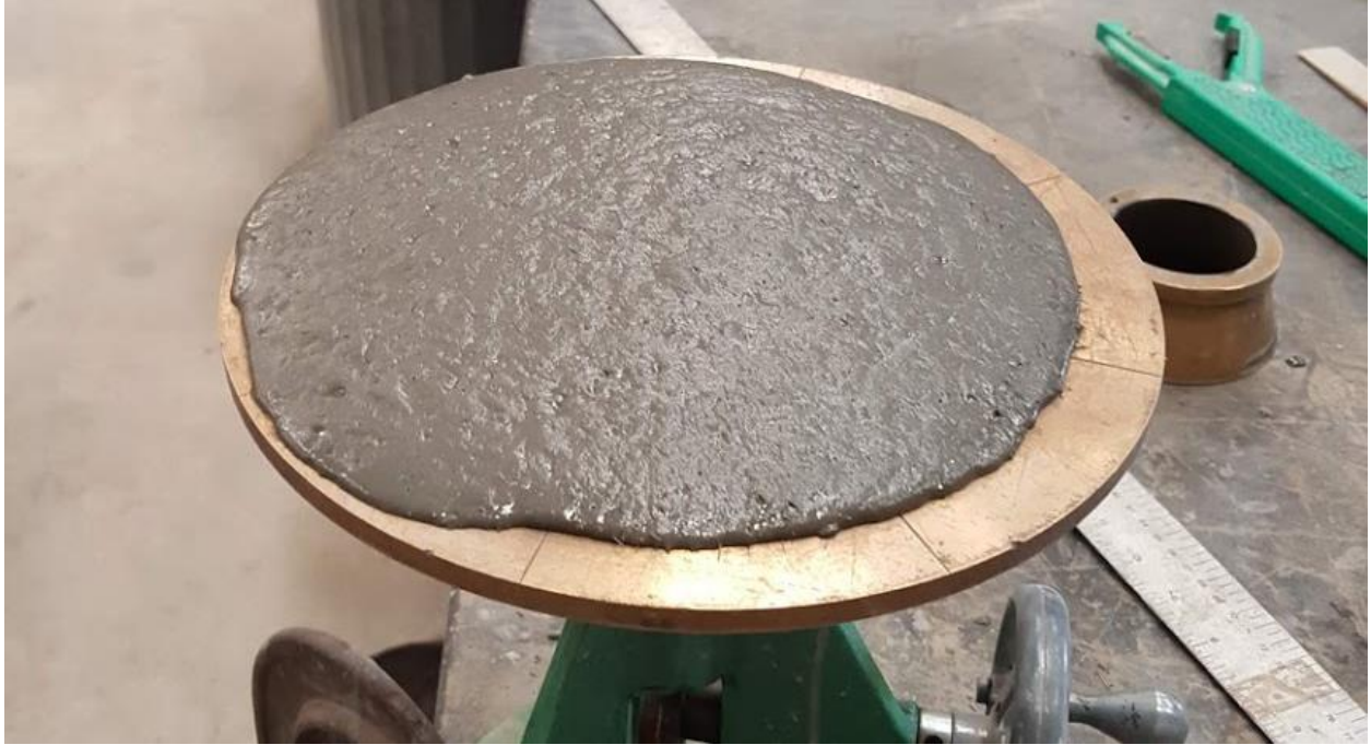
Figure 16: OU J3 2% fiber mix flow test
