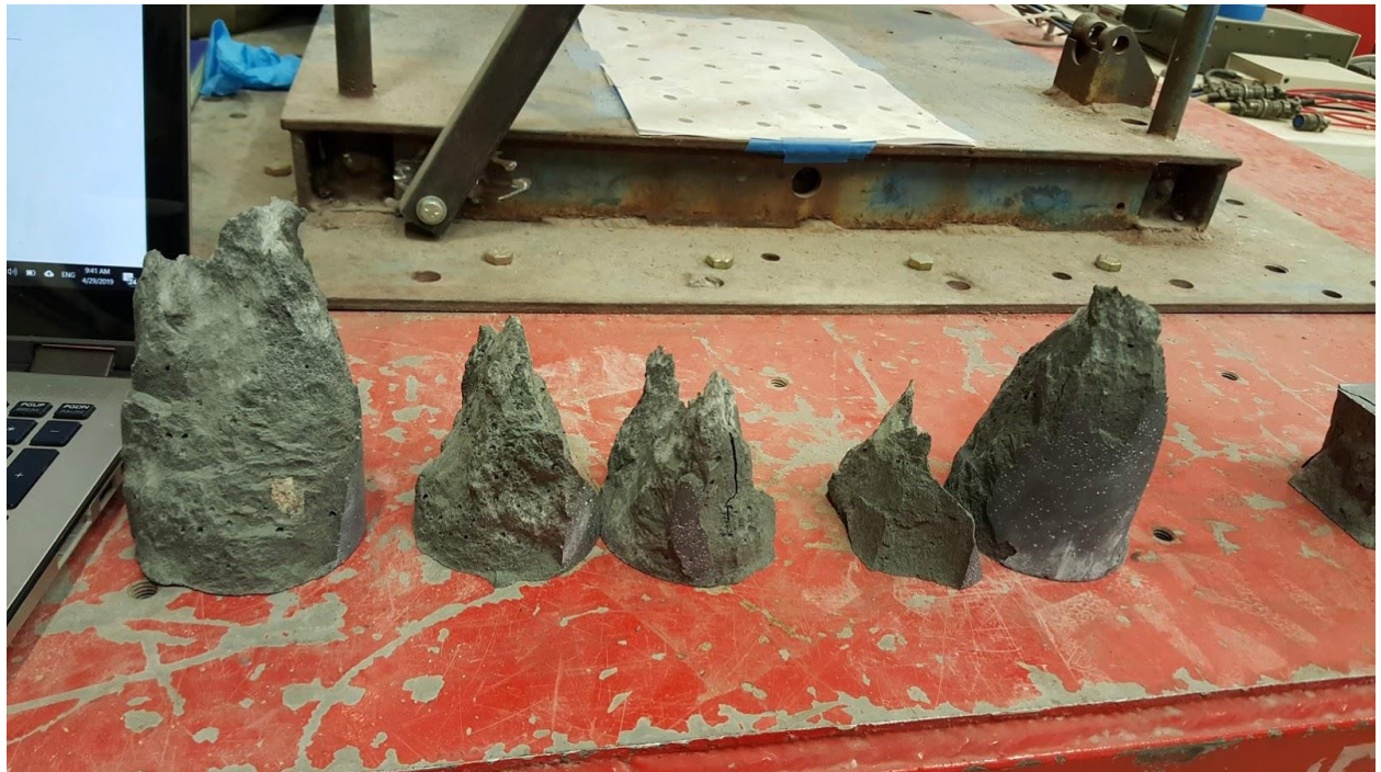
Figure 25: OU J3 0% cylinder 56 day compressive strength test specimens after failure
