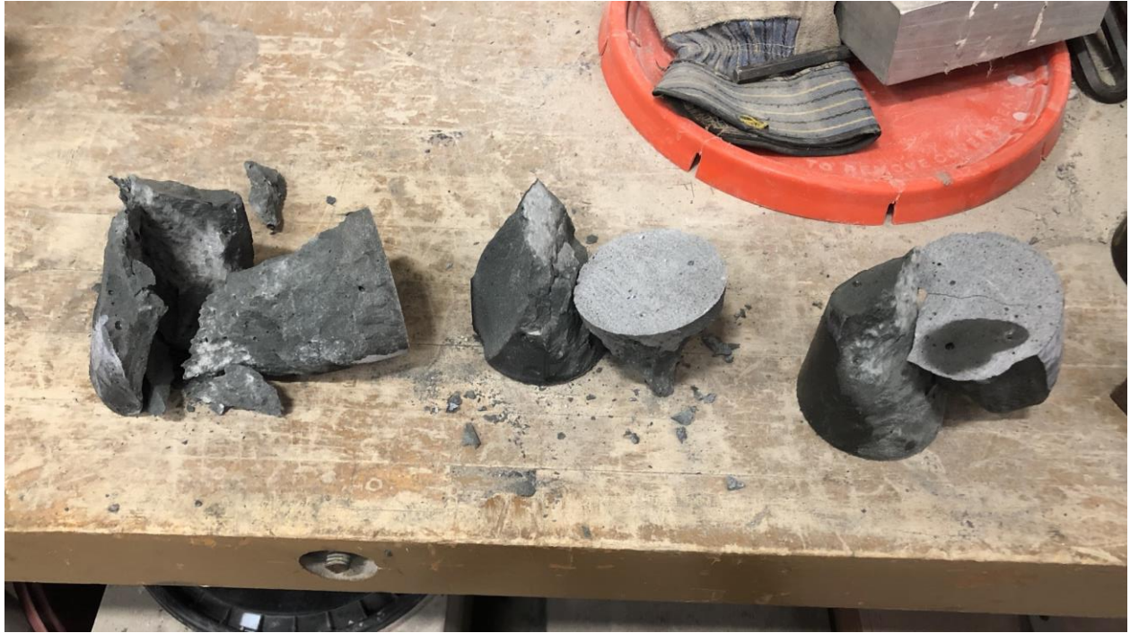
Figure 24: OU J3 0% cylinder 28 day compressive strength test specimens after failure
