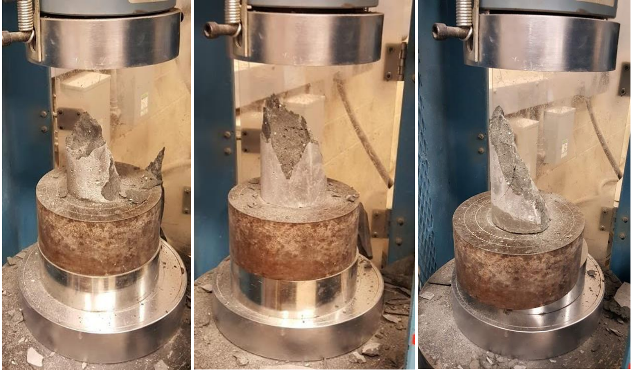
Figure 88: FIU J3 0% cylinder 28 day compressive strength test specimens after failure
