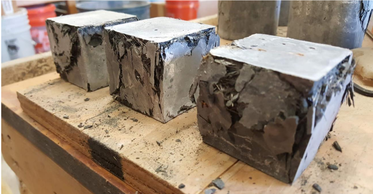
Figure 42: OU J3 6% cube 56 day compressive strength test specimens after failure
