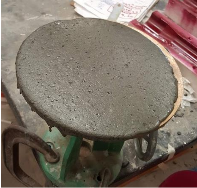
Figure 78: FIU J3 0% fiber mix flow test
