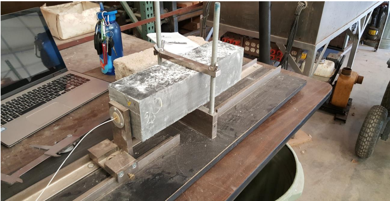
Figure 11: Freeze-thaw test specimen set up set up to measure resonant frequency
