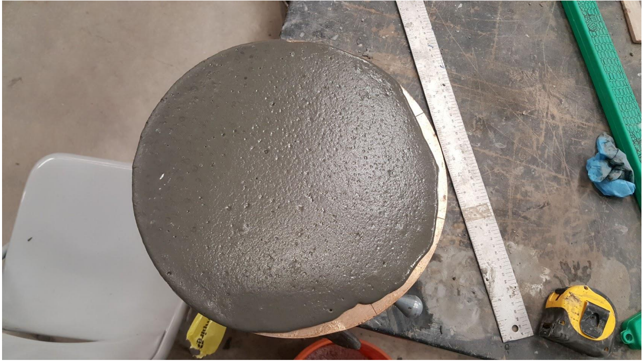
Figure 14: OU J3 0% fiber mix flow test
