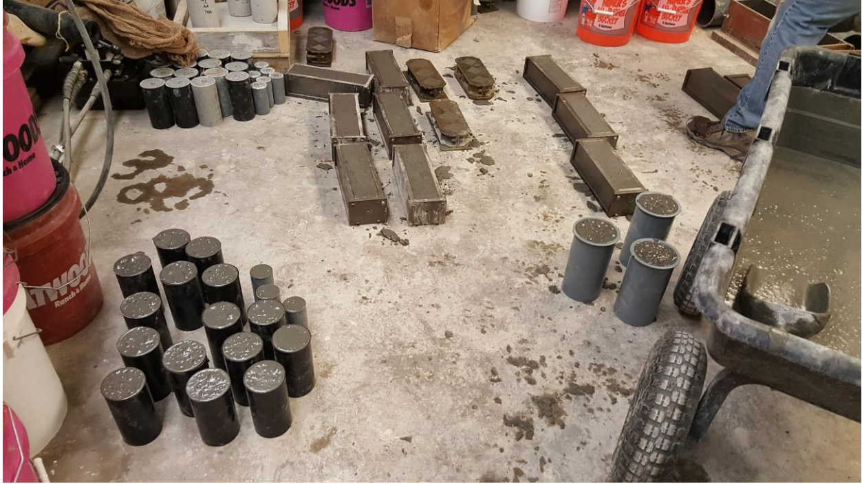
Figure 3: Batch of J3 specimens immediately after casting
