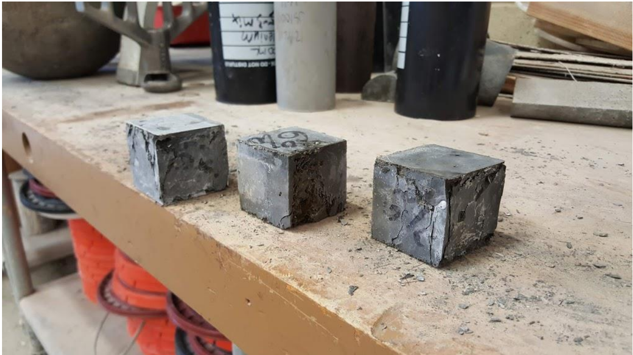
Figure 41: OU J3 6% cube 28 day compressive strength test specimens after failure
