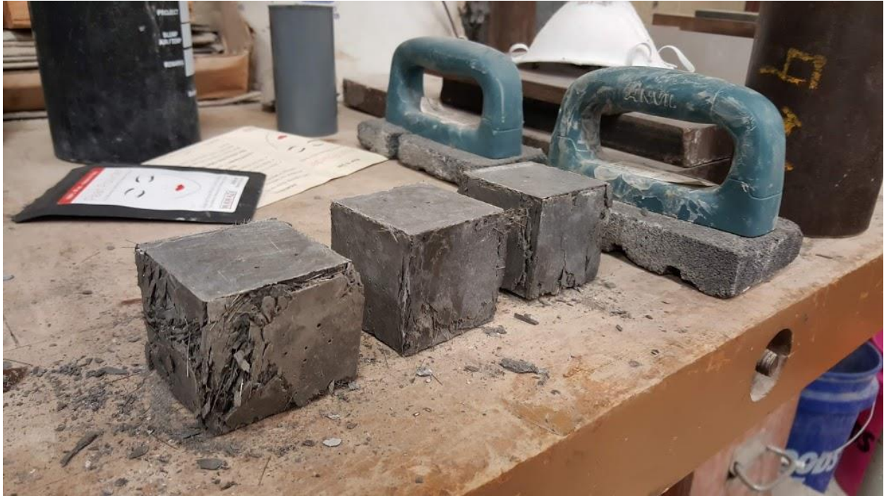
Figure 40: OU J3 6% cube 3 day compressive strength test specimens after failure
