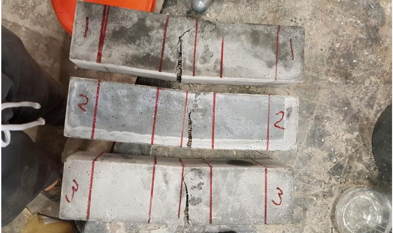
Figure 101: FIU J3 1% 28 day MOR test specimens after failure
