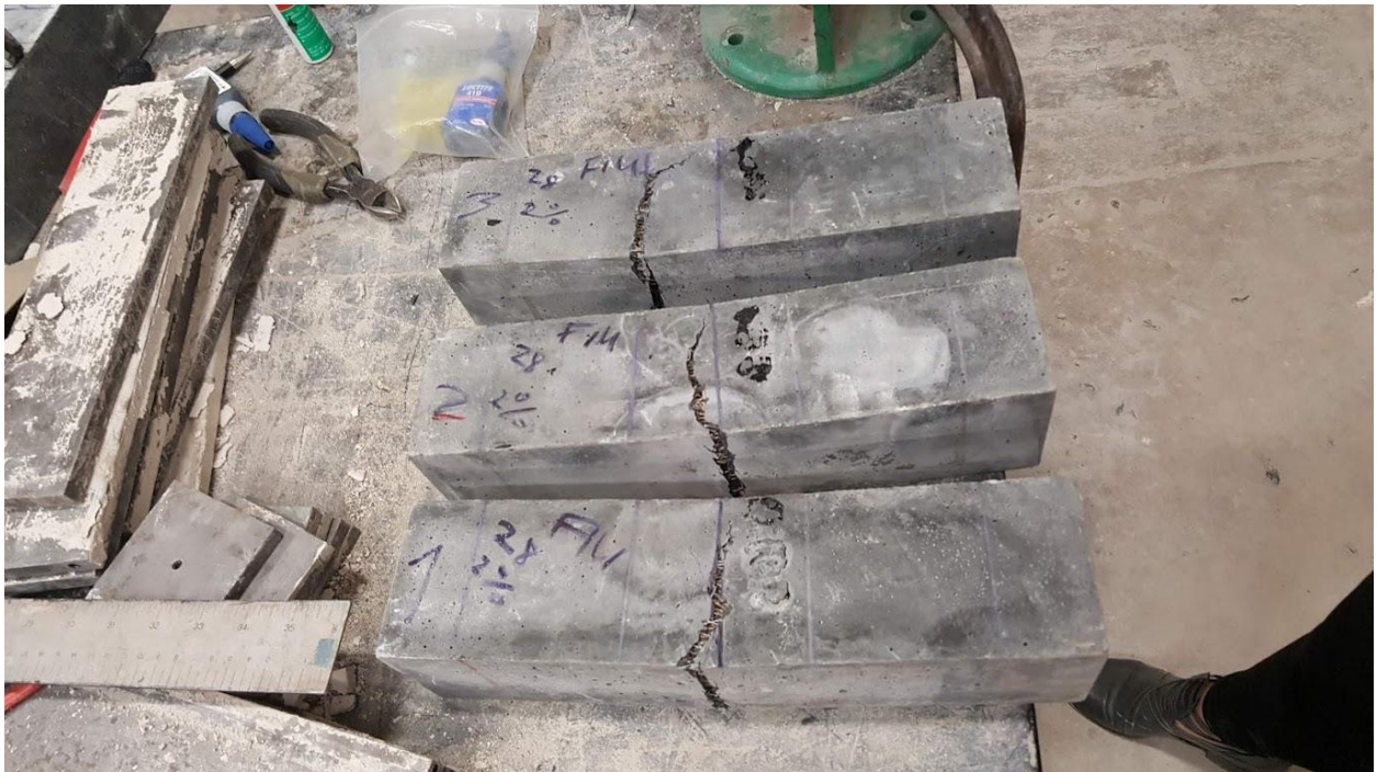
Figure 102: FIU J3 2% 28 day MOR test specimens after failure
