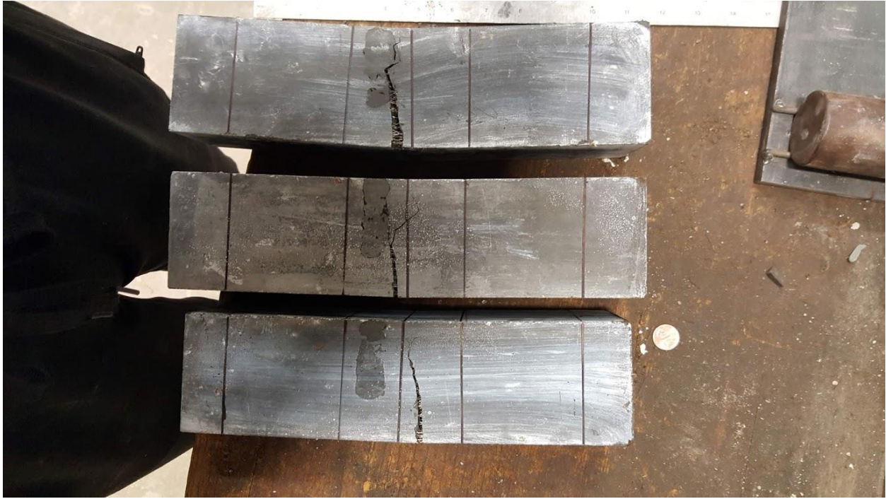
Figure 58: OU J3 1% 56 day MOR test specimens after failure
