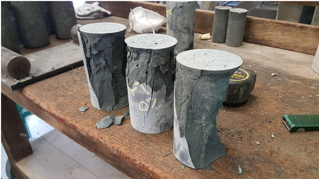
Figure 64: Freeze-thaw 0% 28 day cylinder compressive strength test specimens after failure
