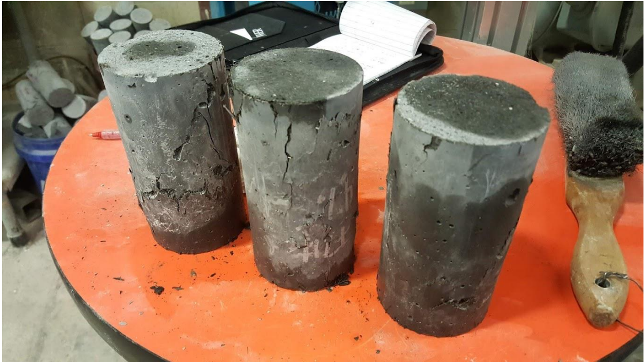
Figure 91: FIU J3 4% cylinder 28 day compressive strength test specimens after failure
