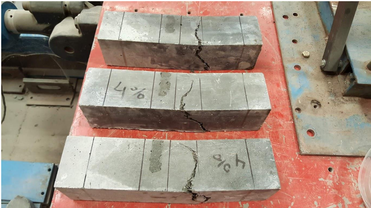
Figure 55: OU J3 4% 28 day MOR test specimens after failure
