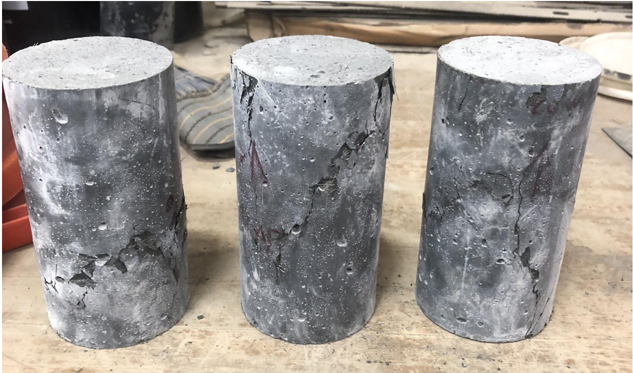
Figure 29: OU J3 2% cylinder 28 day compressive strength test specimens after failure
