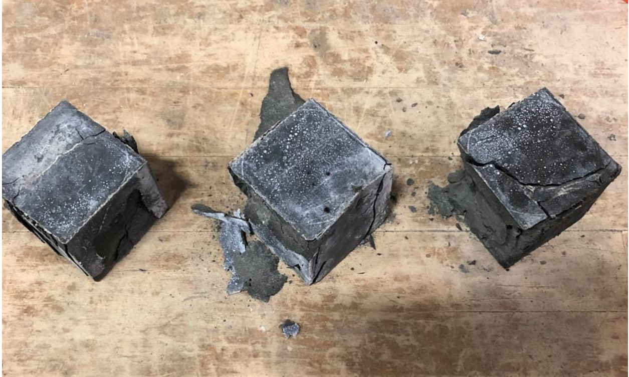
Figure 26: OU J3 0% cube 28 day compressive strength test specimens after failure
