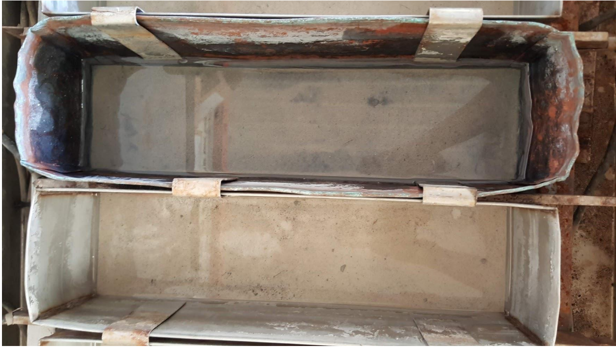
Figure 77: Freeze-thaw chamber trays after 351 cycles (11/03 final day)
