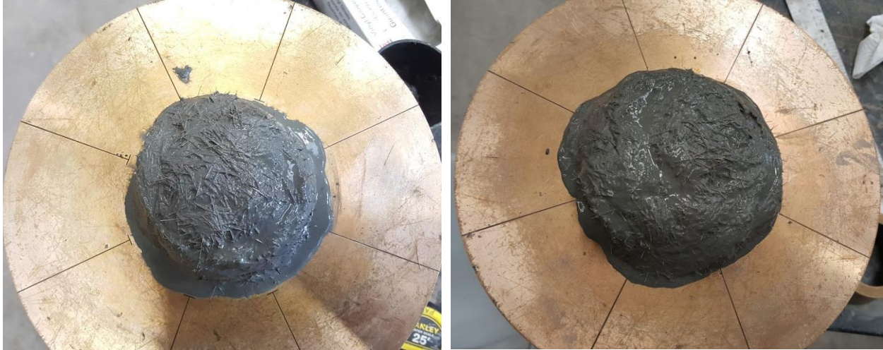
Figure 62:OU J3 (left) vs. freeze-thaw J3 (right) 6% fiber mix flow test
