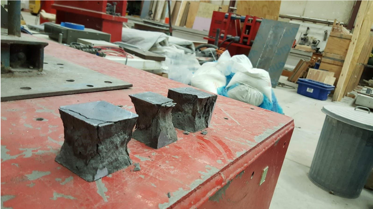
Figure 117: OU J3 0% cube 56 day compressive strength test specimens after failure
