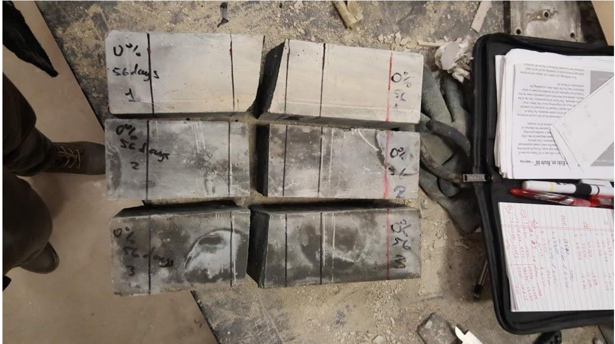
Figure 105: FIU J3 0% 56 day MOR test specimens after failure
