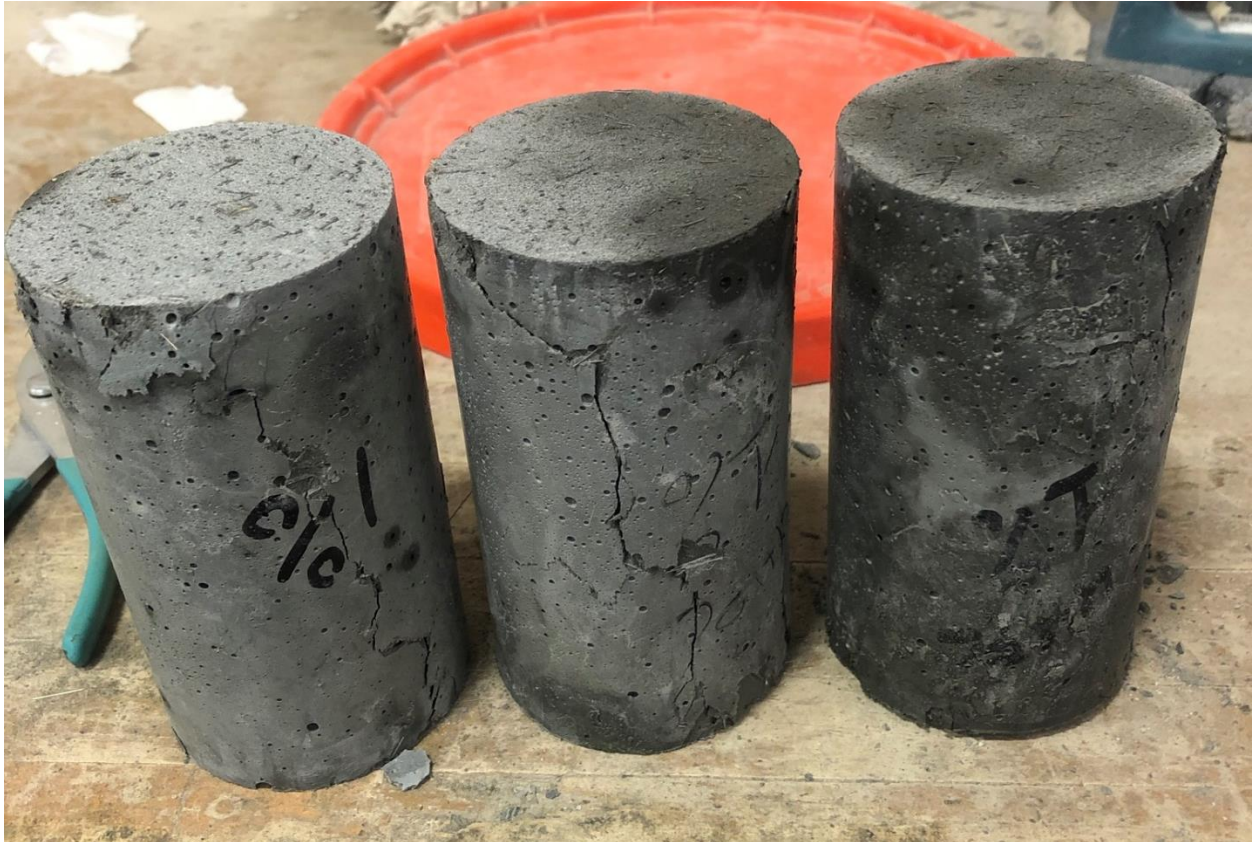
Figure 118: OU J3 1% cylinder 3 day compressive strength test specimens after failure
