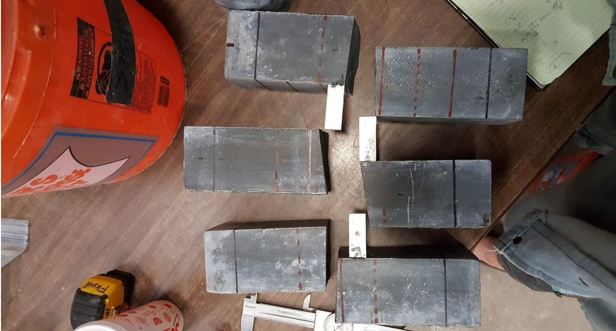
Figure 52: OU J3 0% 28 day MOR test specimens after failure
