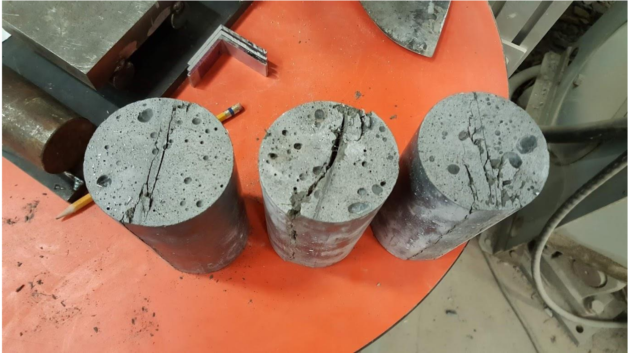
Figure 46: OU J3 1% 28 day splitting tensile test specimens after failure
