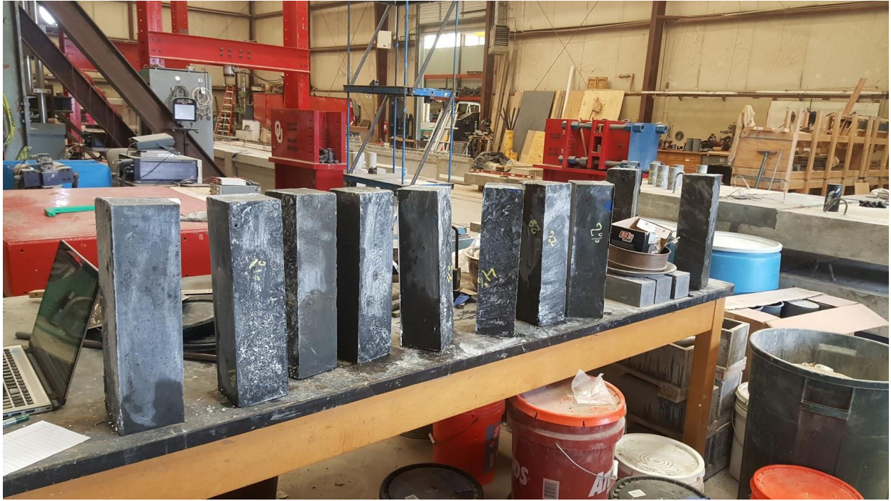
Figure 71: Freeze-thaw specimens after 0 cycles (07/01)
