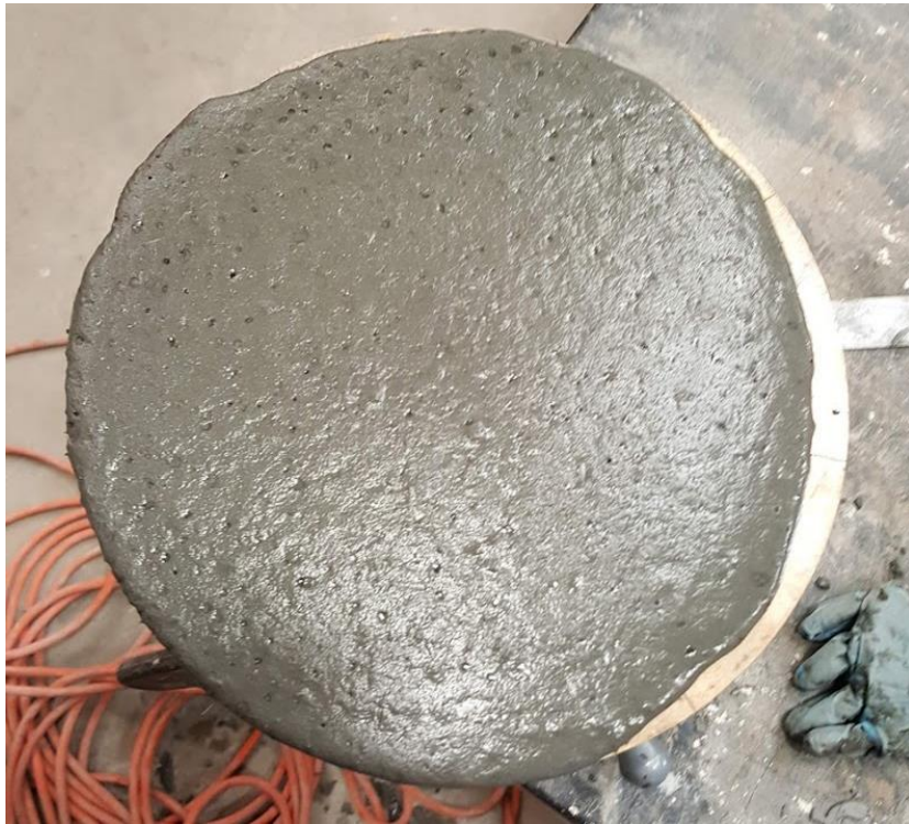
Figure 79: FIU J3 1% fiber mix flow test
