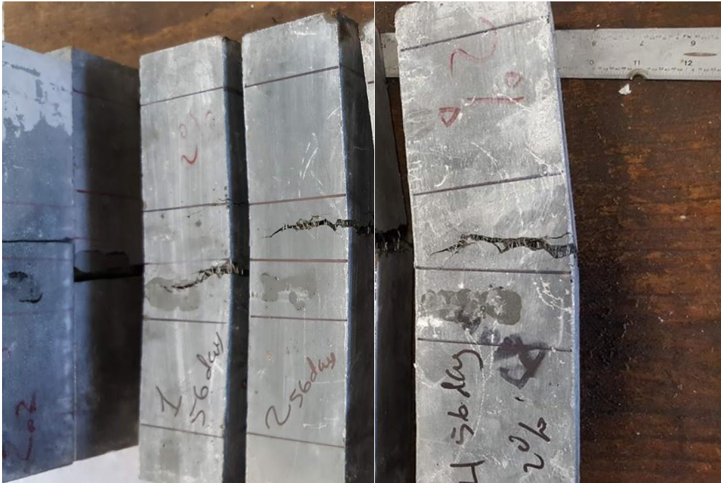
Figure 59: OU J3 2% 56 day MOR test specimens after failure
