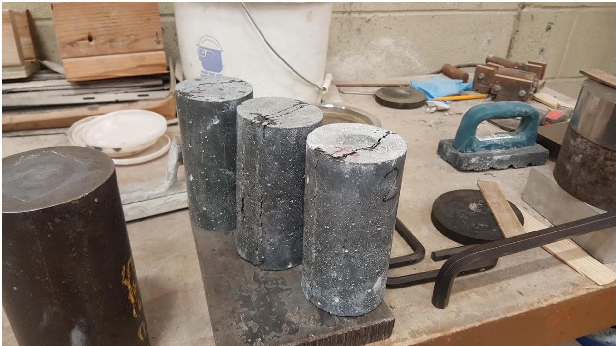
Figure 47: OU J3 2% 28 day splitting tensile test specimens after failure
