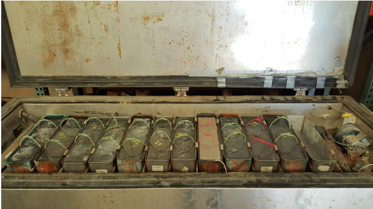
Figure 13: Freeze-thaw specimens in the freeze-thaw chamber
