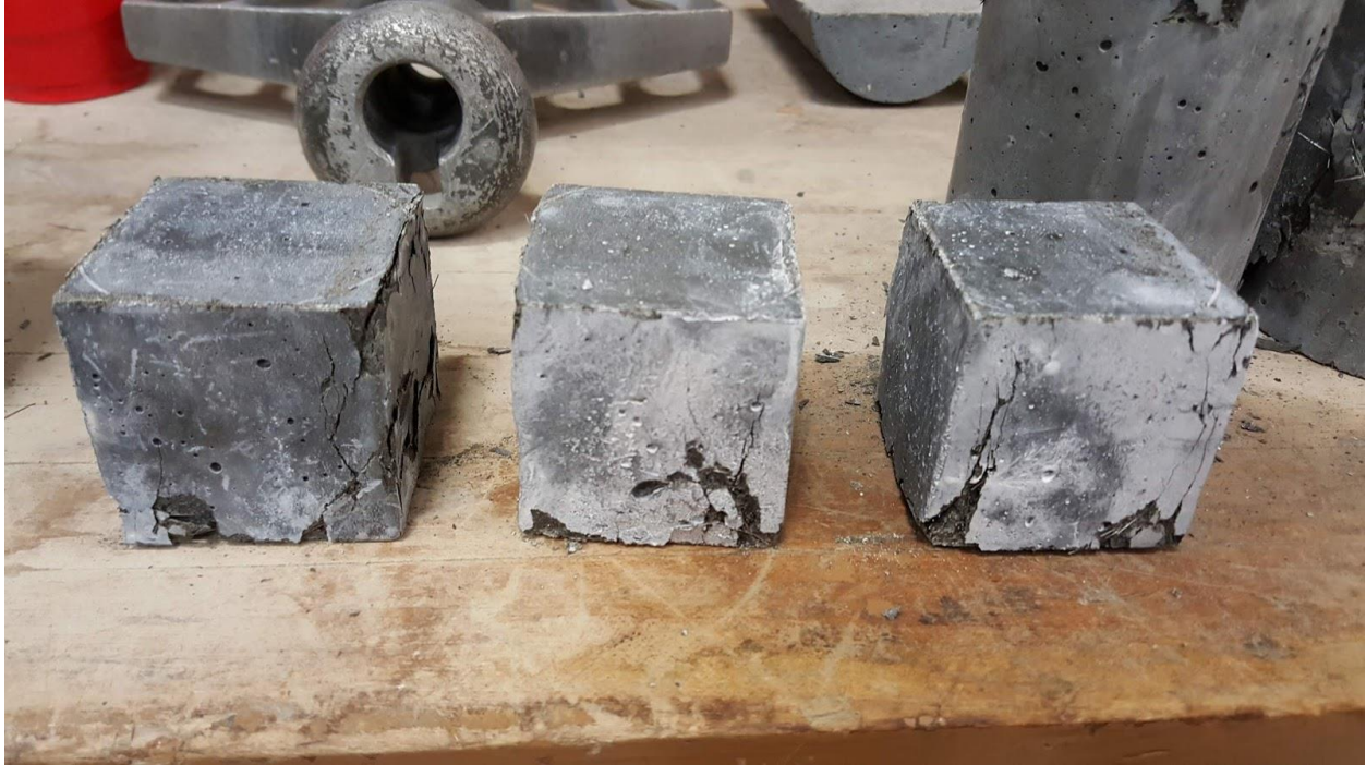
Figure 35: OU J3 4% cube 28 day compressive strength test specimens after failure
