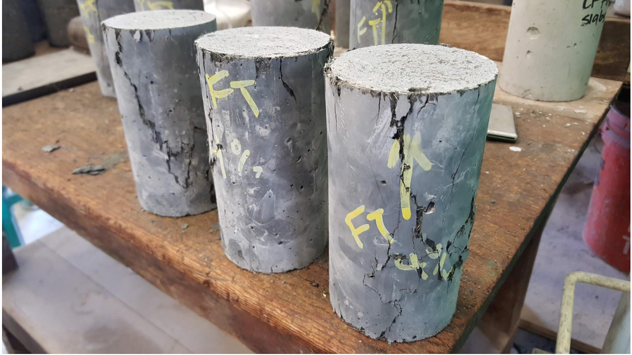
Figure 67: Freeze-thaw 4% 28 day cylinder compressive strength test specimens after failure
