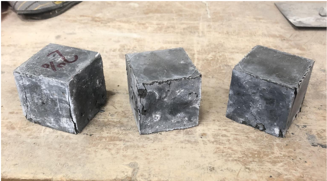
Figure 31: OU J3 2% cube 28 day compressive strength test specimens after failure
