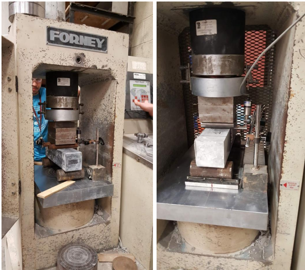
Figure 9: Standard MOR test set up
