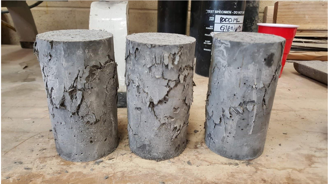
Figure 30: OU J3 2% cylinder 56 day compressive strength test specimens after failure
