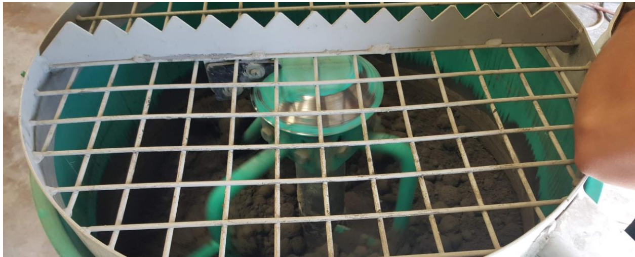
Figure 1: Smaller batch of UHPC in mixer
