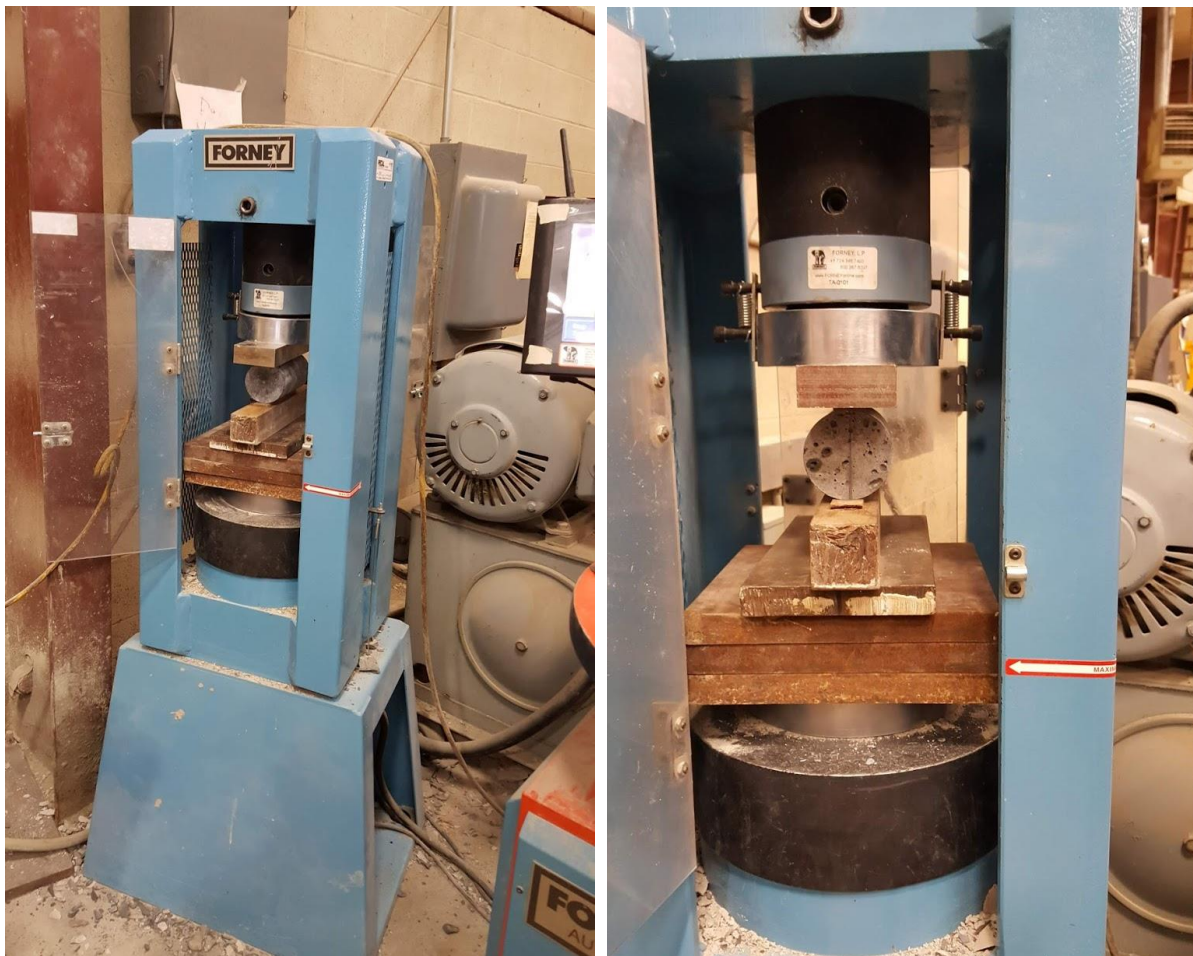
Figure 8: Standard splitting tensile strength test set up
