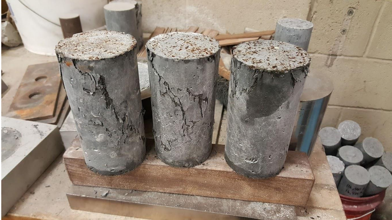
Figure 92: FIU J3 6% cylinder 28 day compressive strength test specimens after failure
