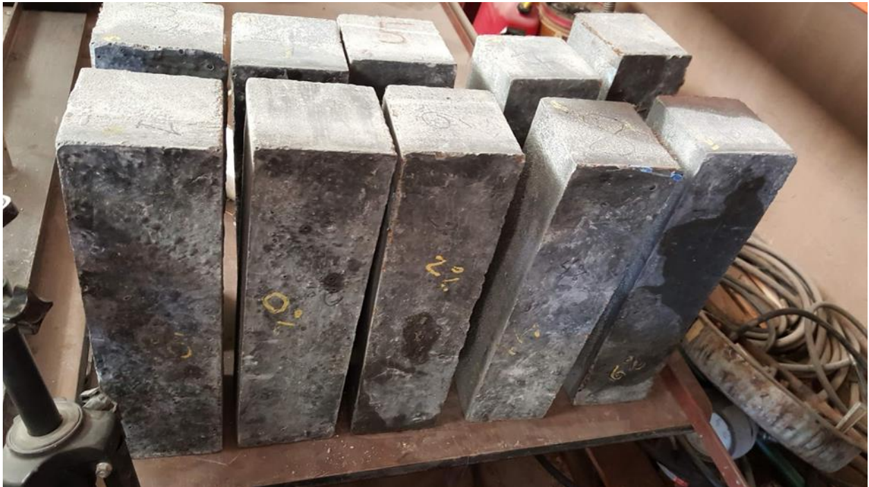
Figure 72: Freeze-thaw specimens after 351 cycles (11/03 final day)
