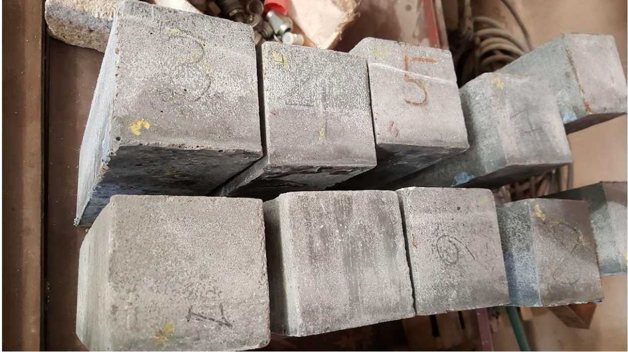
Figure 73: Close up view of freeze-thaw specimen ends after 351 cycles (11/03 final day)
