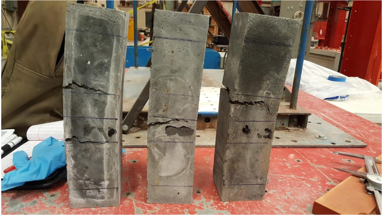
Figure 107: FIU J3 2% 56 day MOR test specimens after failure
