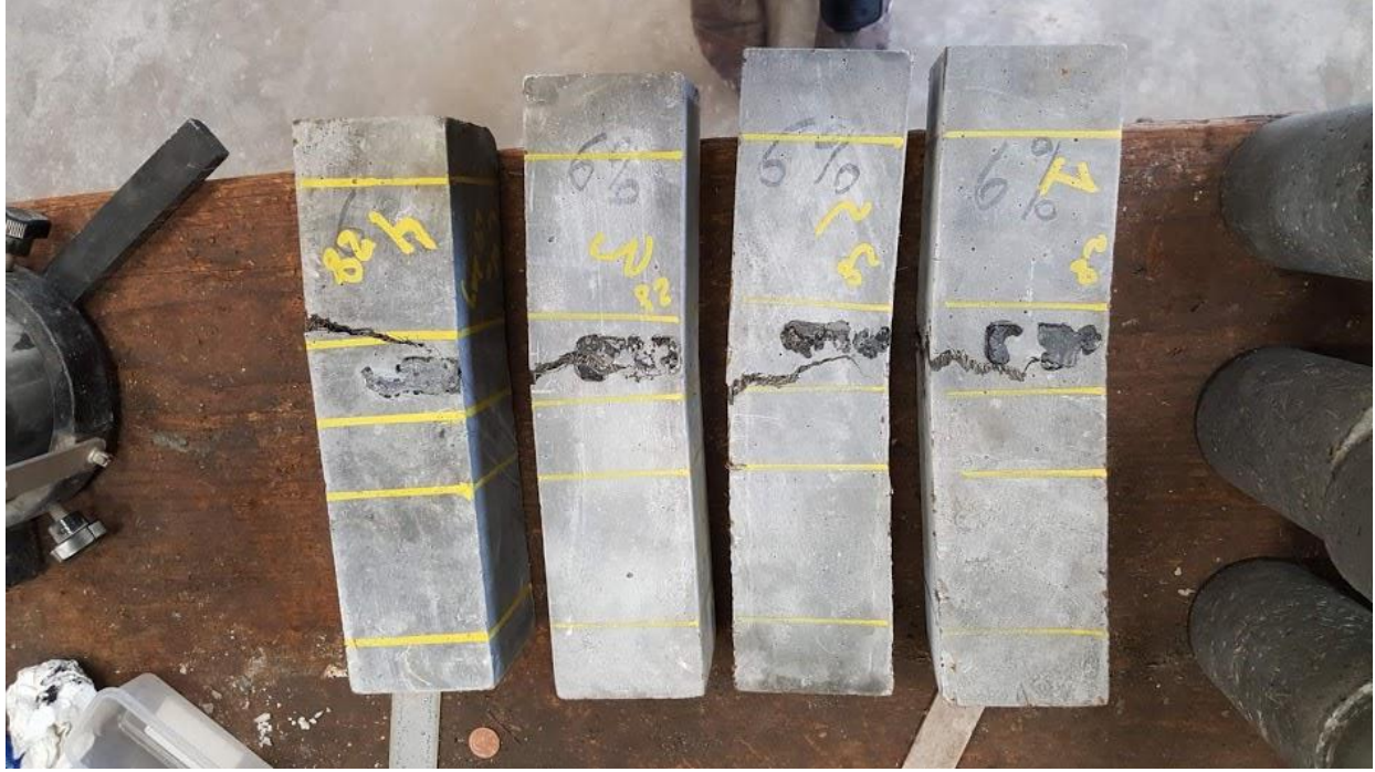
Figure 56: OU J3 6% 28 day MOR test specimens after failure
