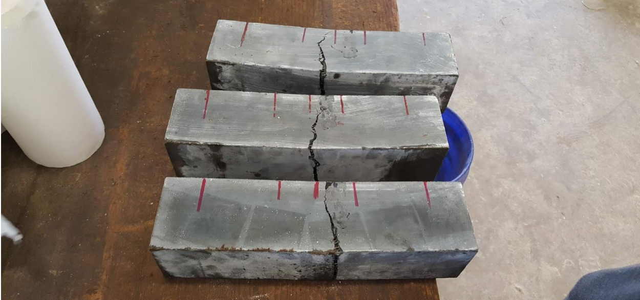
Figure 53: OU J3 1% 28 day MOR test specimens after failure
