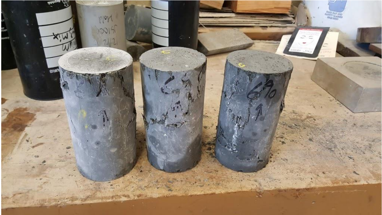
Figure 38: OU J3 6% cylinder 28 day compressive strength test specimens after failure
