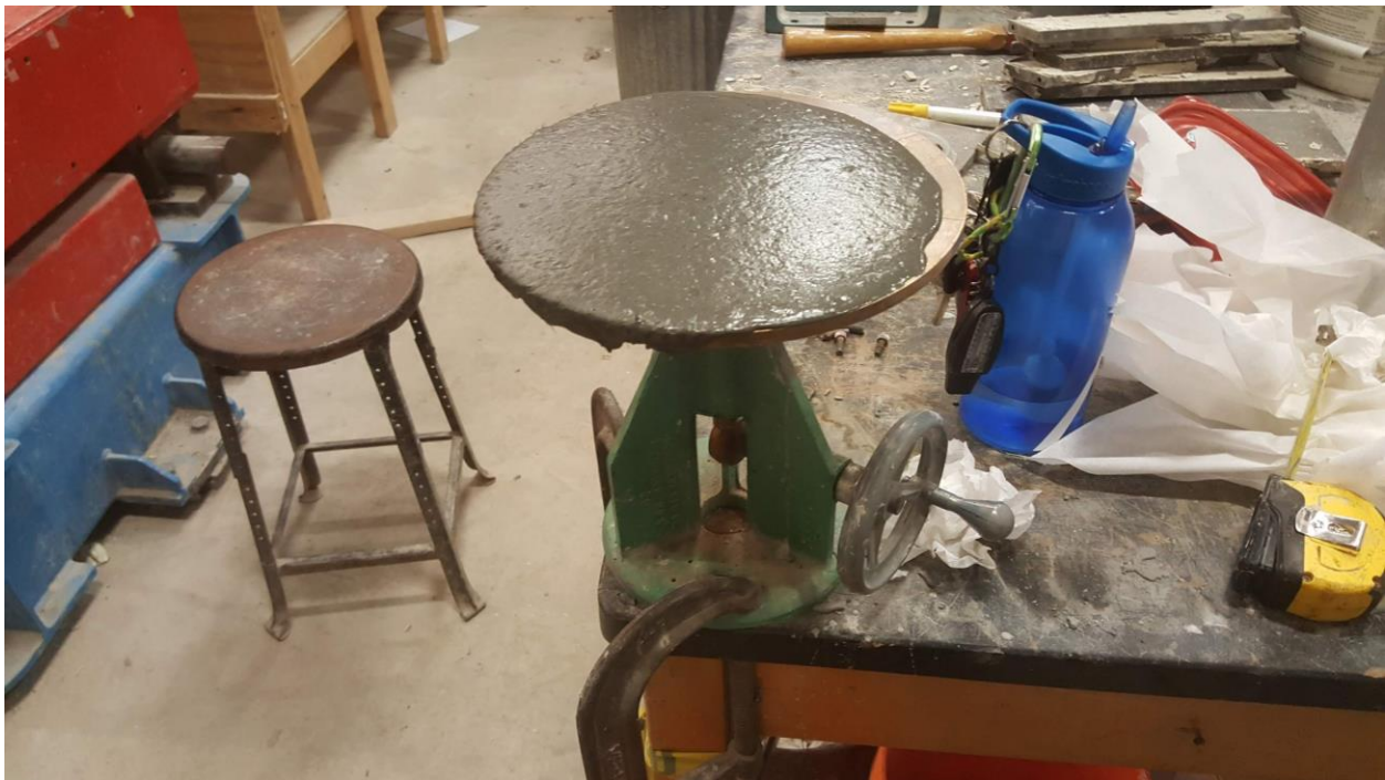
Figure 5: Standard flow test set up
