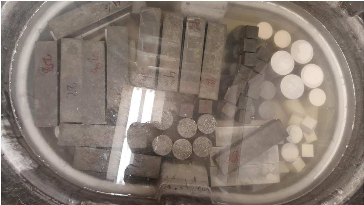
Figure 4: Specimens curing in tank
