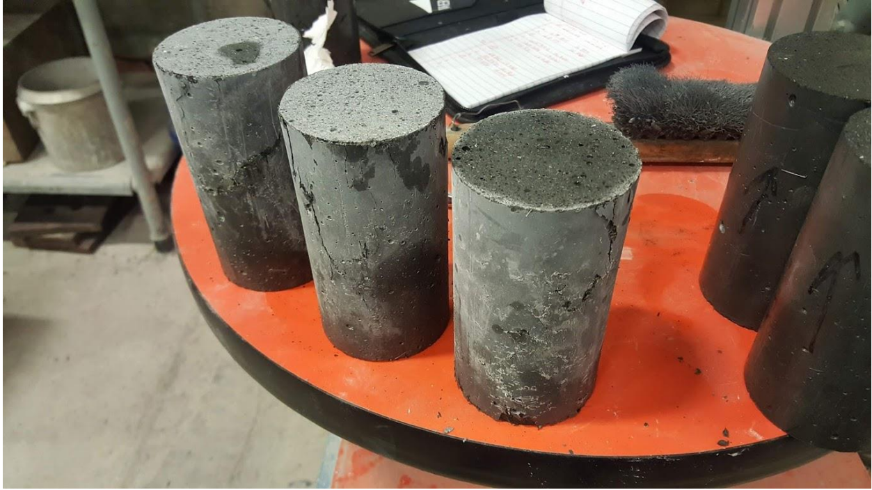
Figure 90: FIU J3 2% cylinder 28 day compressive strength test specimens after failure
