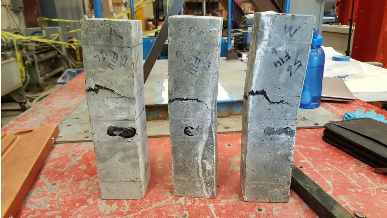
Figure 109: FIU J3 6% 56 day MOR test specimens after failure
