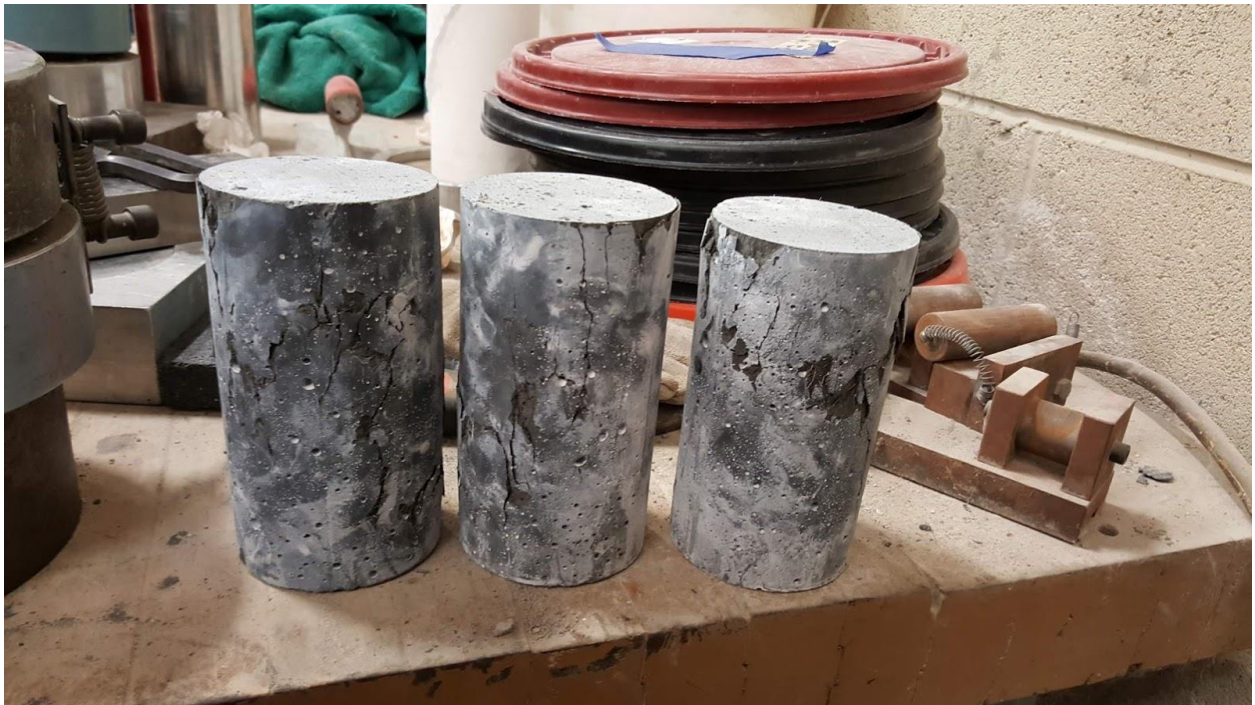
Figure 27: OU J3 1% cylinder 28 day compressive strength test specimens after failure
