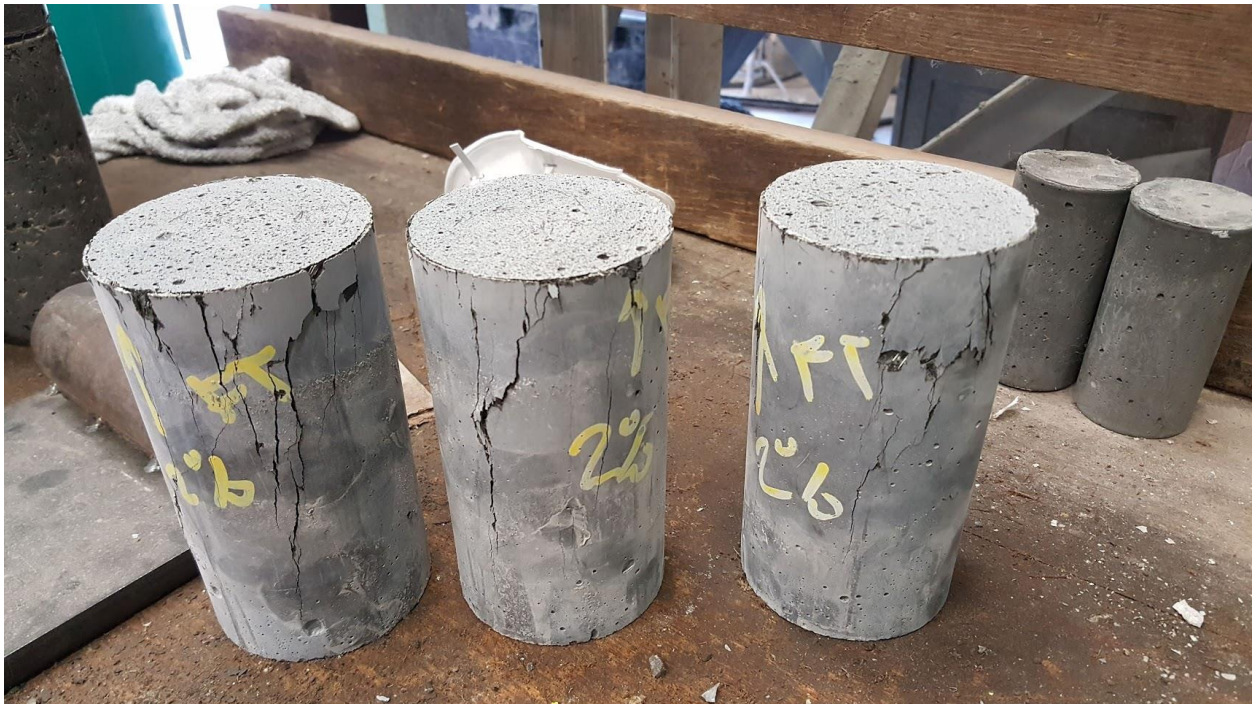
Figure 66: Freeze-thaw 2% 28 day cylinder compressive strength test specimens after failure
