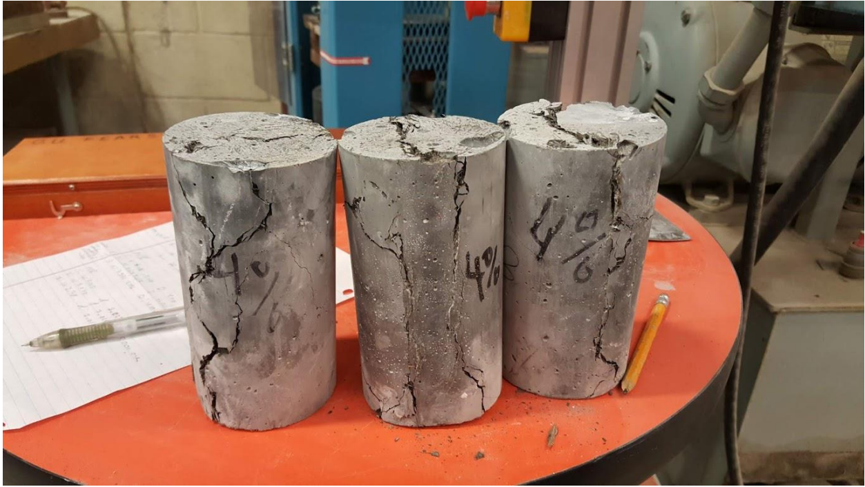
Figure 48: OU J3 4% 28 day splitting tensile test specimens after failure
