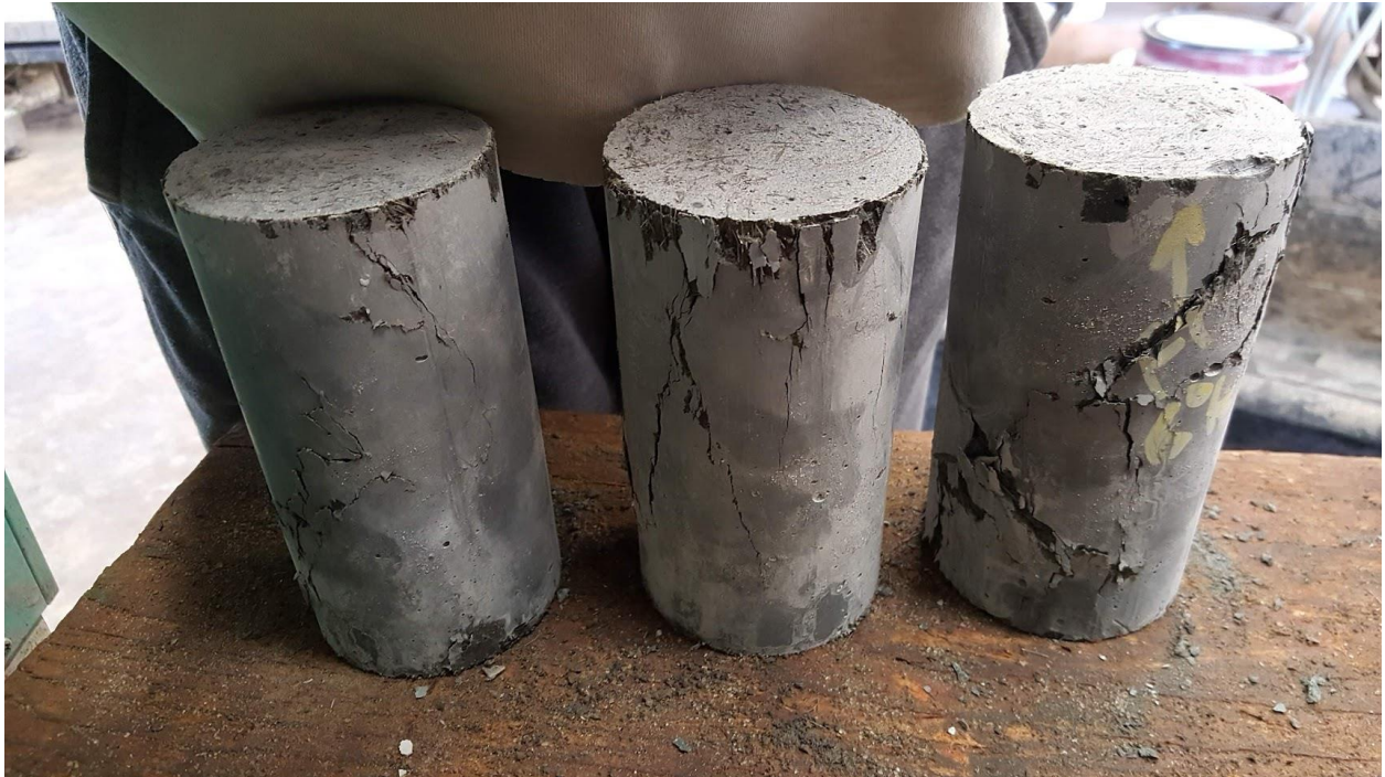
Figure 68: Freeze-thaw 6% 28 day cylinder compressive strength test specimens after failure
