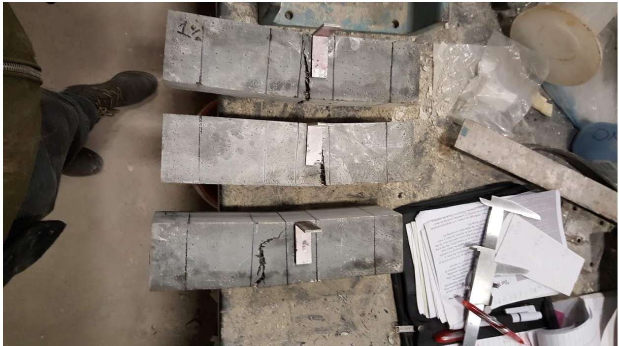
Figure 106: FIU J3 1% 56 day MOR test specimens after failure
