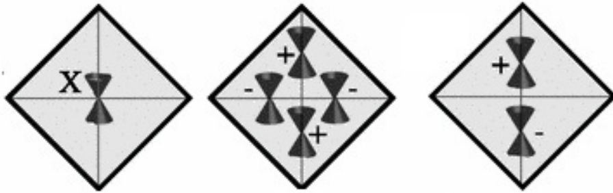
Figure 2.11: Schematic picture of Weyl semimetal (WSM) and Dirac semimetal (DSM). When \mathcal{T} and \mathcal{P} symmetry are both present, Dirac cone don't carry chiral charge (left). If \mathcal{P} symmetry is broken, two Weyl points on the opposite site has the same chiral charge (center). On the other hands, \mathcal{T} broken WSM has opposite chiral charge (right). The chiral charge of each Weyl point is illustrated by \pm sign [88].
