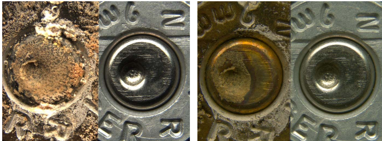
Picture 26: Unknown aluminum sample #16 before (left) and after cleaning with Randich method (right) after 6 months in water environment
