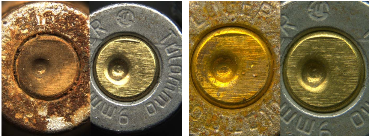
Picture 23: Unknown steel sample #1 before (left) and after cleaning with Randich method (right) after 3 months in water environment
