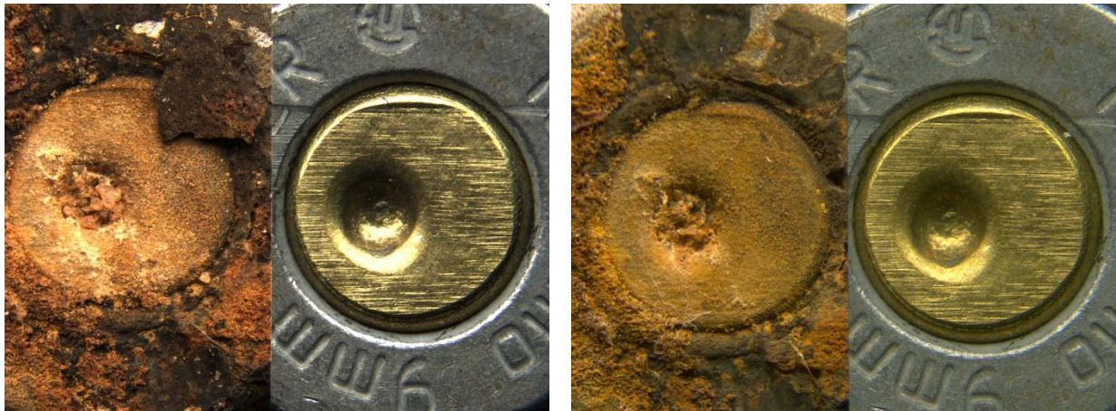
Picture 20: Unknown steel sample #1 before (left) and after cleaning with jewelry cleaner (right) after 6 months in water environment
