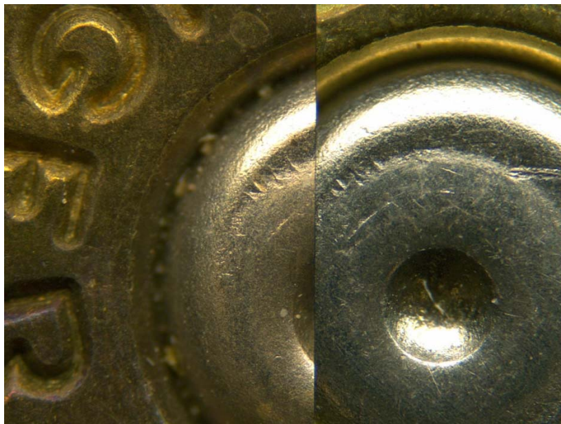
Picture 78: Unknown aluminum sample #7 from shaded exposed environment after 9 months (left) compared to known aluminum sample fired in Beretta model 92FS (right)
