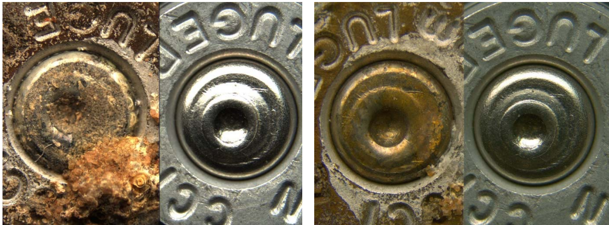
Picture 28: Unknown aluminum sample #14 before (left) and after cleaning with Randich method (right) after 9 months in water environment
