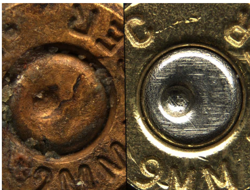
Picture 134: Unknown brass sample #10 from pig buried environment after 12 months (left) compared to known brass sample fired in Hi Point model C9 (right)
