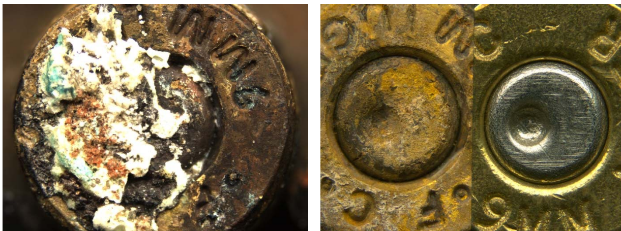
Picture 41: Unknown brass sample #6 before (left) and after cleaning with Randich method (right) after 6 months in pig buried environment
