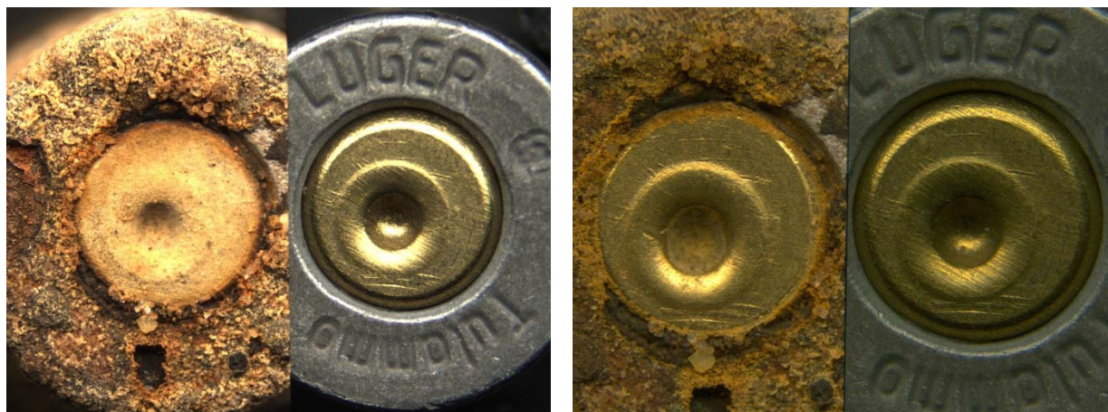
Picture 29: Unknown steel sample #6 before (left) and after cleaning with Aqua Regia (right) after 3 months in water environment
