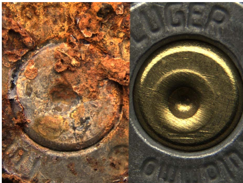
Picture 58: Unknown steel sample #15 from open buried environment after 6 months (left) compared to known steel sample fired in Beretta model 92FS (right)
