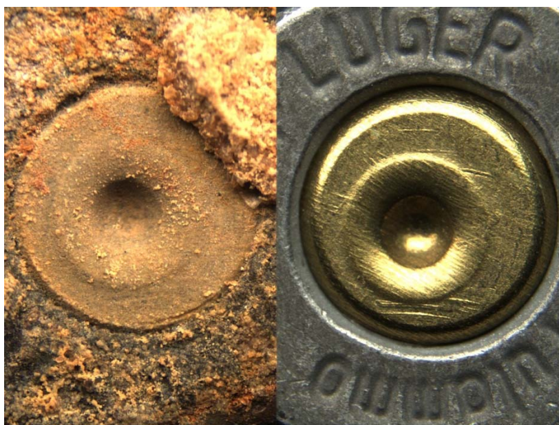
Picture 100: Unknown steel sample #15 from water environment after 9 months (left) compared to known steel sample fired in Beretta model 92FS (right)
