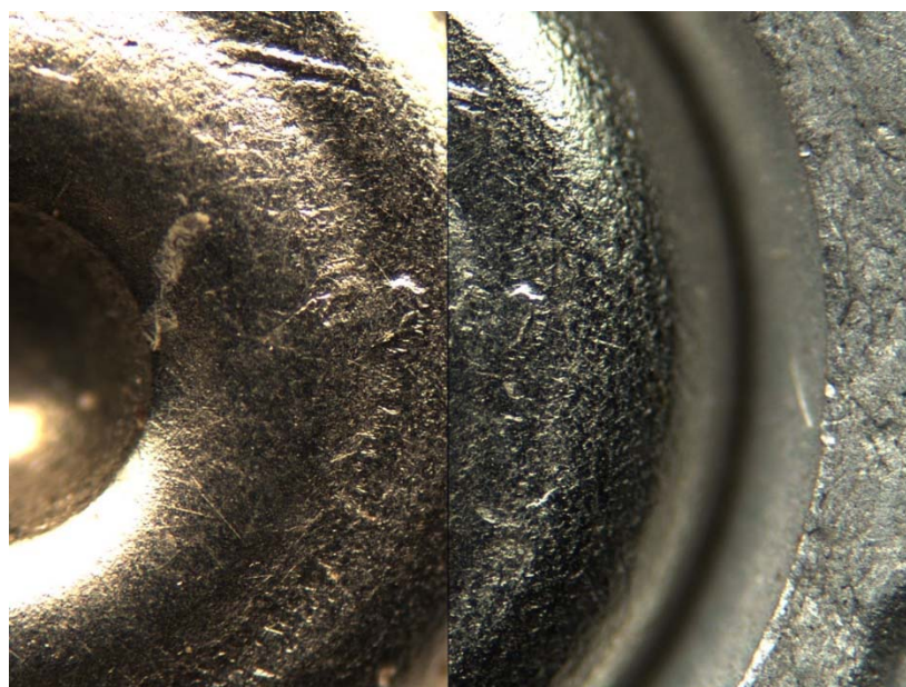
Picture 42: Unknown aluminum sample #17 from shaded exposed environment after 6 months (left) compared to known brass sample fired in Beretta model 92FS (right)
