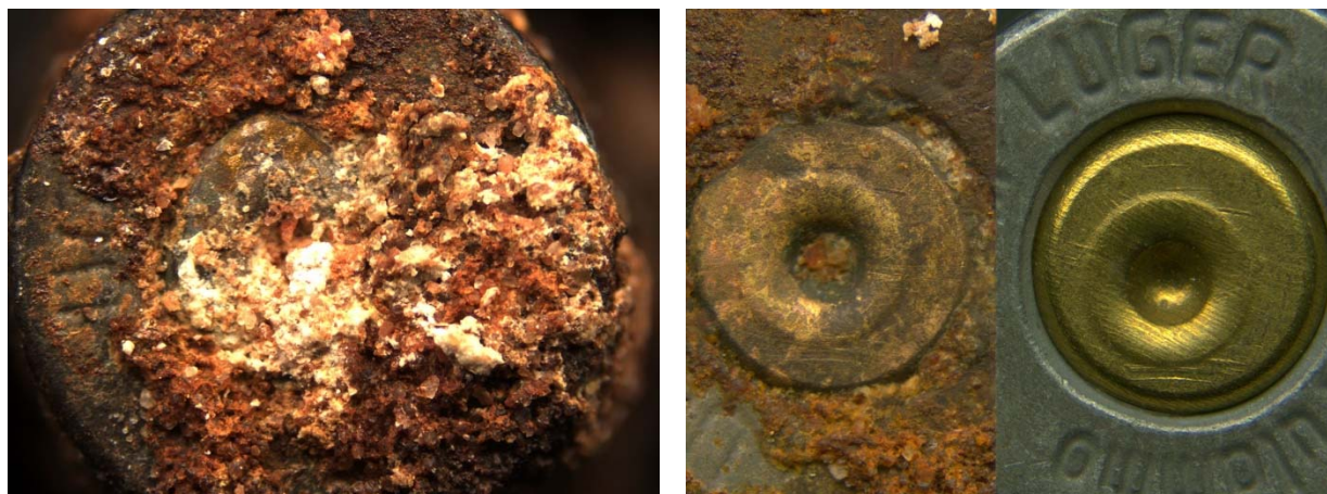
Picture 47: Unknown steel sample #8 before (left) and after cleaning with Aqua Regia (right) after 9 months in pig buried environment
