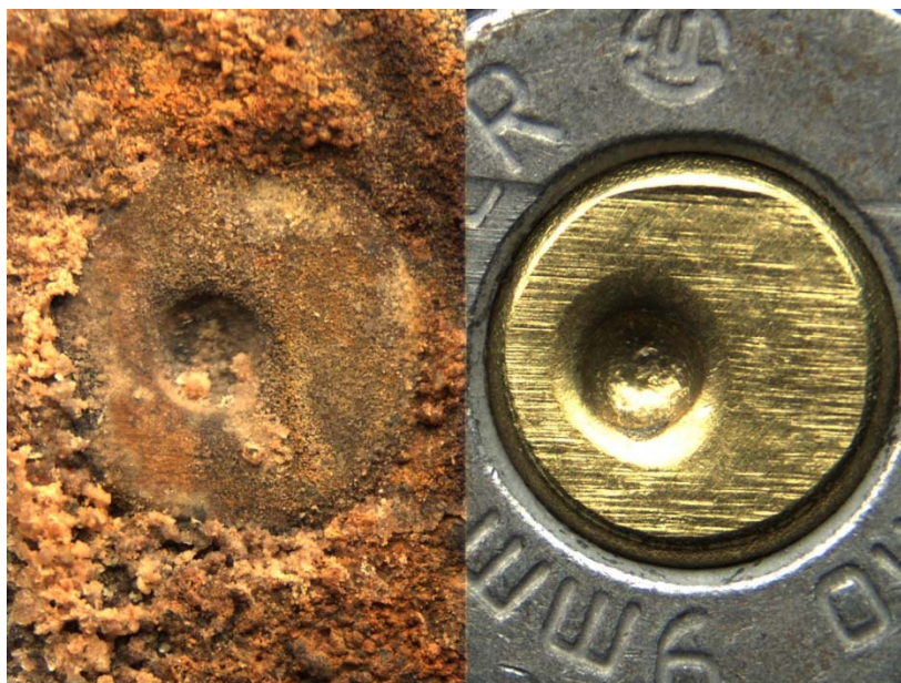
Picture 98: Unknown brass sample #2 from water environment after 9 months (left) compared to known brass sample fired in Hi Point model C9 (right)
