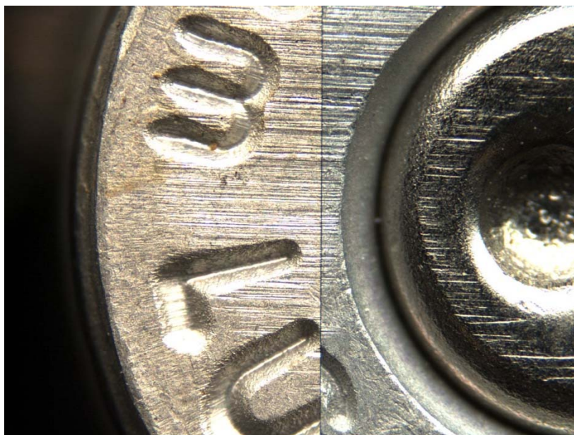
Picture 4: Unknown steel sample #7 from shaded exposed environment after 3 months (left) compared to known steel sample fired in Beretta model 92FS (right)
