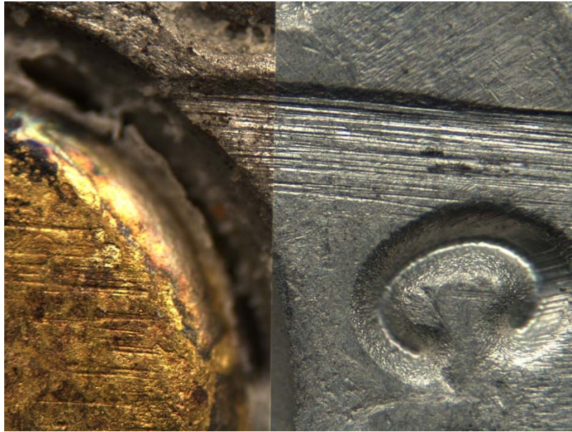
Picture 106: Unknown steel sample #18 from pig buried environment after 9 months (left) compared to known steel sample fired in Beretta model 92FS (right)
