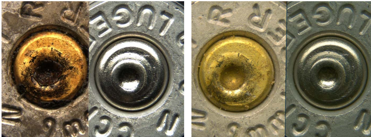
Picture 40: Unknown aluminum sample #4 before (left) and after cleaning with Randich method (right) after 6 months in pig buried environment
