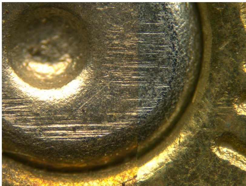
Picture 74: Unknown brass sample #17 from shaded exposed environment after 9 months (left) compare to known brass sample fired in Hi Point model C9 (right)
