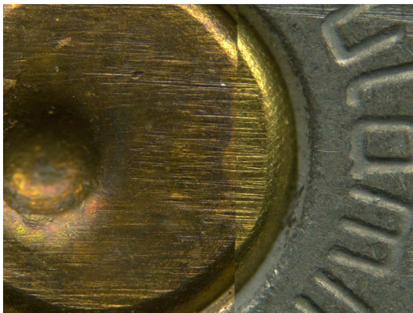
Picture 110: Unknown brass sample #11 from shaded exposed environment after 12 months (left) compared to known brass sample fired in Hi Point model C9 (right)
