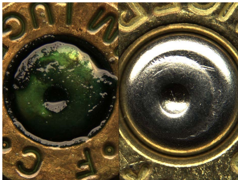
Picture 108: Unknown aluminum sample #2 from pig buried environment after 9 months (left) compared to known aluminum sample fired in Beretta model 92FS (right)
