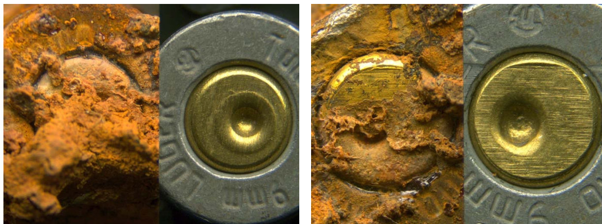
Picture 13: Unknown steel sample #7 before (left) and after cleaning with jewelry cleaner (right) after 9 months in open buried environment
