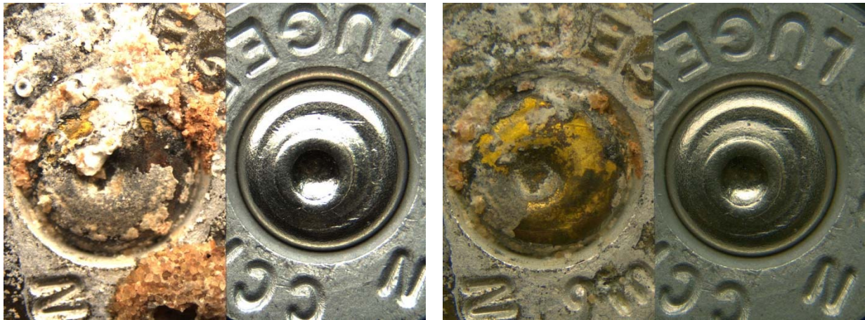
Picture 21: Unknown aluminum sample #11 before (left) and after cleaning with jewelry cleaner (right) after 9 months in water environment
