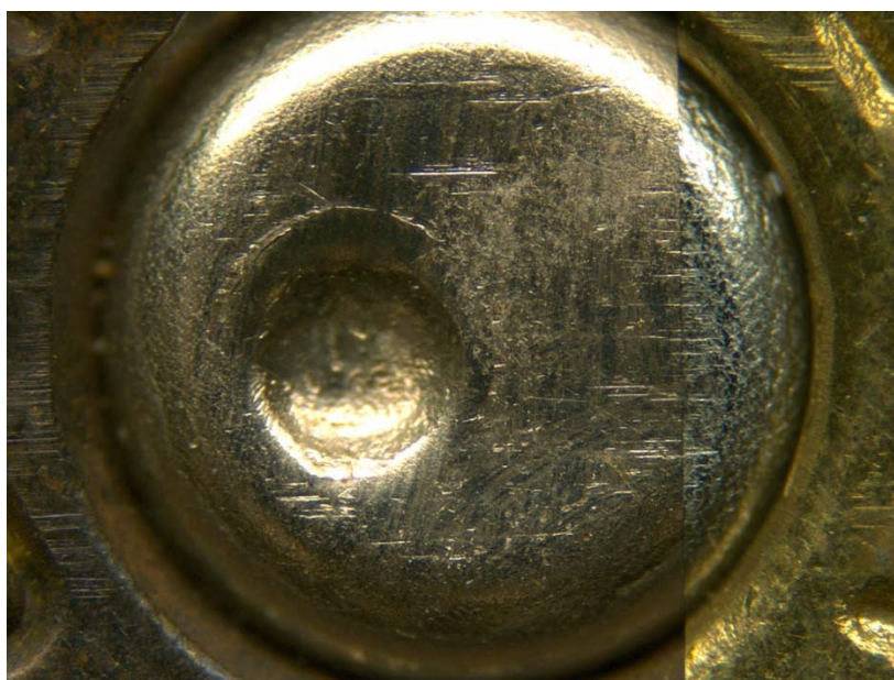
Picture 50: Unknown brass sample #16 from open exposed environment after 6 months (left) compared to known brass sample fired in Hi Point model C9 (right)
