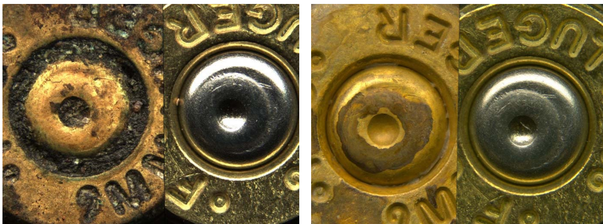
Picture 39: Unknown brass sample #13 before (left) and after cleaning with Randich method (right) after 3 months in pig buried environment
