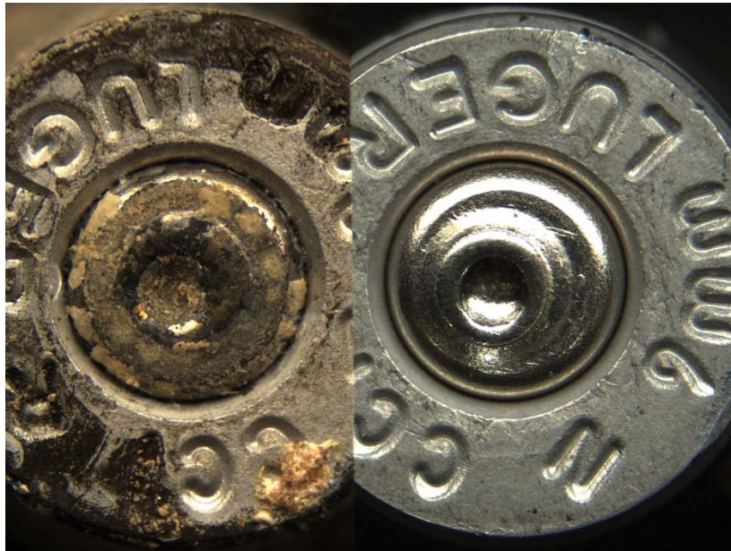
Picture 30: Unknown aluminum sample #2 from water environment after 3 months (left) compared to known aluminum sample fired in Beretta model 92FS (right)
