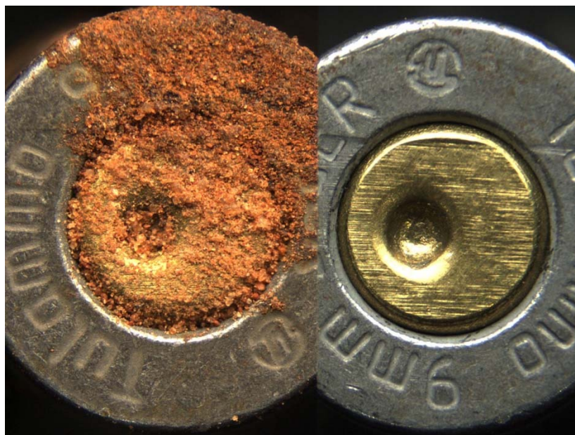
Picture 14: Unknown brass sample #16 from open exposed environment after 3 months (left) compared to known brass sample fired in Hi Point model C9 (right)
