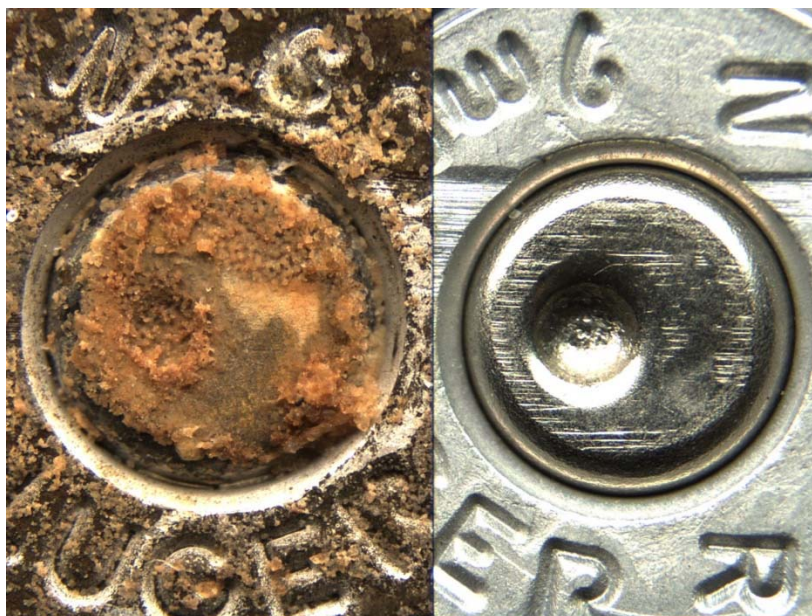
Picture 100: Unknown steel sample #15 from water environment after 9 months (left) compared to known steel sample fired in Beretta model 92FS (right)
