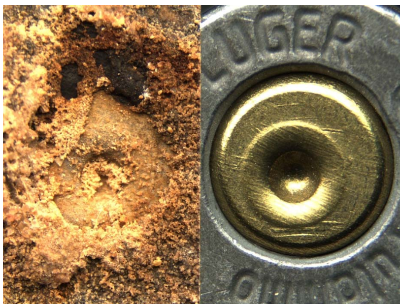
Picture 64: Unknown steel sample #5 from water environment after 6 months (left) compared to known steel sample fired in Beretta model 92FS (right)
