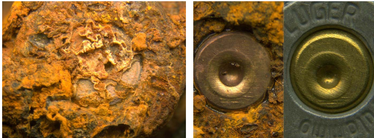
Picture 18: Unknown steel sample #1 before (left) and after cleaning with Aqua Regia (right) after 12 months in open buried environment
