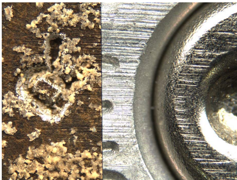
Picture 28: Unknown steel sample #18 from water environment after 3 months (left) compared to known steel sample fired in Beretta model 92FS (right)
