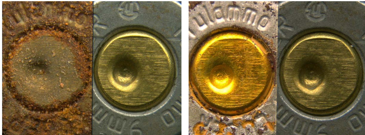
Picture 10: Unknown steel sample #17 before (left) and after cleaning Randich method (right) after 12 months in open exposed environment
