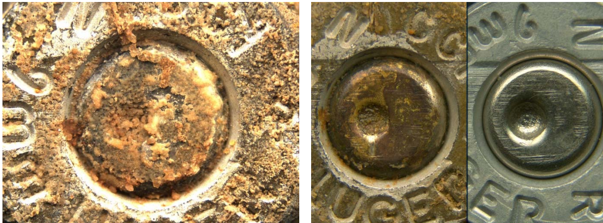
Picture 32: Unknown aluminum sample #4 before (left) and after cleaning with Aqua Regia (right) after 9 months in water environment
