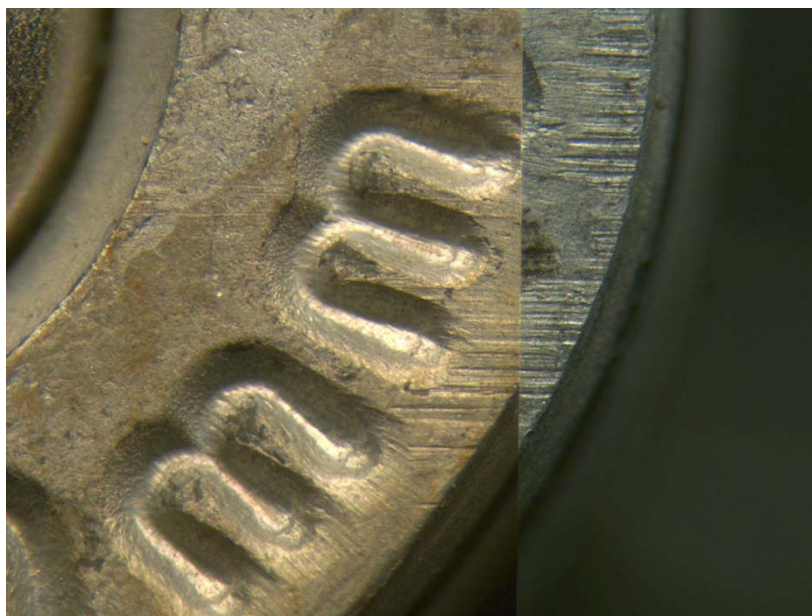
Picture 124: Unknown steel sample #9 from open exposed environment after 12 months (left) compared to known steel sample fired in Beretta model 92FS (right)
