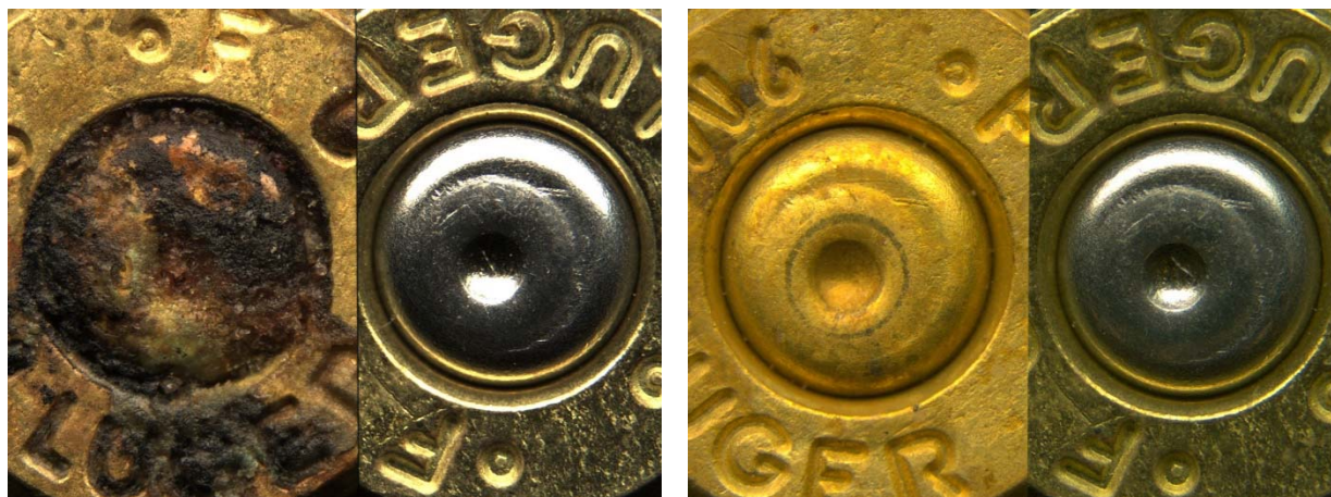
Picture 45: Unknown brass sample #7 before (left) and after cleaning with Randich method (right) after 12 months in pig buried environment
