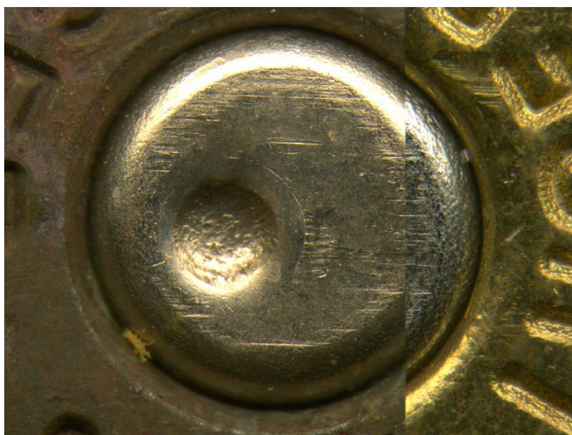
Picture 128: Unknown brass sample #12 from open buried environment after 12 months (left) compared to known brass sample fired in Hi Point model C9 (right)
