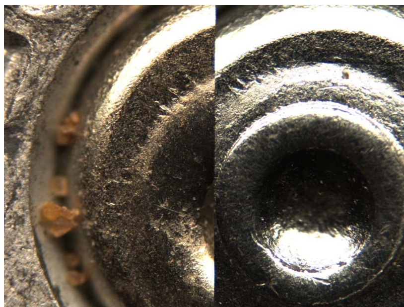
Picture 48: Unknown aluminum sample #9 from shaded buried environment after 6 months (left) compared to known aluminum sample fired in Beretta model 92FS (right)
