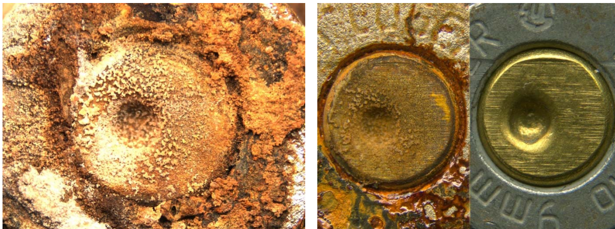
Picture 27: Unknown steel sample #7 before (left) and after cleaning with Randich method (right) after 9 months in water environment
