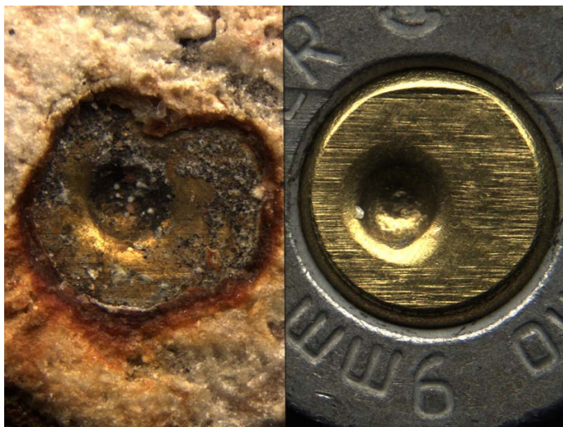
Picture 134: Unknown brass sample #10 from pig buried environment after 12 months (left) compared to known brass sample fired in Hi Point model C9 (right)
