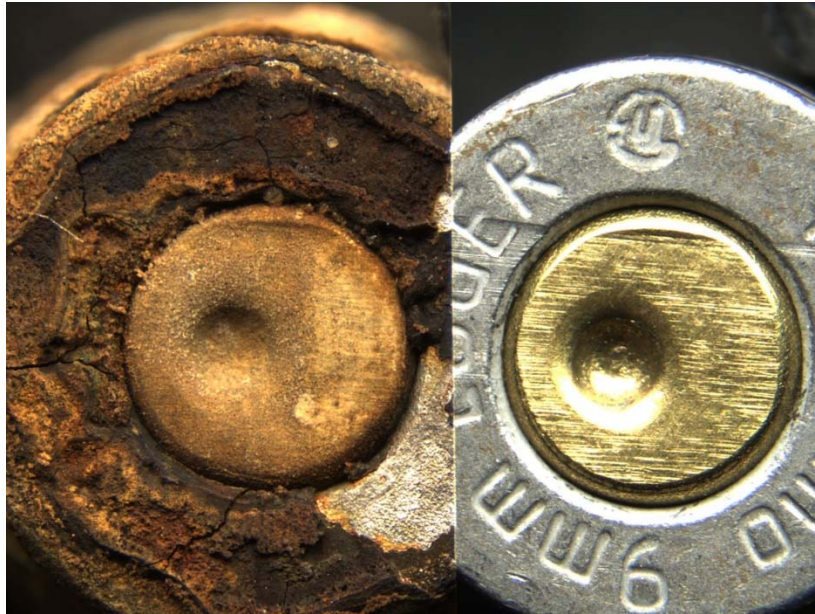
Picture 26: Unknown brass sample #5 from water environment after 3 months (left) compared to known brass sample fired in Hi Point model C9 (right)
