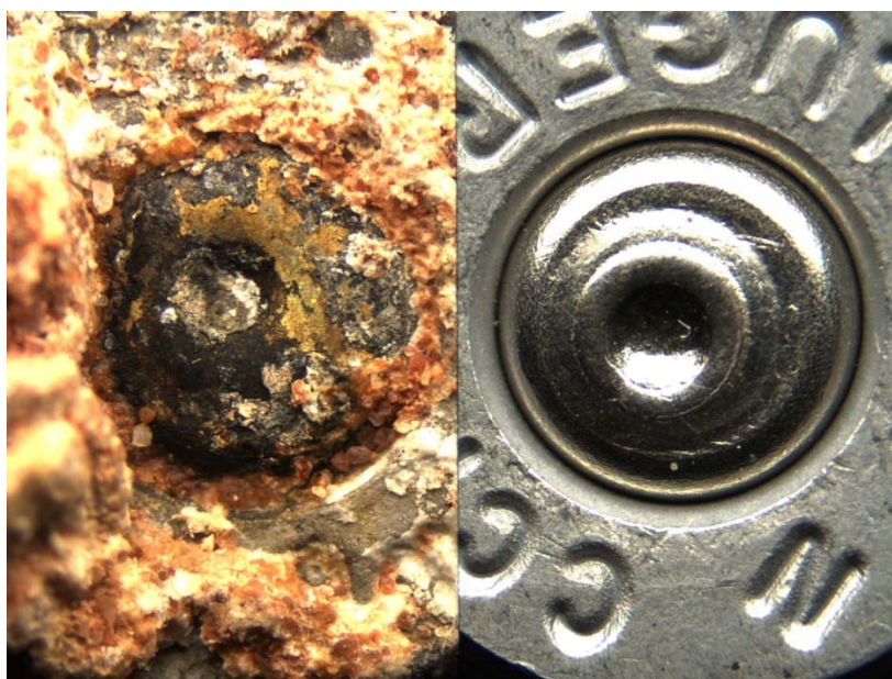
Picture 138: Unknown aluminum sample #8 from pig buried environment after 12 months (left) compared to known aluminum sample fired in Beretta model 92FS (right)
