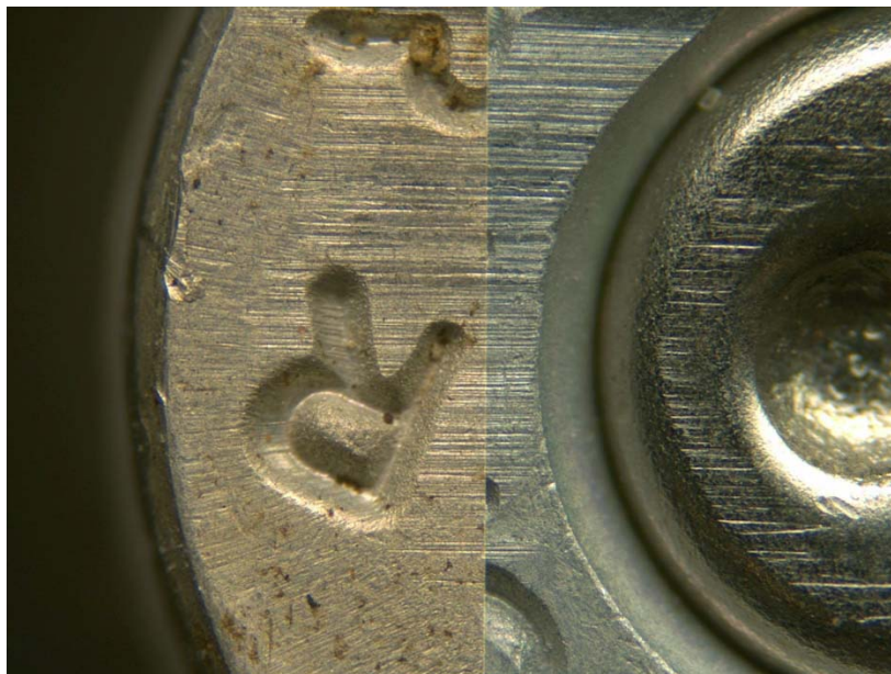
Picture 76: Unknown steel sample #10 from shaded exposed environment after 9 months (left) compared to known aluminum sample fired in Beretta model 92FS (right)
