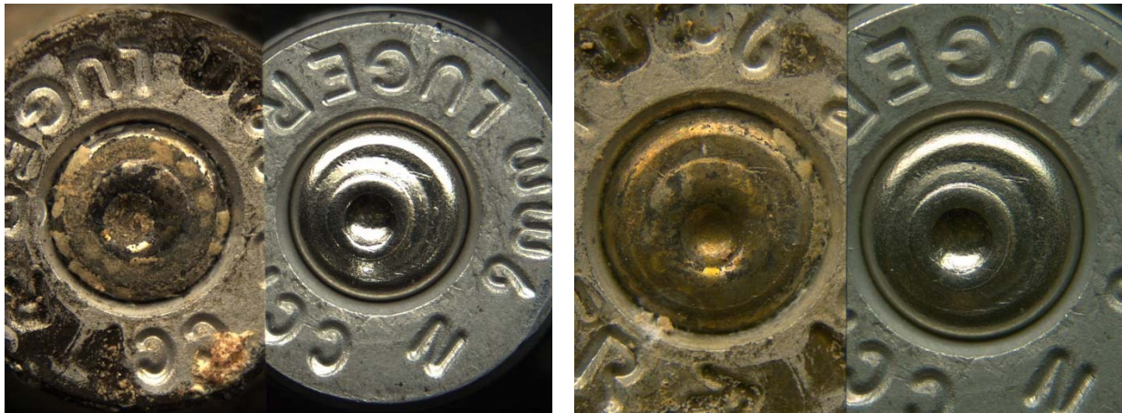
Picture 24: Unknown aluminum sample #2 before (left) and after cleaning with Randich method (right) after 3 months in water environment
