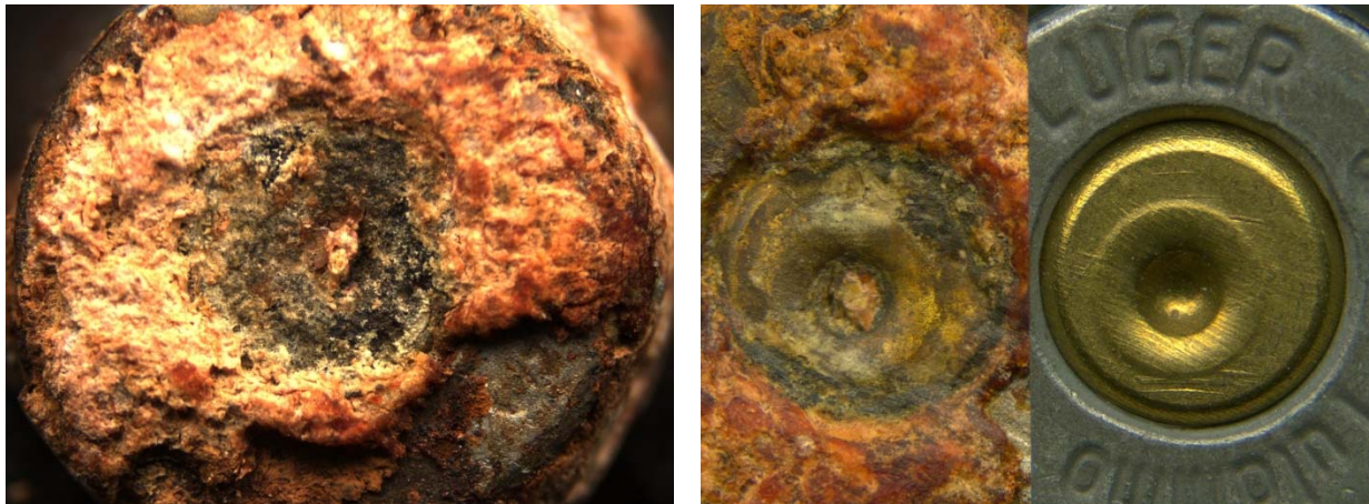
Picture 36: Unknown steel sample #4 before (left) and after cleaning with jewelry cleaner (right) after 9 months in pig buried environment
