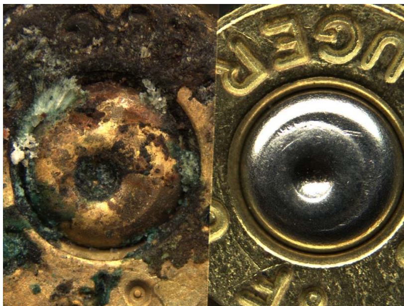
Picture 72: Unknown aluminum sample #1 from pig buried environment after 6 months (left) compared to known aluminum sample fired in Beretta model 92FS (right)
