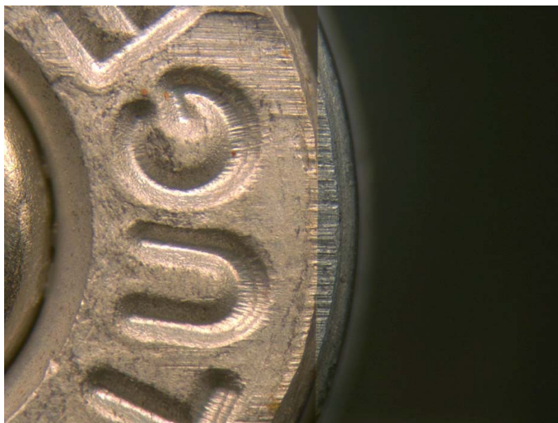
Picture 118: Unknown steel sample #5 from shaded buried environment after 12 months (left) compared to known steel sample fired in Beretta model 92FS (right)
