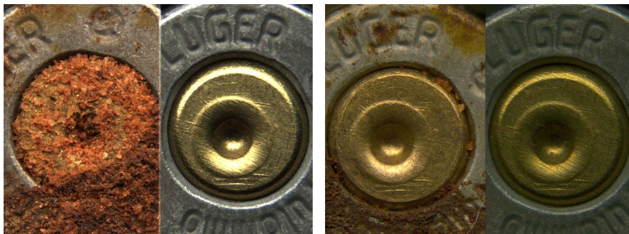
Picture 11: Unknown steel sample #11 before (left) and after cleaning with Aqua Regia (right) after 6 months in open exposed environment
