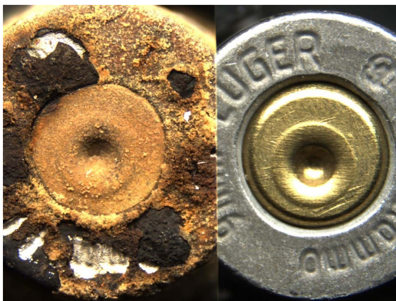
Picture 28: Unknown steel sample #18 from water environment after 3 months (left) compared to known steel sample fired in Beretta model 92FS (right)
