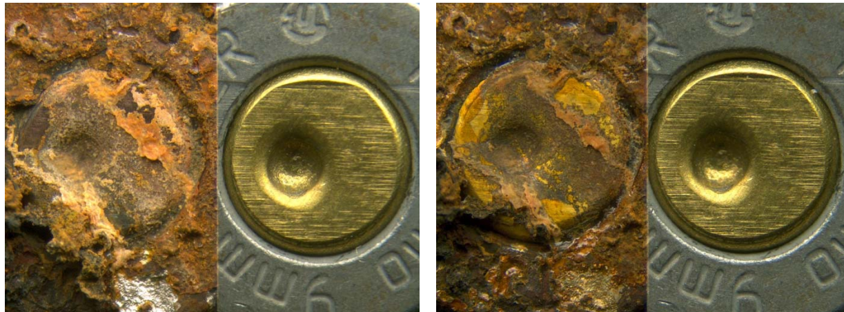
Picture 16: Unknown steel sample #7 before (left) and after cleaning with Randich method (right) after 12 months in open buried environment
