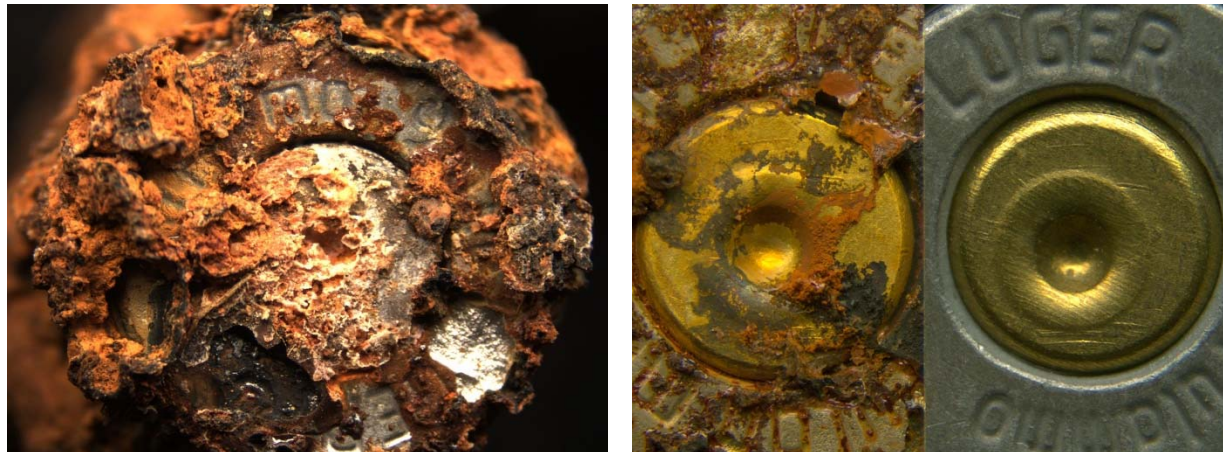
Picture 14: Unknown steel sample #3 before (left) and after cleaning with Randich method (right) after 6 months in open buried environment
