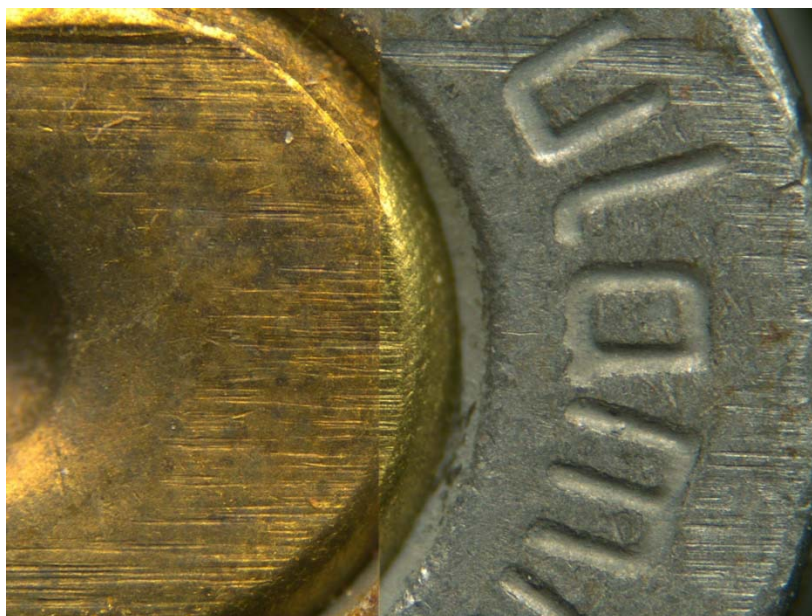
Picture 92: Unknown brass sample #2 from open buried environment after 9 months (left) compared to known brass sample fired in Hi Point model C9 (right)
