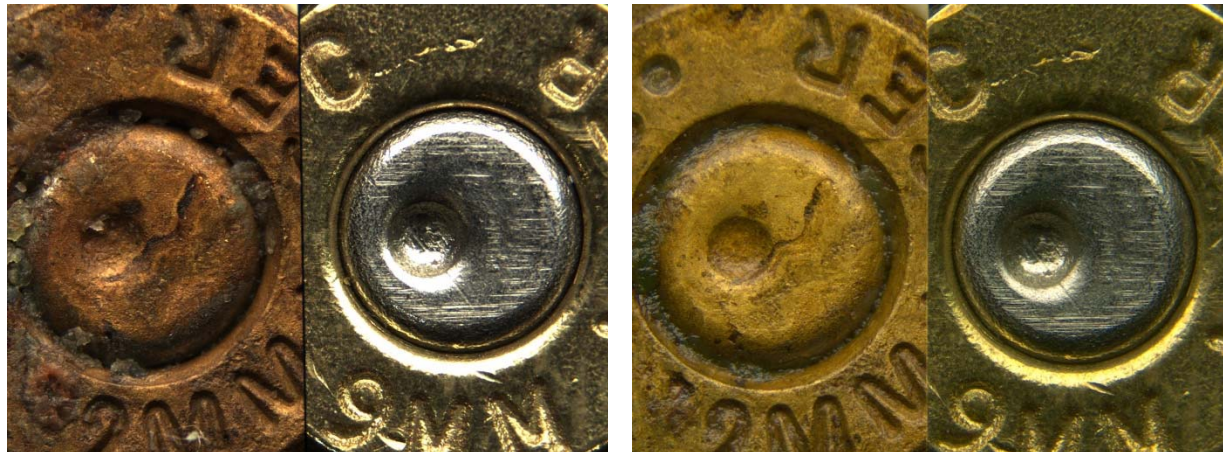
Picture 50: Unknown brass sample #10 before (left) and after cleaning with Aqua Regia (right) after 12 months in pig buried environment
