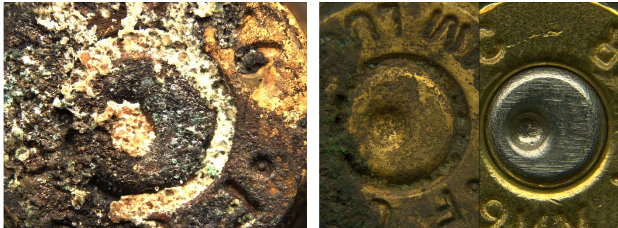
Picture 48: Unknown brass sample #1 before (left) and after cleaning with Aqua Regia (right) after 9 months in pig buried environment
