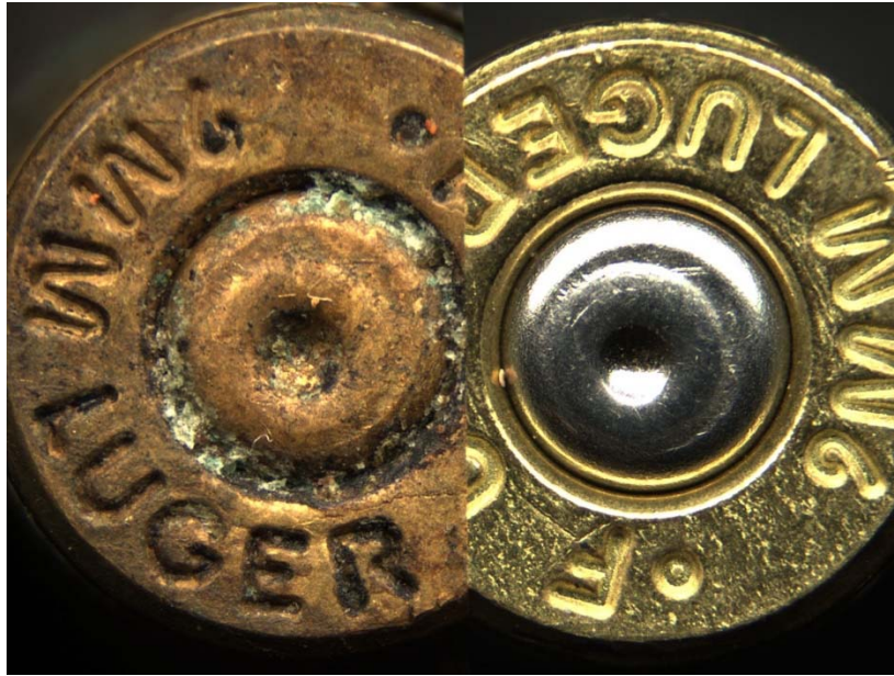
Picture 36: Unknown aluminum sample #3 from pig buried environment after 3 months (left) compared to known aluminum sample fired in Beretta model 92FS (right)
