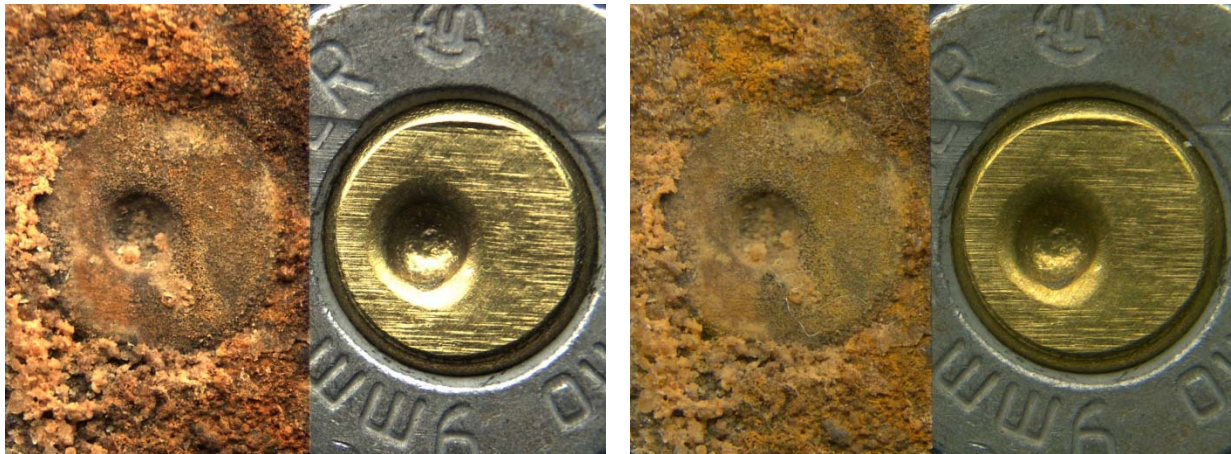
Picture 22: Unknown steel sample #10 before (left) and after cleaning with jewelry cleaner (right) after 9 months in water environment
