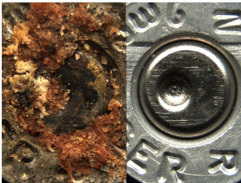
Picture 136: Unknown steel sample #13 from pig buried environment after 12 months (left) compared to known steel sample fired in Beretta model 92FS (right)
