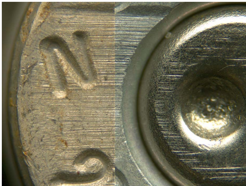
Picture 82: Unknown steel sample #1 from shaded buried environment after 9 months (left) compared to known steel sample fired in Beretta model 92FS (right)
