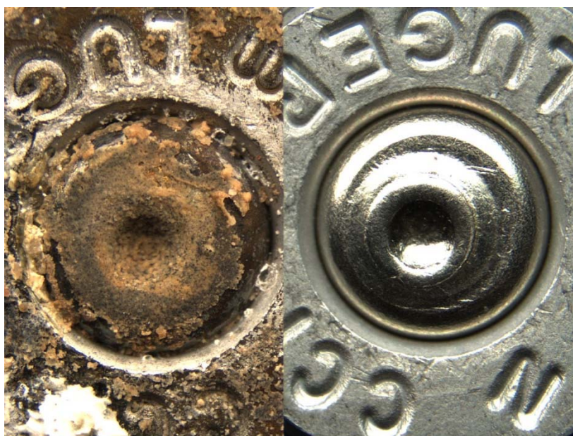
Picture 102: Unknown aluminum sample #16 from water environment after 9 months (left) compared to known aluminum sample fired in Beretta model 92FS (right)
