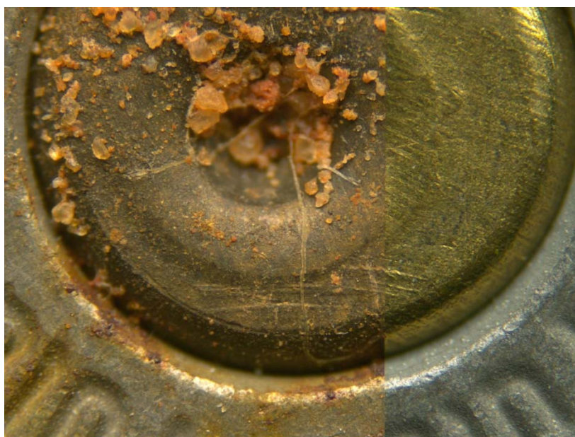
Picture 88: Unknown steel sample #14 from open exposed environment after 9 months (left) compared to known steel sample fired in Beretta model 92FS (right)
