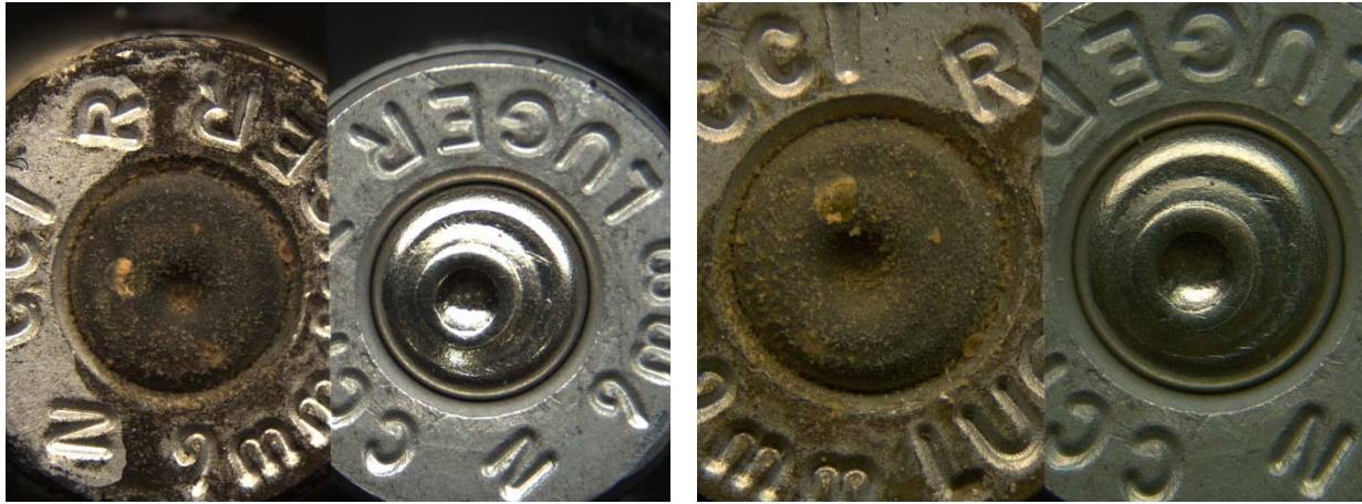
Picture 19: Unknown aluminum sample #4 before (left) and after cleaning with jewelry cleaner (right) after 3 months in water environment
