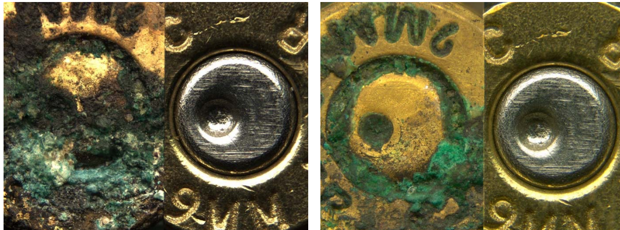
Picture 46: Unknown brass sample #14 before (left) and after cleaning with Aqua Regia (right) after 6 months in pig buried environment
