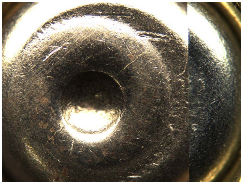
Picture 24: Unknown aluminum sample #11 from open buried environment after 3 months (left) compared to known aluminum sample fired in Beretta model 92FS (right)
