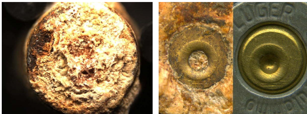
Picture 49: Unknown steel sample #4 before (left) and after cleaning with Aqua Regia (right) after 12 months in pig buried environment
