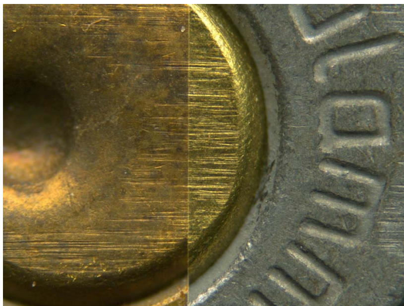
Picture 86: Unknown brass sample #6 from open exposed environment after 9 months (left) compared to known brass sample fired in Hi Point model C9 (right)
