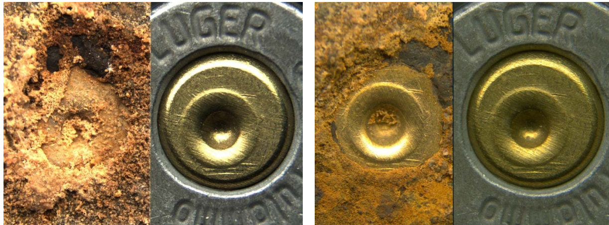
Picture 30: Unknown steel sample #5 before (left) and after cleaning with Aqua Regia (right) after 6 months in water environment
