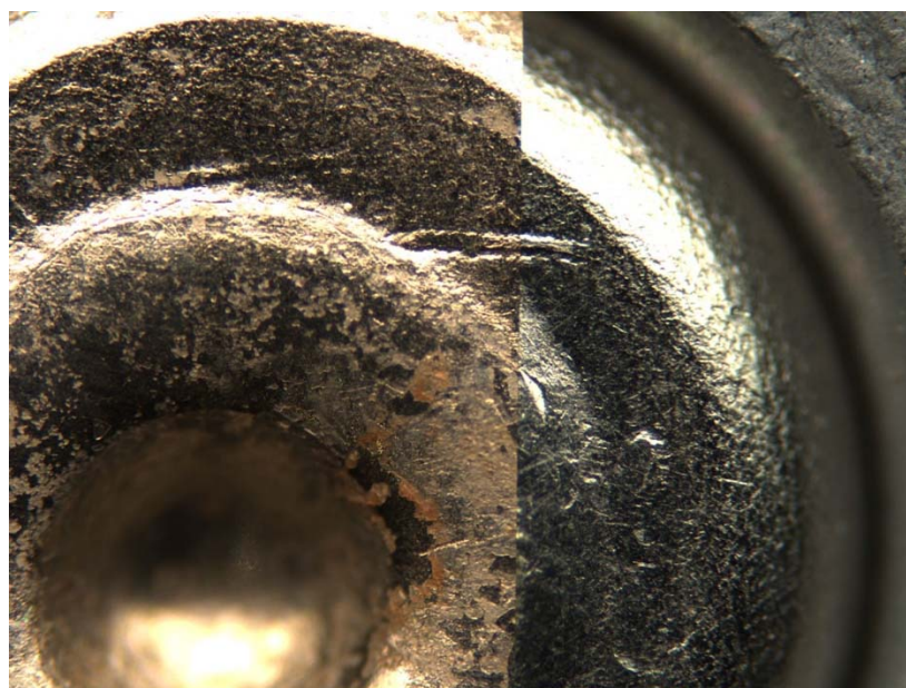
Picture 60: Unknown aluminum sample #17 from open buried environment after 6 months (left) compared to known aluminum sample fired in Beretta model 92FS (right)
