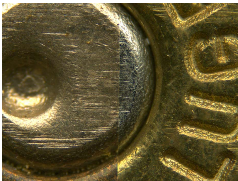
Picture 110: Unknown brass sample #11 from shaded exposed environment after 12 months (left) compared to known brass sample fired in Hi Point model C9 (right)
