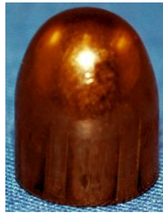
Figure 2. LEAs and GEAs on a fired bullet.
