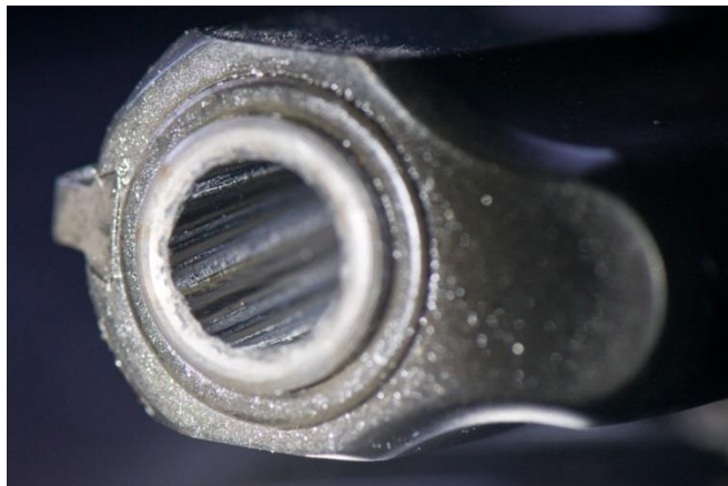
Figure 1. Rifling inside of a pistol barrel. [Photograph], by ArtBrom, 2011, Retrieved from https://www.flickr.com/photos/art-sarah/5554842728
