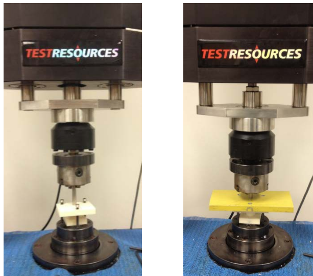
Figure 4.2 (a) Static tests setup in UTM before curing; (b) during curing
