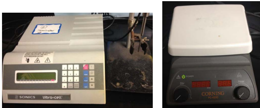
Figure 5.2 (a) Sonic vitro & sonication device used for sonication; (b) Corning heating & magnetic stirring cell
