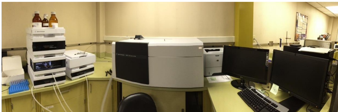
Figure 10. Agilent LC/MS/MS system used in study
