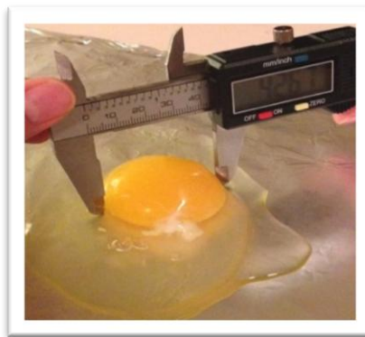
Figure 7 Measuring yolk width by a digital vernier caliper micrometer gauge
