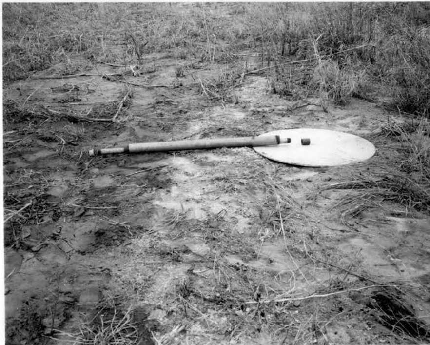
Figure 5. Basic elements of consolidation gages showing 24" plate, 1" union, 1" gage pipe and 2" protecting pipe
