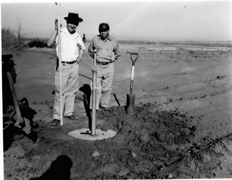
Figure 16. The complete gage with first joints of gage (1") pipe and protecting (2") pipe installed.
