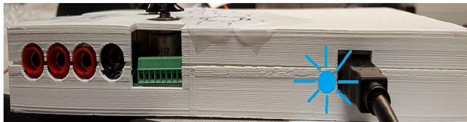
Figure 4-9: The Line Interface's power indicator LED.
