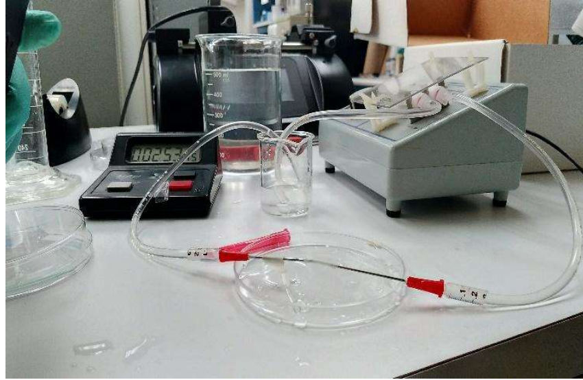
Figure 4-3: Flow test setup for a fabricated blood vessel
