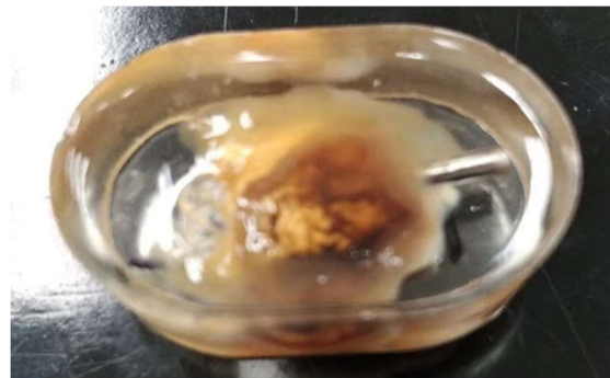
Figure 3-3: The implant is embedded in the Technovit-7200 VLC
