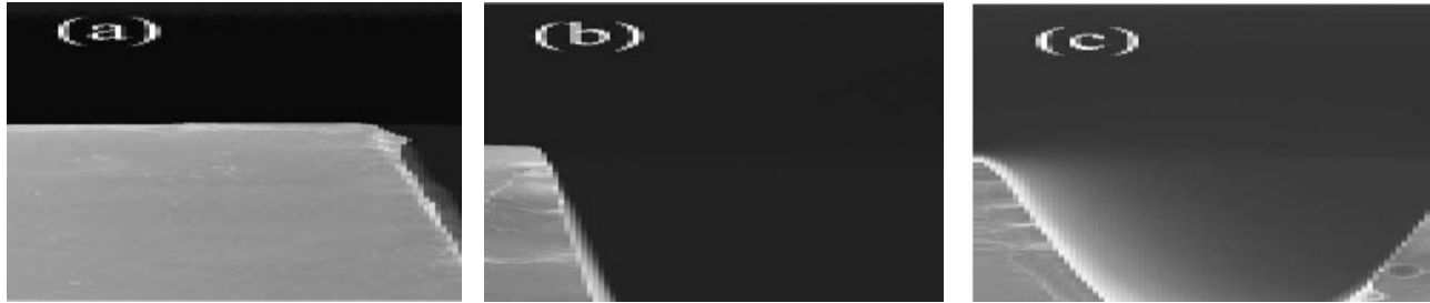
Figure 2.4: Rim bulging on machined PMMA. SEM images of machined PMMA. Adopted from Cheng et. al. [39]. a.) Cast PMMA without annealing. b.) Cast PMMA after annealing. c.) Extruded PMMA without annealing.
