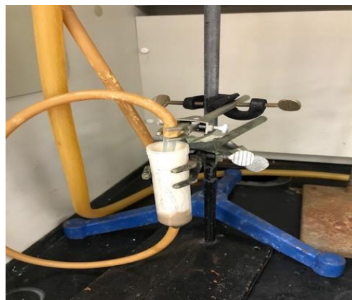
Figure 9: Passing nitrogen gas to dry sample
