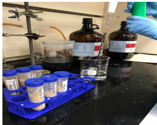
Figure 7: Adding solvent to mealworm powder by pipette
