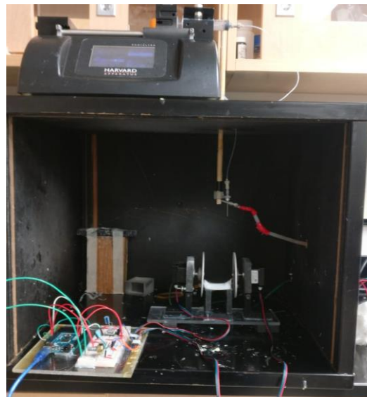
Figure 6: Dual disc setup to create electrospun nanofibers
