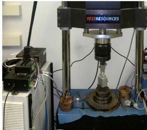
Figure 3-5: Three-point bend fixture for determining the bending properties of the bone cement.
