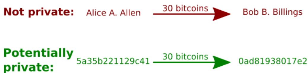
Figure 2. Explanation of Bitcoin’s pseudo-anonymous transaction structure. The example in red shows a traditional non-private transaction, while the example in green illustrates what information appears in Bitcoin’s blockchain. From “Excellent Privacy,” retrieved from https://bitcoin.org/en/bitcoin-core/features/privacy . Copyright 2015 by Bitcoin.org.
