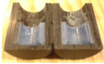
Figure 2-4 Measurement of the cement height by cutting cement holding cup into half using the band saw machine.
