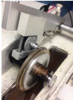
Figure 4-4. Micron depth grooving on the circumference of a Ti wire using Buehler diamond saw blade check and gripper. The gripper is holding a motor in which the shaft of the motor is secured with the implant.
