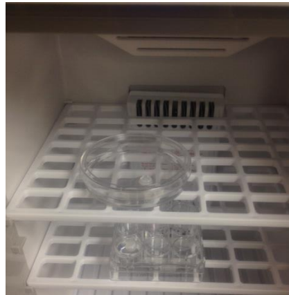
Figure 7-11 PEGDA IVD in PBS solution at 38 degree centigrade in an incubator.
