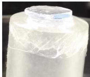
Figure 6-3 Fabricated 10 mm diameter and 1.5 mm thickness composite hydrogel on the mold.
