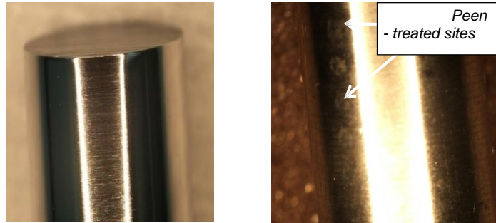
Figure 2-5 Laser-peened Ti samples. (left) Control and (right) peen-treated sample set
