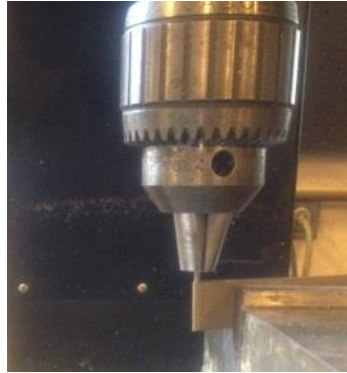
Figure 4-3. Polishing of Ti wire using a drill machine chuck and gripper
