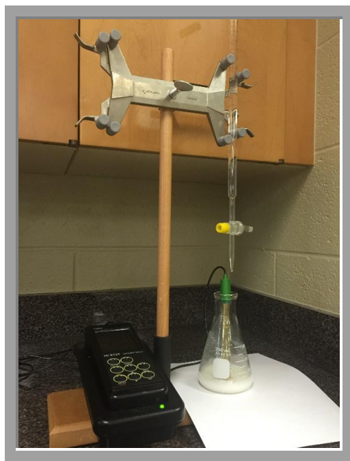
Figure 9. The titrateable acidity was measured triplicated by the standard titrateable method of AOAC (1990) with a pH/ORP Meter (HI 9125, HANNA instruments Co., Ltd)
